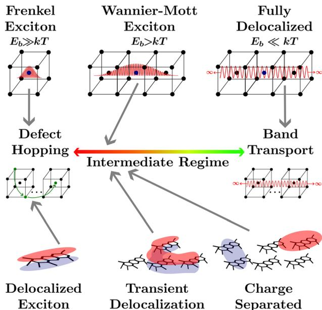
**Fig. 1** An illustration of the quasiparticle transport spectrum in solids. Top row—the difference between quasiparticle confinement in a body-centred cubic solid-state crystal. Middle row—the quasiparticle transport spectrum from inefficient defect hopping to efficient band transport. Bottom row—the excitonic structure of polymers and polymer films including excitons delocalized across a single polymer, transient delocalized excitons, and delocalized charge separated states.
