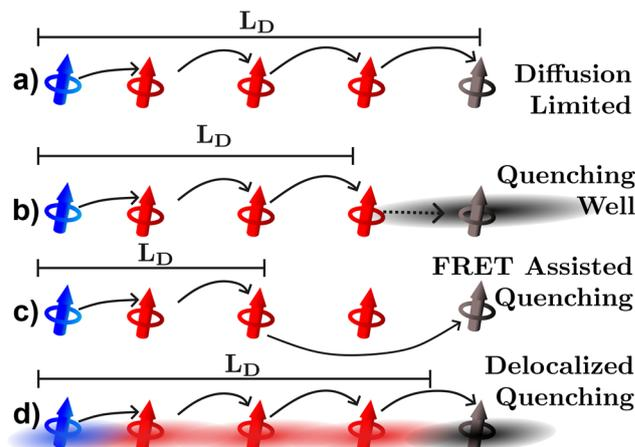
**Fig. 6** Pictorial representation of challenge (iii): quenching distances. Excitons generated on the blue dipole (polymer or molecule) diffuse through the red dipole and to the black quenching dipole. (a) The diffusion limited case as assumed by most quenching experiments. Underestimations can be caused by (b) quencher acting as a well pulling the excited exciton towards it, (c) FRET assisted quenching, or (d) delocalization assisted quenching.
