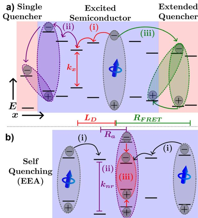
**Fig. 4** Excitonic processes in organic semiconductors. (a) Exciton created in the excited semiconductor can undergo diffusion until decay occurs (path i), electron transfer (path ii), or FRET transfer to a nearby quenching molecule, film, or phase (path iii), possibly followed by hole transfer. (b) Exciton–exciton annihilation processes, two excitons interact *via* FRET to produce a non-radiative decay and a thermalized exciton.
