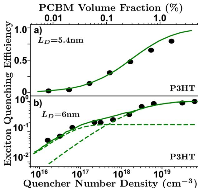
Fig. 7 Volume quenching experiments in P3HT-RR.<sup>84</sup> (a) Time-resolved photoluminescence experiments reveals a  $L_D$  of 5.4 nm.<sup>52</sup> (b) Anomalous quenching mechanism causing two quenching regimes revealing a  $L_D$  of 6 nm with a 17% anomalous yield.<sup>34</sup>
