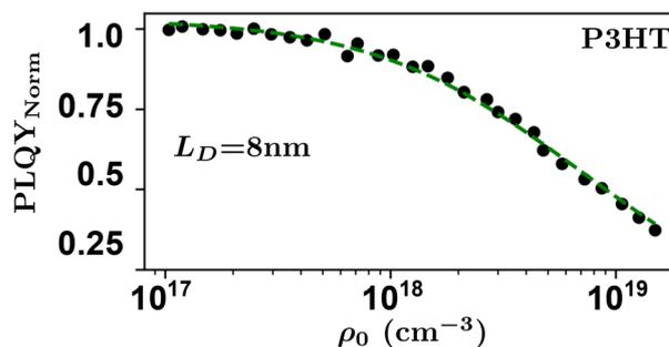
Fig. 9 Pulsed-PLQY on P3HT-RR.<sup>84</sup> A diffusion length of 8 nm was measured.<sup>48</sup>
