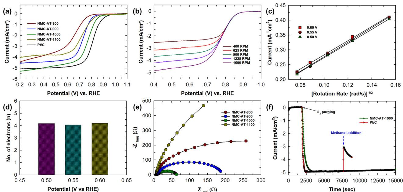
**Fig. 4** (a) LSV curves obtained at 10 mV s<sup>-1</sup> and 1600 RPM. (b) LSV curves obtained at 5 mV s<sup>-1</sup> and different speeds. (c) K–L plot derived from LSV curves. (d) Number of electrons calculated at different potentials. (e) EIS spectra of NMC-AT samples. (f) Methanol tolerance of the NMC-AT-1000 sample and Pt/C.
