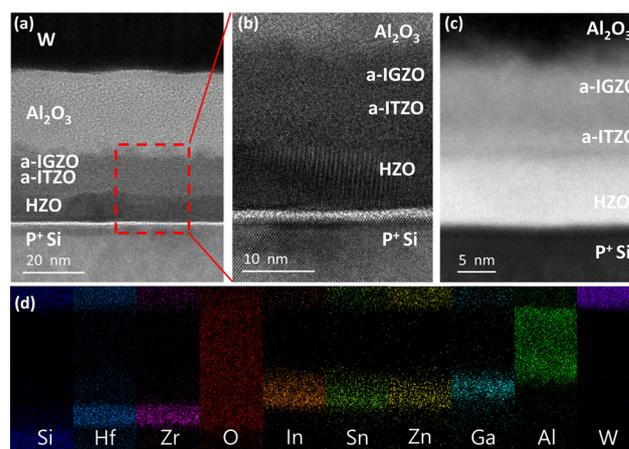
**Fig. 3** Cross-sectional (a) low-magnification and (b) high-magnification TEM, (c) STEM, (d) EDS image of fabricated FeFET. It shows a clear W/Al<sub>2</sub>O<sub>3</sub>/a-IGZO/a-ITZO/HZO/P<sup>+</sup> Si structure.
