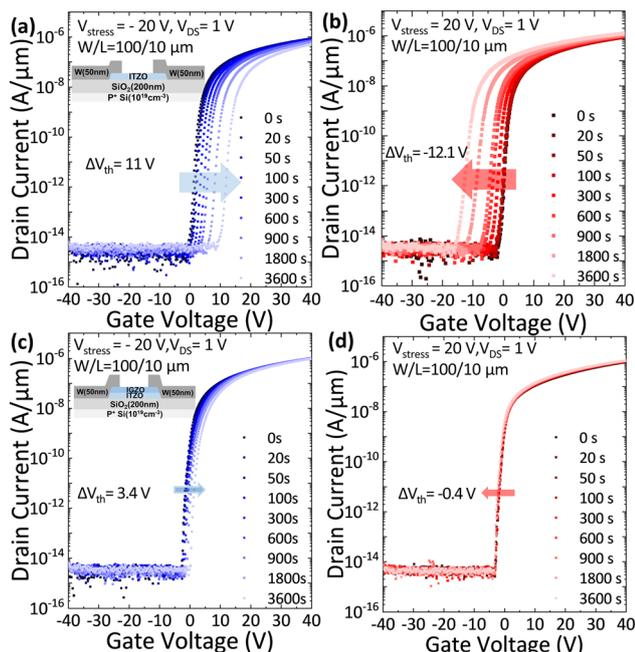
**Fig. 5** Transfer characteristics under (a) PBS and (b) NBS for a-ITZO single-layer FET, and (c) PBS and (d) NBS for a-ITZO/a-IGZO FET. Stress conditions:  $V_{stress} = \pm 20$  V for 3600 s,  $V_{DS} = 1$  V. Enhanced PBS/NBS stability achieved through reduced electron trapping at the channel/gate dielectric interface or oxygen molecule adsorption at the back-channel surface.
