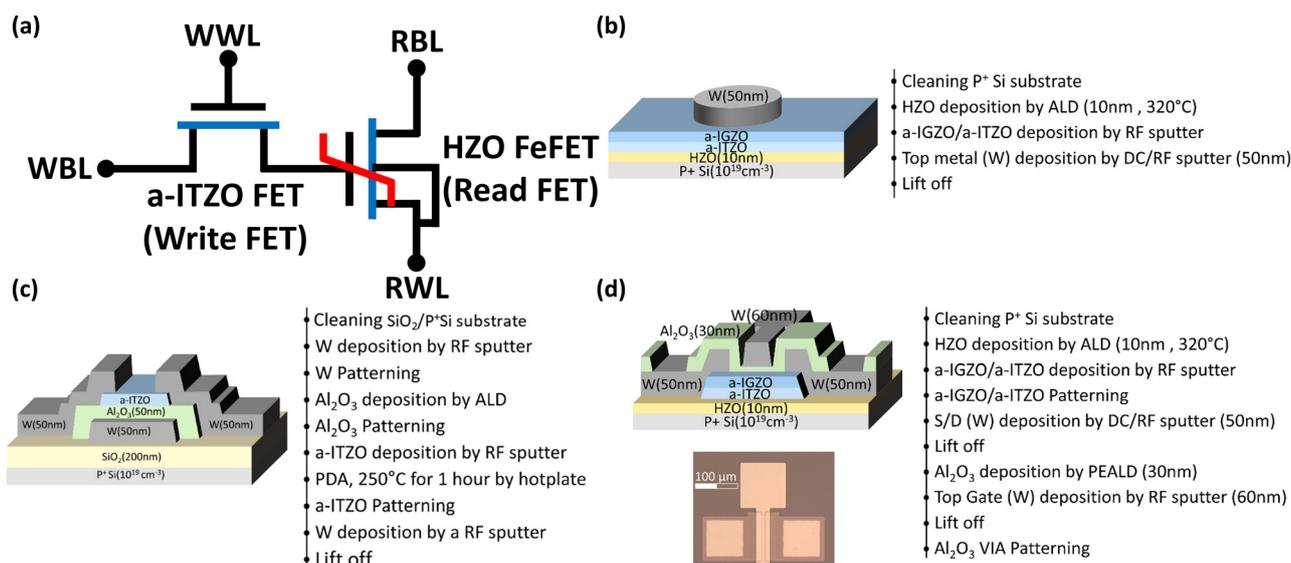
**Fig. 2** (a) Layout of the AOS-based 2T0C-FeDRAM cell with schematic device structure and fabrication process flow of (b) W/a-IGZO/a-ITZO/HZO/P<sup>+</sup> Si MSFM ferroelectric capacitors. (c) The a-ITZO FET as a W<sub>tr</sub>, and (d) the double gate W/Al<sub>2</sub>O<sub>3</sub>/a-IGZO/a-ITZO/HZO/P<sup>+</sup> Si MSFM ferroelectric capacitors.
