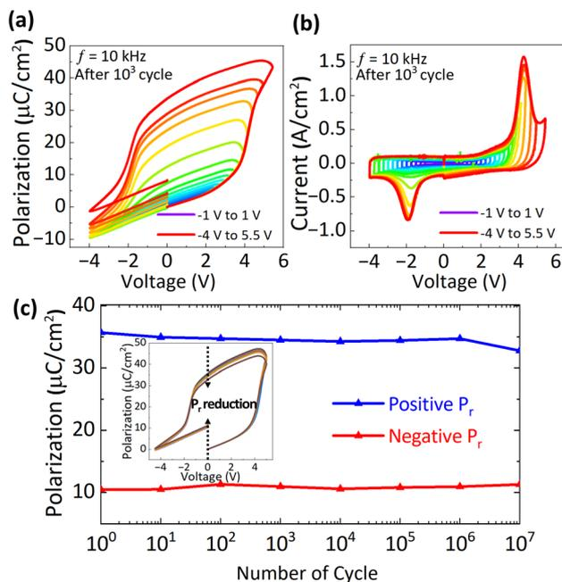
Fig. 4 (a) *P*–*V* and (b) *I*–*V* curves of W/a-IGZO/a-ITZO/HZO/P<sup>+</sup> Si MSFM capacitor. (c) Variation of the remanent polarization as a function of the number of cycles.
