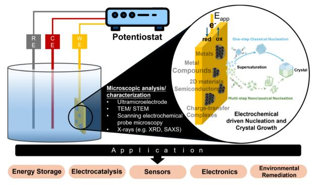
Fig. 1 Schematic representation of a typical three-electrode electrochemical cell setup for electrocrystallization, in situ analytical techniques for advancing the microscopic understanding of the electrocrystallization process, and the types of materials that can be electrochemically deposited.
