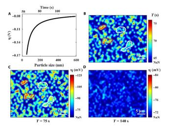
Fig. 9 Localized overpotential mapping by RIM. (A) Proof-of-concept curve fitting correlates  $\eta$  with the nucleus size. (B) The nuclei formation time map. (C) The overall  $\eta$  map at the deposition time of 75 s. (D) The overall  $\eta$  map at the deposition time of 140 s. "NaN" represents the region without nuclei. Reproduced from ref. 207 with permission. Copyright, 2021, under CC-BY license, published by Science Advances.
