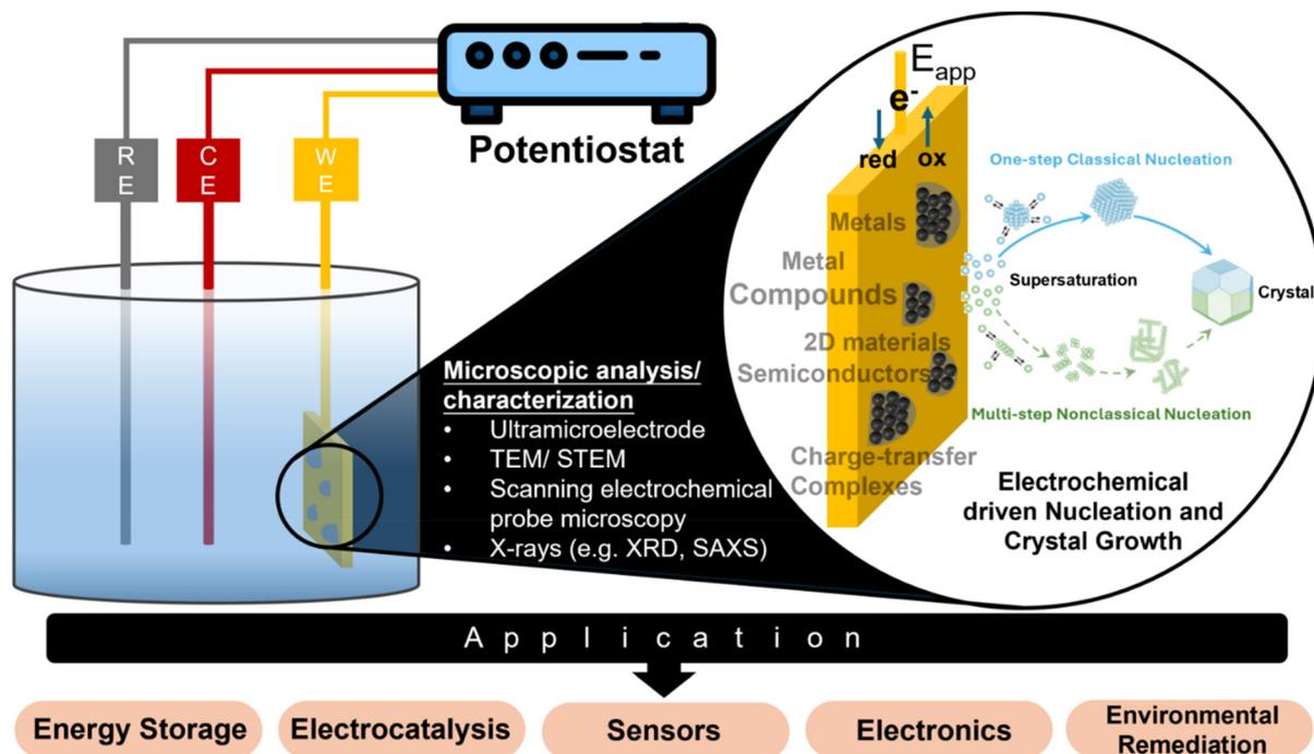
**Fig. 1** Schematic representation of a typical three-electrode electrochemical cell setup for electrocrystallization, *in situ* analytical techniques for advancing the microscopic understanding of the electrocrystallization process, and the types of materials that can be electrochemically deposited.
