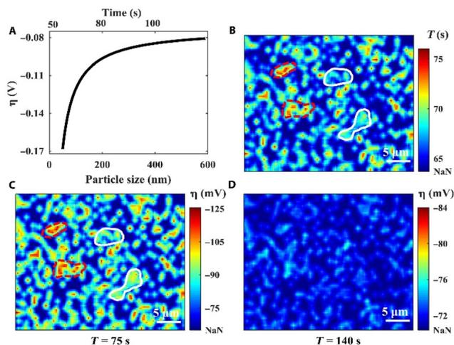
**Fig. 9** Localized overpotential mapping by RIM. (A) Proof-of-concept curve fitting correlates  $\eta$  with the nucleus size. (B) The nuclei formation time map. (C) The overall  $\eta$  map at the deposition time of 75 s. (D) The overall  $\eta$  map at the deposition time of 140 s. "NaN" represents the region without nuclei. Reproduced from ref. 207 with permission. Copyright, 2021, under CC-BY license, published by Science Advances.
