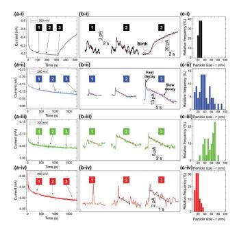
Fig. 12 (a) The current–time transients of TTF-Br electrodeposition at 300, 280, 270, and 250 mV, respectively, on the Au microdisk electrode in 0.1 mM TTF and 20 mM TBAB MeCN solution. (b) The magnified views from (a) showing individual current spikes represented by solid lines, alongside fits corresponding to zero-order kinetics represented by dashed lines. (c) The nanocluster size histograms at different applied potentials. Reproduced from ref. 24 with permission from John Wiley and Sons.
