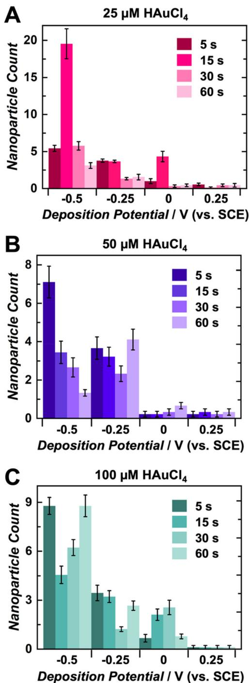
**Fig. 3** Gold nanoparticle (AuNP) count per individual electrode within the carbon ultramicroelectrode array (CUA) at various deposition times and potentials in solutions of (A) 25  $\mu\text{M}$ , (B) 50  $\mu\text{M}$ , and (C) 100  $\mu\text{M}$   $\text{HAuCl}_4$  in 0.5 M  $\text{H}_2\text{SO}_4$ , displayed in pink, purple, and green, respectively. Particles were counted from nine individual electrodes ( $n = 9$ ) within the CUA.
