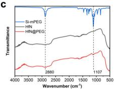
Fig. 5 Coating of laser-synthesized HfN-based NPs with PEG. (a) Hydrodynamic diameter distribution for HfN and HfN@PEG NPs in water and PBS buffer. (b) ζ-potential distribution for HfN NPs before and after coating with mPEG-Silane polymer. (c) FTIR spectra of mPEG-Silane polymer, HfN and HfN@PEG NPs.
