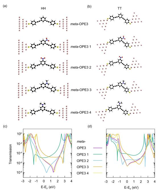
Fig. 5 (a) HH and (b) TT junction geometries of **meta-OPE3** and **meta-OPE3** 1–4 from top to bottom. Transmission curves based on the DFT+ $\Sigma$  approach for the **meta-OPE3** molecule and its derivatives **meta-OPE3** 1–4 in the (c) HH and (d) TT junction configurations.
