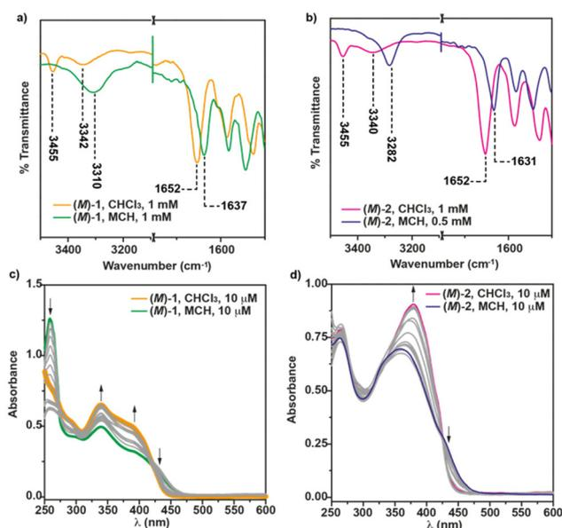
**Fig. 3** FTIR spectra of (**M**)-1 (a) and (**M**)-2 (b) in CHCl<sub>3</sub> and MCH. The dotted lines show the wavenumber values for the NH and Amide I stretching bands; UV-Vis spectra of (**M**)-1 (c) and (**M**)-2 (d) in CHCl<sub>3</sub>, MCH and in different MCH/CHCl<sub>3</sub> mixtures. Arrows in panel (c) and (d) show the absorption changes upon increasing the amount of the good solvent (CHCl<sub>3</sub>).
