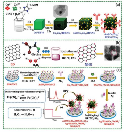
Fig. 12 Preparation of (A) Au@Cu<sub>5</sub>Zn<sub>8</sub>/HPCNC/Ab<sub>2</sub> and (B) NHG. (C) Preparation of immune-based electrochemical biosensors. <sup>160</sup>
