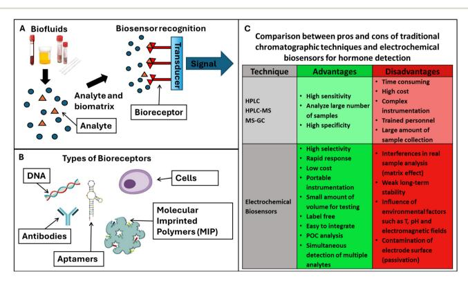
Fig. 3 Schematic representation of (A) biosensor components, (B) types of bioreceptors and (C) comparison between the pros and cons of the traditional techniques for hormone detection and electrochemical biosensors.
