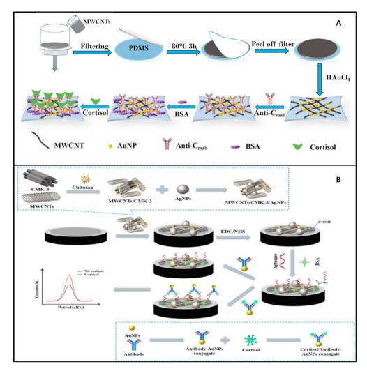
Fig. 7 (A) Stepwise fabrication of the immunosensor (Anti-Cmab/AuNPs/MWCNTs/PDMS);<sup>125</sup> (B) preparation and functioning of the cortisol sensor described by Huang et al. 126
