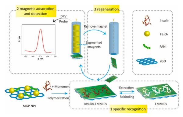
Fig. 11 Preparation and electrochemical detection operation of EMMIPs. 158
