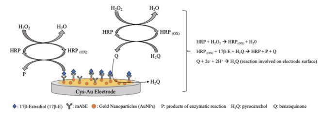
Fig. 9 Schematic presentation of the  $17-\beta$ -estradiol electrochemical immunosensor based on Cys-Au electrode modified with gold nanoparticles and anti- $17-\beta$ -estradiol monoclonal antibody. <sup>142</sup>
