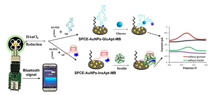
Fig. 13 Diagram of the simultaneous detection of insulin and glucose using the smartphone-assisted electrochemical aptasensor, measured by amperometric technique.<sup>170</sup>
