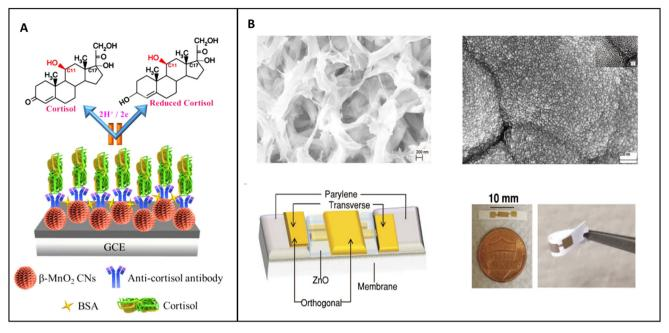
Fig. 8 (A) Schematic representation of  $MnO_2$  nanocacti electrochemical biosensor; <sup>128</sup> (B) TEM pictures of the polyamide matrix before and after the deposition of ZnO, scheme of the electrochemical biosensor and real-life image of the biosensor. <sup>129</sup>
