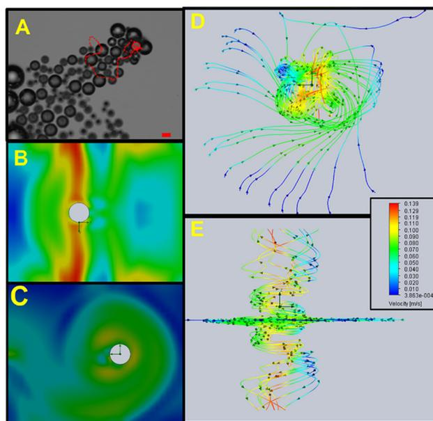
Fig. 3 (A) Time-lapse image showing the propulsion of a ZIF-8@Au@catalase micromotor (taken from Video S2†) and (B) corresponding schematic of the flow dynamics simulations of the  $Z$ - and  $X$ -axis sections. (C)  $Y$ - and  $X$ -axis sections. (D) Bottom view and (E) back view trajectories. Conditions:  $250 \mu\text{g L}^{-1}$  of Cu, 1% Triton X-100 and 10%  $\text{H}_2\text{O}_2$  as the fuel. Scale bar, 20  $\mu\text{m}$ .
