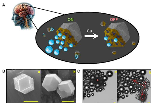
**Fig. 1** (A) Schematic of ZIF-8 composition and catalytic movement of the ZIF-8@Au@catalase micromotors through CSF. (B) SEM images showing the morphologies of ZIF-8 (a) and the ZIF-8@Au@catalase micromotors (b). Scale bars, 1  $\mu\text{m}$ . (C) Time-lapse microscopy images (taken from Video S1†) of the ZIF-8@Au@catalase micromotors after 0 s (a) and 2 s (b) navigation in water. Conditions: 1% Triton X-100 and 10%  $\text{H}_2\text{O}_2$  as the fuel. Scale bars, 10  $\mu\text{m}$ .
