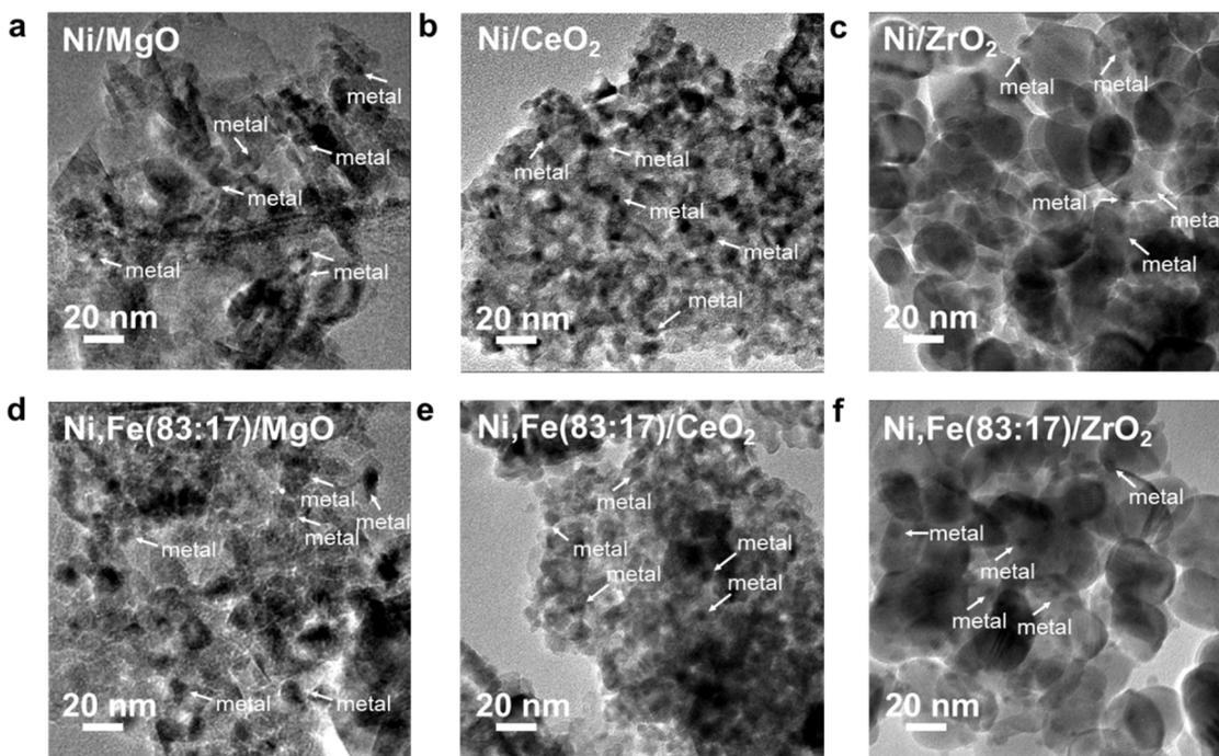
Fig. 5 TEM images for Ni–Fe monometallic and bimetallic catalysts supported on (a) & (d) MgO, (b) & (e) ZrO<sub>2</sub> and (c) & (f) CeO<sub>2</sub>.
