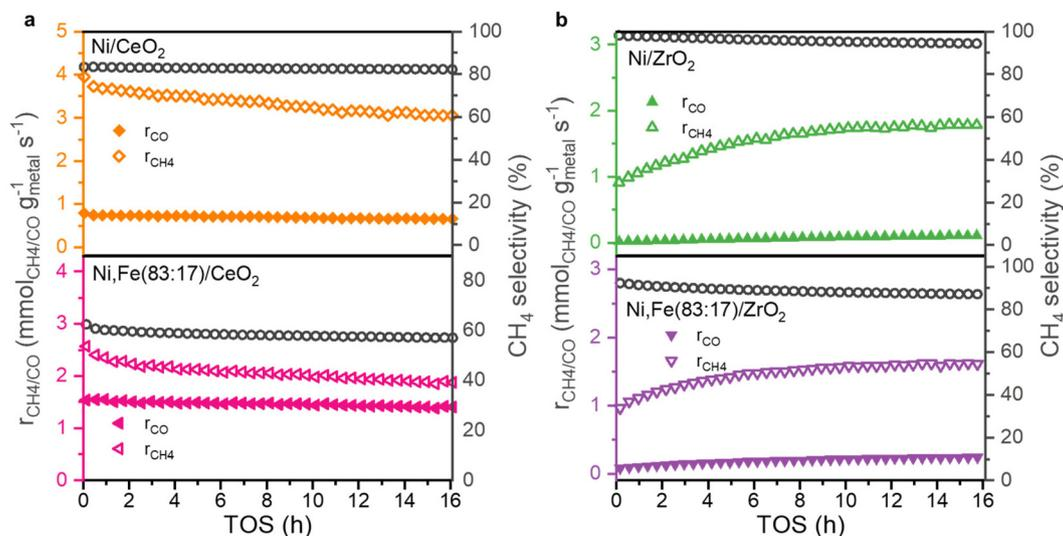
Fig. 6 Methanation and RWGS rates and selectivity towards CH<sub>4</sub> as a function of TOS for (a) CeO<sub>2</sub> and (b) ZrO<sub>2</sub>-supported monometallic and bi-metallic catalysts for 16 h TOS at 350 °C.
