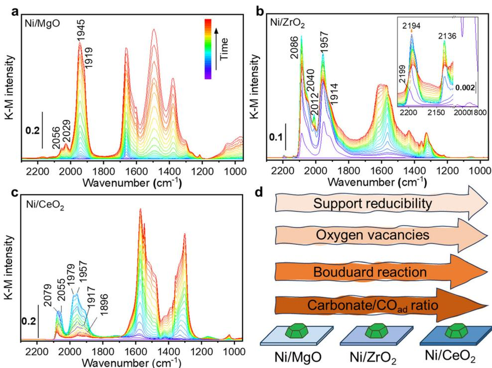
**Fig. 12** *In situ* DRIFTS spectra of (a) Ni/MgO, (b) Ni/ZrO<sub>2</sub> and (c) Ni/CeO<sub>2</sub> catalysts collected during CO adsorption, inset images in (b) representing the zoom-in spectra at features above 2100 cm<sup>-1</sup>. Illustration (d) of the structural properties changes in three different supported Ni Catalysts.
