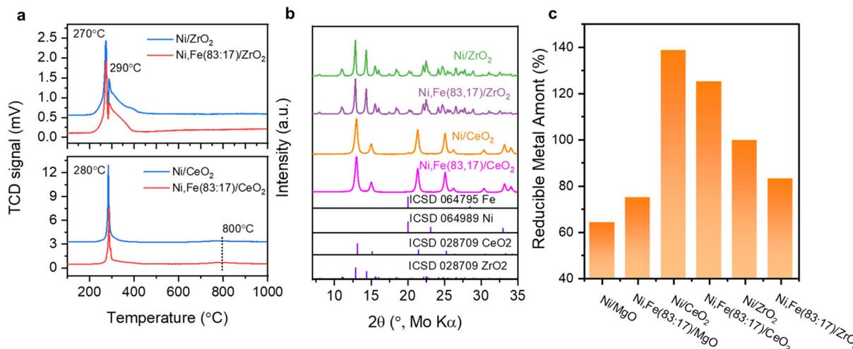
Fig. 4 (a) H<sub>2</sub>-TPR profile for Ni monometallic and Ni,Fe bimetallic catalysts supported on ZrO<sub>2</sub>, CeO<sub>2</sub>; (b) the PXRD patterns of the samples reduced isothermally at 450 °C and (c) the estimated degree of reduction, where valued beyond 100% refer to co-reduction of support species.
