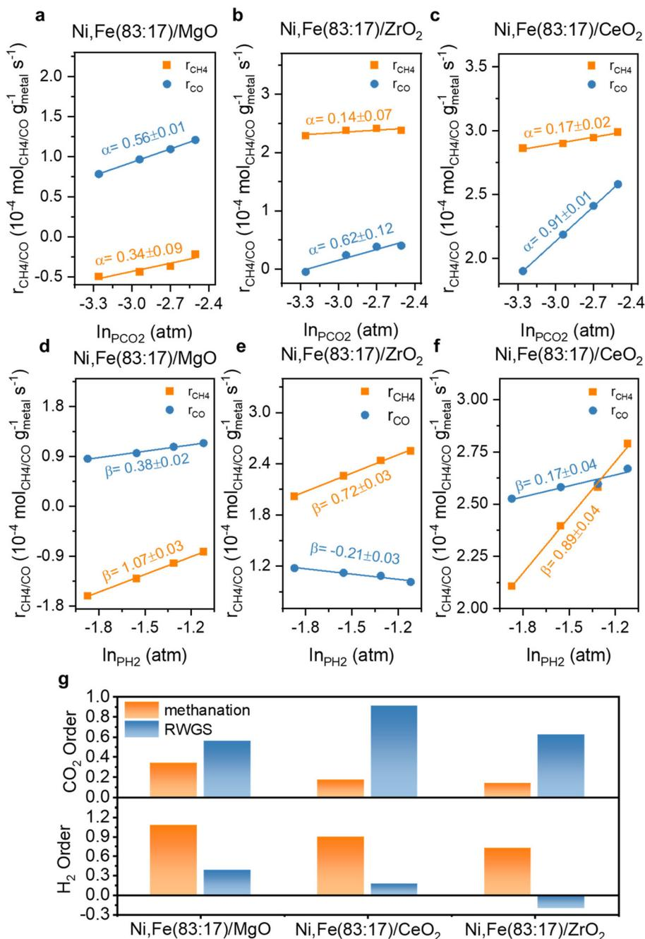
**Fig. 11** The reaction order of CO<sub>2</sub> ( $\alpha$ ) and H<sub>2</sub> ( $\beta$ ) at 350 °C for Ni,Fe bimetallic catalysts supported on (a) & (d) MgO, (b) & (e) ZrO<sub>2</sub> and (c) & (f) CeO<sub>2</sub> and (g) their comparison.
