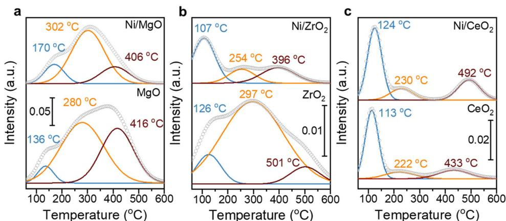
Fig. 8  $\text{CO}_2$ -TPD profiles at  $10 \text{ }^\circ\text{C min}^{-1}$  for (a) MgO, (b)  $\text{ZrO}_2$ , (c)  $\text{CeO}_2$  supports, and their corresponding Ni loaded catalysts where grey dots represent the smoothed raw profiles and the solid color lines indicate the fitting results for weak, medium and strong basic sites at different temperatures.
