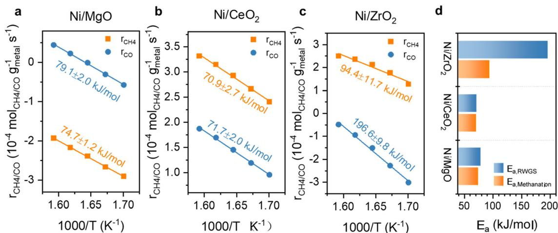
Fig. 9 Arrhenius plots with calculated  $E_a$  for Ni catalysts supported on (a) MgO, (b) CeO<sub>2</sub>, (c) ZrO<sub>2</sub> and (d) comparison of their  $E_a$ s for RWGS and methanation.
