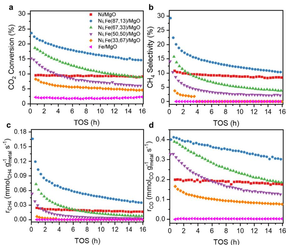
**Fig. 2** (a) CO<sub>2</sub> conversion, (b) selectivity towards CH<sub>4</sub>, (c) methanation rate and (d) RWGS rate as a function of TOS for MgO-supported catalysts with various Ni : Fe ratios at 350 °C.
