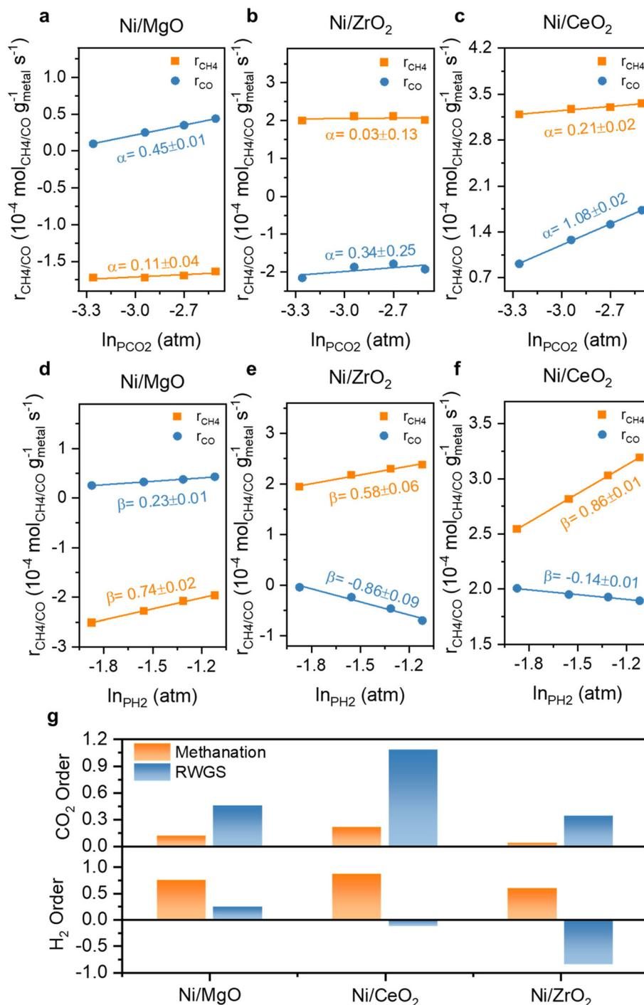
**Fig. 10** The reaction order of CO<sub>2</sub> ( $\alpha$ ) and H<sub>2</sub> ( $\beta$ ) at 350 °C for Ni monometallic catalysts supported on (a) & (d) MgO, (b) & (e) ZrO<sub>2</sub> and (c) & (f) CeO<sub>2</sub> and (g) their comparison.
