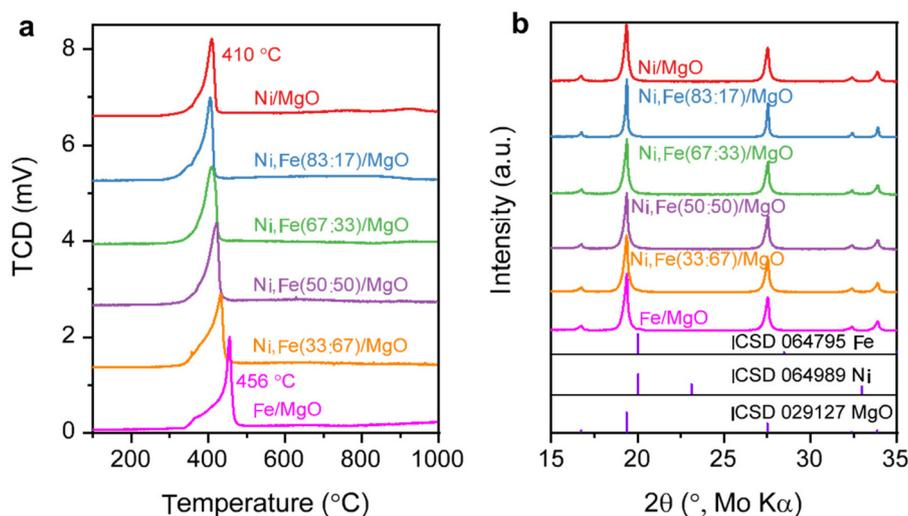
**Fig. 1** (a) H<sub>2</sub>-TPR profile for Ni,Fe monometallic and bimetallic catalysts supported on MgO and (b) their PXRD patterns after isothermal reduction of 450 °C.
