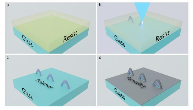
Fig. 1 Overview of the fabrication process. (a) Negative-tone photoresist (yellow) drop-cast on glass substrate (blue). (b) Exposure of wavelength  $\lambda$  = 405 nm laser. (c) Unexposed resist is removed through solvent development and polymer (purple) nanowires remain. (d) Thermal evaporation of Permalloy (Ni<sub>81</sub>Fe<sub>19</sub>, grey) is used to coat the polymer nanowires.
