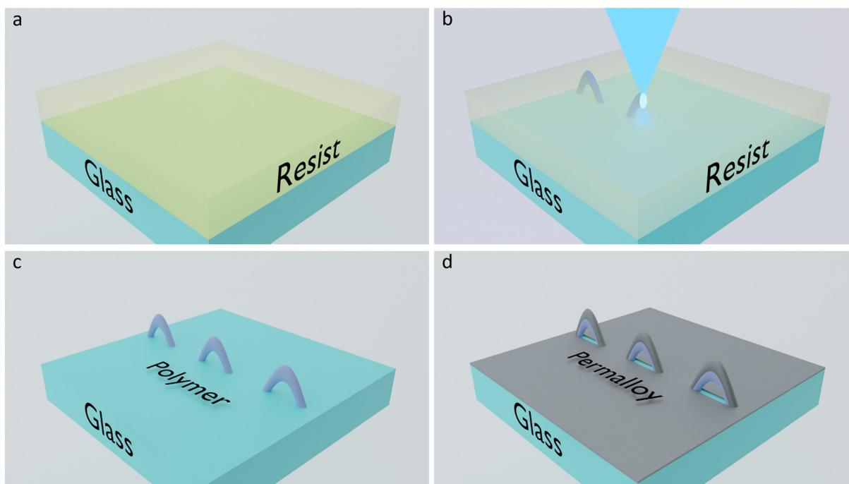
**Fig. 1** Overview of the fabrication process. (a) Negative-tone photoresist (yellow) drop-cast on glass substrate (blue). (b) Exposure of wavelength  $\lambda = 405 \text{ nm}$  laser. (c) Unexposed resist is removed through solvent development and polymer (purple) nanowires remain. (d) Thermal evaporation of Permalloy ( $\text{Ni}_{81}\text{Fe}_{19}$ , grey) is used to coat the polymer nanowires.
