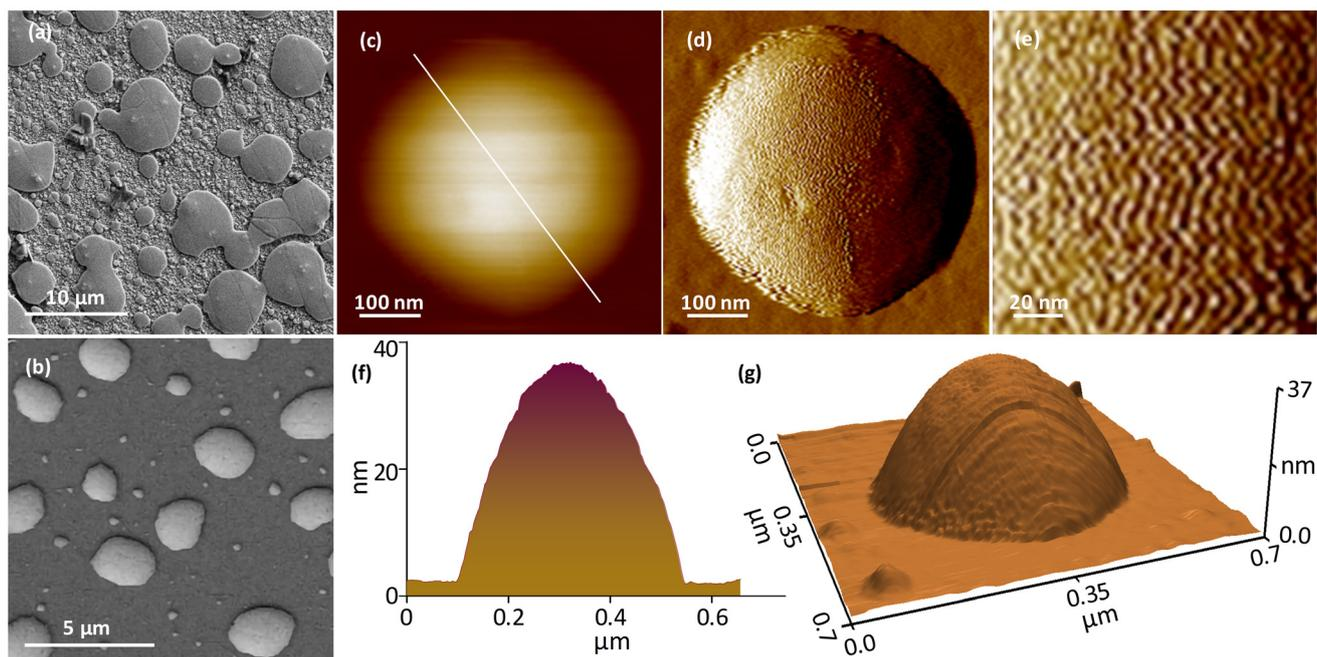
**Fig. 3** (a and b) FESEM images of (a)  $C_3$ -NC and (b)  $C_9$ -NC assemblies. (c and d) High-resolution tapping mode AFM (c: topography and d: amplitude) images of the single superstructure derived from  $C_3$ -NC. (e) A zoomed and focused AFM image captured from the top surface of the  $C_3$ -NC assembly showing the NC direction in the assembly. (f and g) The height profile and three-dimensional (3D) AFM image of the same assembly.
