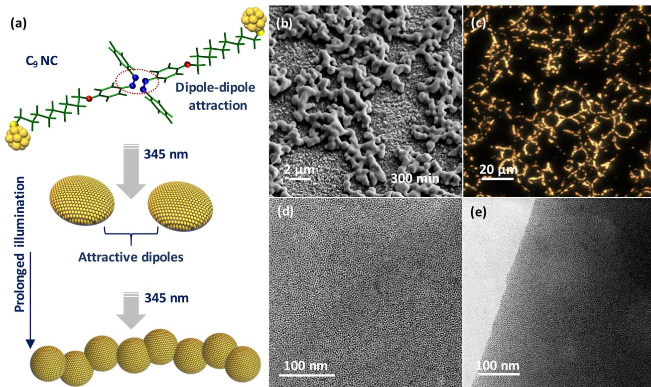
**Fig. 5** (a) The schematic depicts the formation of a chain-like assembly. (b) FESEM and (c) dark-field scattering images of the chain-like assembly. (d and e) TEM micrographs from the surface and edge of the chain-like assembly.
