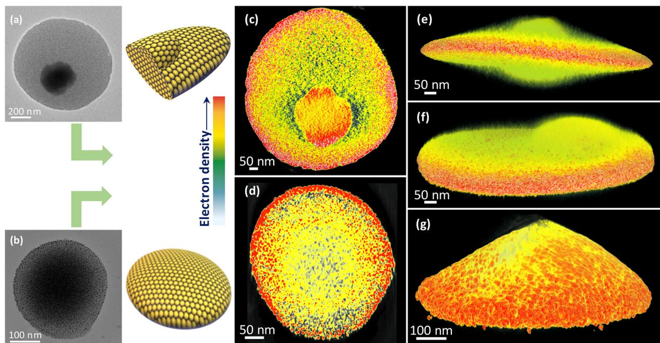
**Fig. 4** (a and b) TEM images and (c and d) corresponding cross-sectional views from the ET reconstructed images of (a and c)  $C_3$ -NC and (b and d)  $C_9$ -NC superstructures. (e–g) The 3D-reconstructed tomograms of (e and f)  $C_3$ -NC and (g)  $C_9$ -NC superstructures in different orientations.
