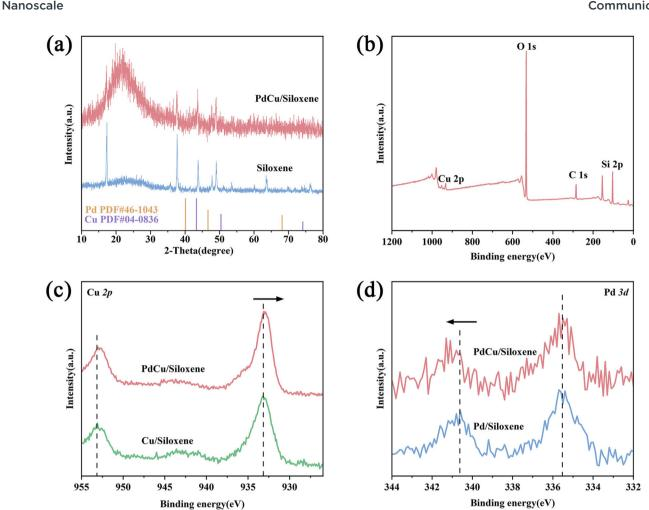
Fig. 2 (a) The XRD spectra of siloxene and PdCu/siloxene. (b) XPS survey spectra pf PdCu/siloxene. (c) Cu 2p XPS spectra of different catalysts, (d) Pd 3d XPS spectra of different catalysts.
