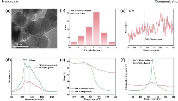
Fig. 4 (a) TEM image, (b) the diameter distributions, (c) Pd 3d XPS spectra of PdCu/siloxene-tested. (d) Raman spectra, (e) and (f) TG-MS curves of PdCu/siloxene-tested and PdCu/SiO2-tested.
