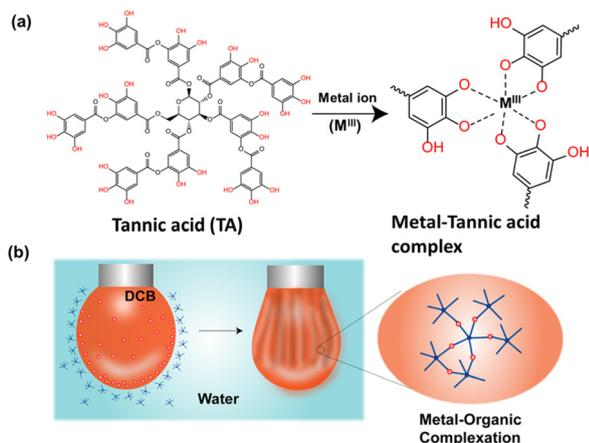
**Fig. 1** (a) Chemical structure of TA and  $\text{M}^{\text{III}}$ –TA complexation. (b) Schematic representation of  $\text{M}^{\text{III}}$ –TA complexation at the oil–water interface.
