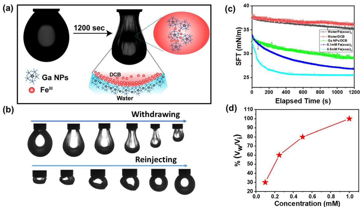
**Fig. 6** (a) Schematic representation of TA-coated Ga NP–metal complexation at the oil–water interface. (b) Snapshot showing droplet morphology during withdrawal and reinjection. (c) Time evolution of interfacial tension and (d) surface coverage of Ga NPs with Fe<sup>III</sup> metal ions (1 mM).
