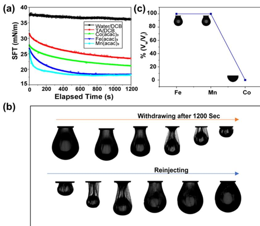
**Fig. 2** (a) Time evolution of interfacial tension of TA and  $M^{III}$ -TA complexes. (b) Snapshot showing droplet morphology during the withdrawing and reinjection processes. (c) Surface coverage of the pendant droplets with TA ( $1 \text{ mg mL}^{-1}$ ) and  $M^{III}$  ions ( $1 \text{ mM}$ ).
