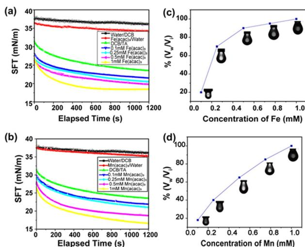
**Fig. 3** (a) Time evolution of interfacial tension of TA ( $1 \text{ mg mL}^{-1}$ ) with varying  $\text{Fe}^{III}$  concentration and (b) TA ( $1 \text{ mg mL}^{-1}$ ) varying  $\text{Mn}^{III}$  concentration. (c) Surface coverage of TA ( $1 \text{ mg mL}^{-1}$ ) with varying  $\text{Fe}^{III}$  concentration and (d) TA ( $1 \text{ mg mL}^{-1}$ ) with varying  $\text{Mn}^{III}$  concentration.
