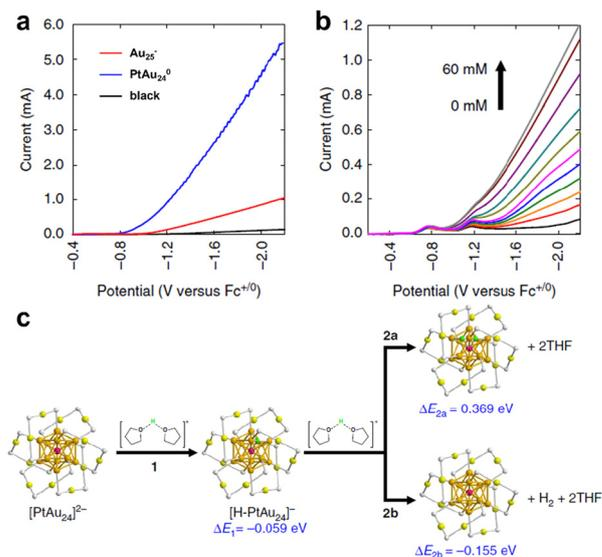
**Fig. 5** (a) LSV curves of THF containing 0.1 M  $\text{Bu}_4\text{NPF}_6$  and 1.0 M TFA solution for  $\text{Au}_{25}(\text{SR})_{18}^-$  and  $\text{PtAu}_{24}(\text{SR})_{18}^0$  clusters. (b) The polarization curves of 1 mM  $\text{PtAu}_{24}(\text{SR})_{18}^0$  in THF with different TFA concentrations. (c) The calculated energy of  $\text{H}_2$  evolution on  $\text{PtAu}_{24}(\text{SR})_{18}^0$ . Reproduced with permission from ref. 58. Copyright 2023 Nature Publishing Group.
