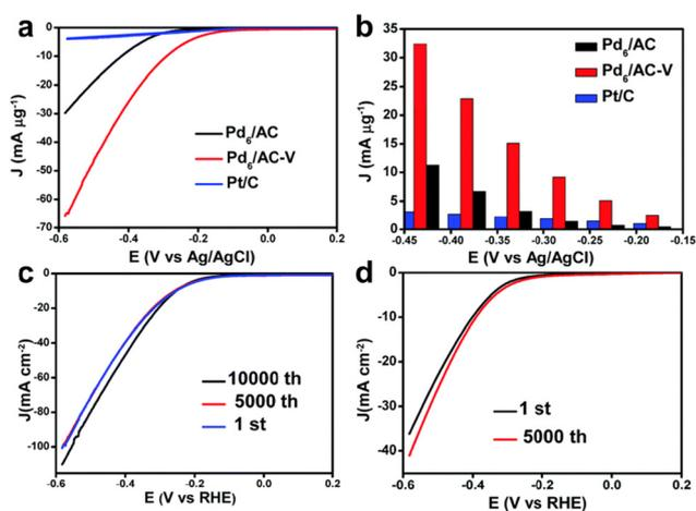
**Fig. 1** (a) The polarization curves of  $Pd_6/AC$ ,  $Pd_6/AC-V$  and commercial Pt/C for the HER. (b) The mass activities of the three catalysts at different applied potentials. (c) ADTs of  $Pd_6/AC-V$ . (d) ADTs of  $Pd_6/AC$ . All the LSV curves were obtained for a solution of 0.5 M  $H_2SO_4$  with a scanning rate of 5  $mV s^{-1}$ . Reproduced with permission from ref. 43. Copyright 2017 Royal Society of Chemistry.
