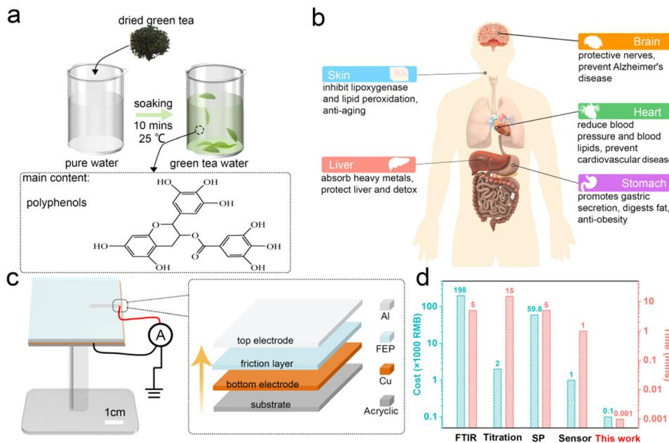
**Fig. 1** (a) Preparation of green tea water. The molecular structural formula of GTPs is shown at the bottom. (b) Benefits of GTPs to the human body. (c) Schematic diagram of the layered self-powered droplet sensor. (d) Comparison of the self-powered droplet sensor with FTIR, titration, SP, and sensor in terms of cost and time consumption.
