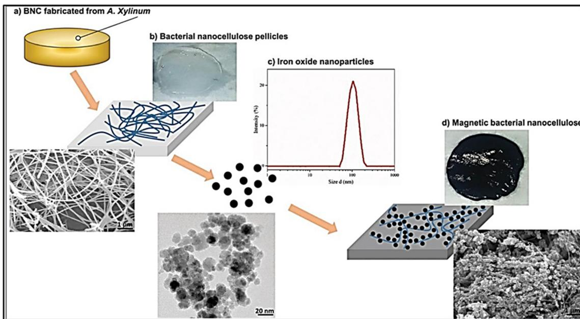
**Fig. 10** (a) BNC produced by the bacterium *A. xylinum*; (b) digital and SEM pictures of the BNC hydrogel membrane; (c) transmission electron microscopy and dynamic light scattering analysis of the  $\text{Fe}_3\text{O}_4$  NPs; and (d) comprehensive SEM evaluation of the  $\text{Fe}_3\text{O}_4$ /BNC digital image, which shows the strong bonding of the  $\text{Fe}_3\text{O}_4$  NPs to the BNC fibres. Reproduced with permission from ref. 104. Copyright 2017, Wiley.
