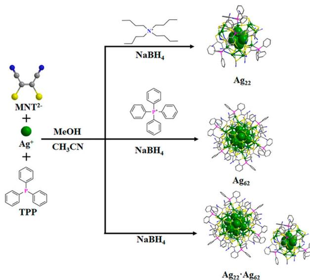
**Fig. 2** Synthetic route for counter cation-directed synthesis of  $[\text{Ag}_{62}(\text{MNT})_{24}(\text{TPP})_6]^{8-}$  and  $[\text{Ag}_{22}(\text{MNT})_{12}(\text{TPP})_4]^{4-}$  NCs. Color legend: green, Ag; pink, P; yellow, S; blue, N; gray, C. Reproduced with permission from ref. 43. Copyright (2023).
