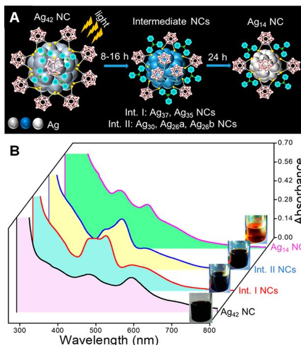
**Fig. 6** (A) Schematic of the light-activated conversion of Ag<sub>42</sub> to Ag<sub>14</sub> through intermediate clusters. (B) UV-vis absorption spectra of Ag<sub>42</sub> NC before and after light irradiation along with the mixture of intermediate clusters. Insets: photographs of the color change of cluster solutions during the light-irradiation. Reproduced with permission from ref. 86. Copyright (2021).
