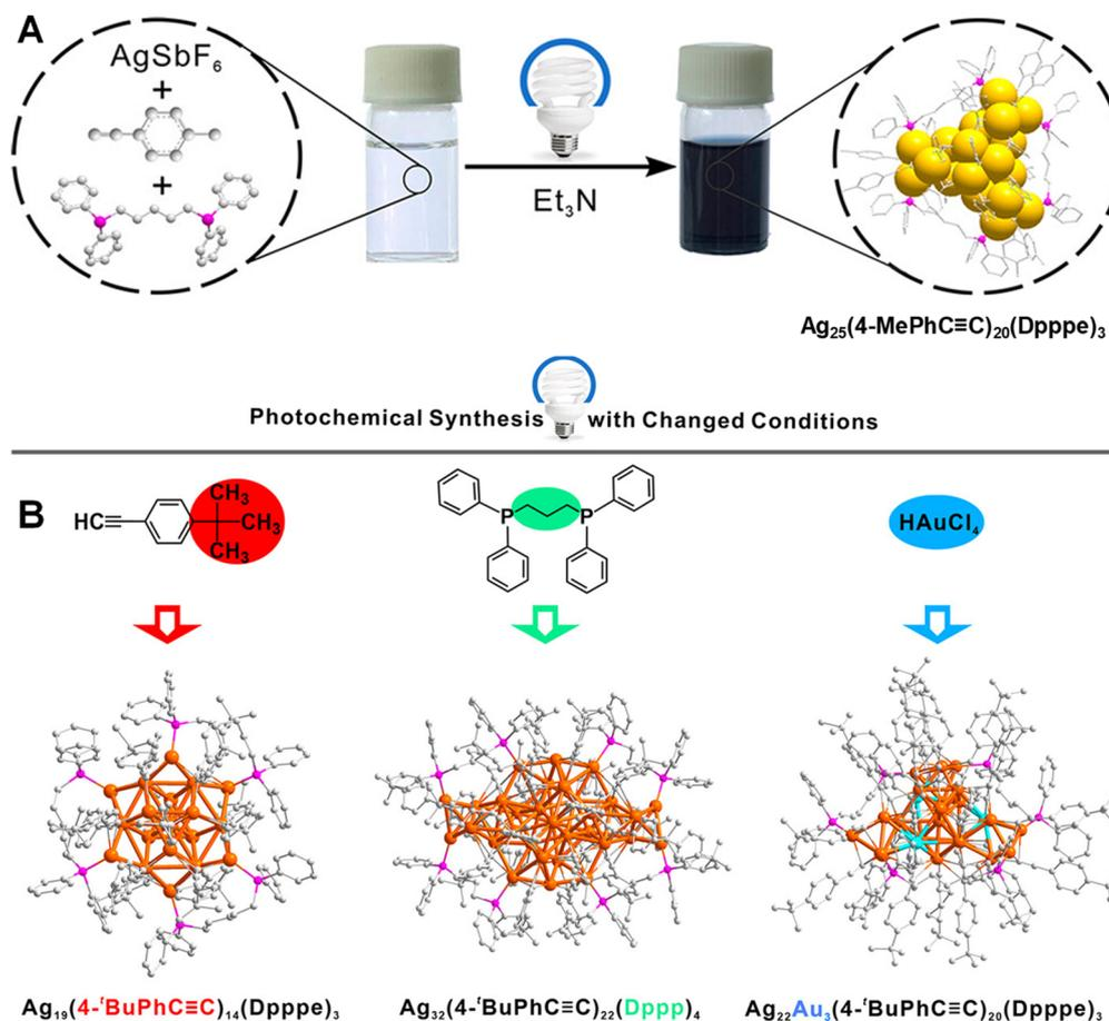
**Fig. 3** (A) Schematic illustration of the photochemical synthesis of  $\text{Ag}_{25}$  NCs by irradiating the precursor solution by <455 nm light for 24 h. (B) Schematic of the photochemical synthesis of Ag NCs of different size, structure and composition. Reproduced with permission from ref. 53. Copyright (2023).
