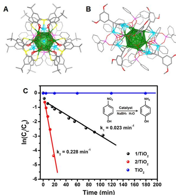
**Fig. 10** Molecular structures of (A) thiacalixarene- and (B) alkynyl-protected Ag<sub>21</sub> NCs. (C) Catalytic activity of Ag<sub>21</sub>(thiacalixarene)/TiO<sub>2</sub> (1/TiO<sub>2</sub>) and Ag<sub>21</sub>(alkynyl)/TiO<sub>2</sub> (2/TiO<sub>2</sub>) and TiO<sub>2</sub> in nitrophenol reduction. Reproduced with permission from ref. 118. Copyright (2022).
