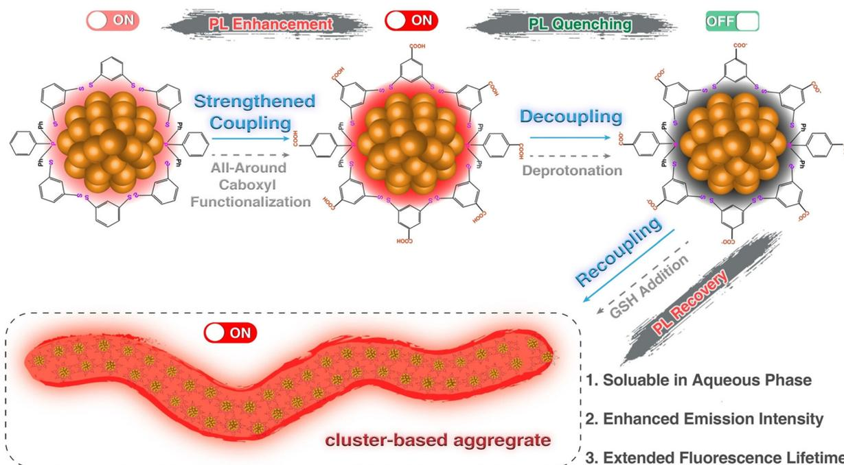
**Fig. 5** Schematic of the emission enhancement of the  $\text{Ag}_{29}\text{-AC}$  NC through the strengthened coupling, the emission quenching of  $\text{Ag}_{29}\text{-AC}$  in the aqueous phase caused by molecular decoupling, and the emission recovery of the  $\text{Ag}_{29}\text{-AC}$  NC by its supramolecular recoupling in the presence of reduced glutathione (GSH). Reproduced with permission from ref. 76. Copyright (2024).
