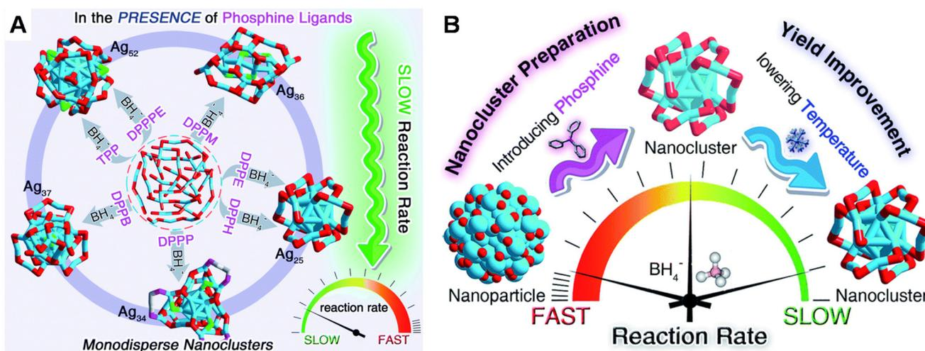
Fig. 1 Schematic illustration of (A) first-level and (B) dual-level kinetic control *via* introducing phosphine ligands and low reaction temperature, leading to synthesis of a series of Ag NCs with improved yields. Reproduced with permission from ref. 36. Copyright (2022).
