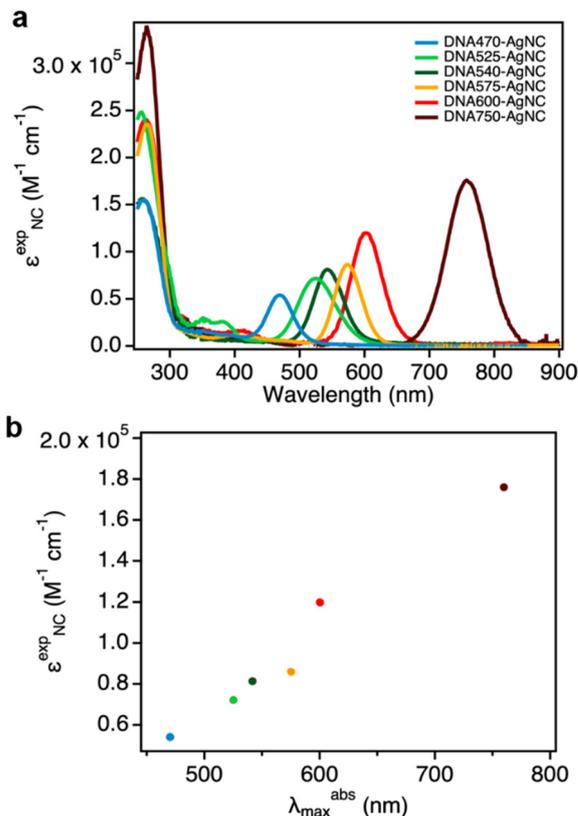
**Fig. 2** (a) Normalized absorption spectra of selected DNA-AgNCs expressed in units of  $\epsilon$  ( $\text{M}^{-1} \text{ cm}^{-1}$ ); (b) experimentally-determined molar absorption coefficients ( $\epsilon_{\text{NC}}^{\text{exp}}$ ) as a function of absorption maxima of the AgNC related peak in the Vis/NIR range ( $\lambda_{\text{max}}^{\text{abs}}$ ).
