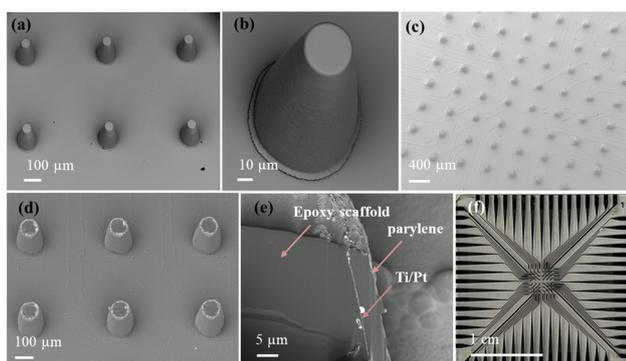
**Fig. 3** SEM images of micropillars and an optical image of the overall layout of the MEA. (a) An image of epoxy-based pillars, (b) a close-up image of an individual pillar, (c) epoxy-based 3D electrodes after laser ablation of the tips, (d) a close-up image of individual ring electrodes at the tip of the pillar. (e) A cross-sectional view of an individual pillar electrode obtained by focused-ion-beam milling. (f) An overall view of the MEA layout.
