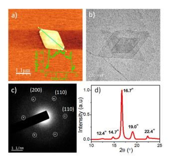
Fig. 1 (a) AFM image (inset: showing height profile of the 2D platelet) and (b) TEM image of the self-assembled diamond-shaped platelet of PTZ-P1;  $C = 0.05 \text{ mg mL}^{-1}$ ; (c) Selected area electron diffraction (SAED) patterns obtained from the diamond platelet of PTZ-P1 in iPrOH; C = 0.05 mg mL<sup>-1</sup>; (d) WAXRD of PTZ-P1. The powdered sample was prepared by slowly drying its self-assembled dispersion in iPrOH.
