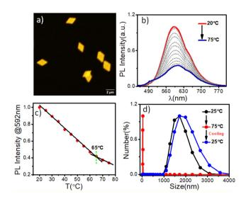
Fig. 2 (a) CLSM image of self-assembled PTZ-P1 in iPrOH; C = 0.05 mg mL<sup>-1</sup>; (b) Variable-temperature (VT) photoluminescence (PL) studies of PTZ-P1 ( $\lambda_{ex}$  = 430 nm); excitation and emission slit = 2.5 nm/2.5 nm; (c) PL-Intensity vs. temperature plot from (b); (d) VT-DLS data of PTZ-P1; C  $= 0.1 \text{ mg mL}^{-1}$
