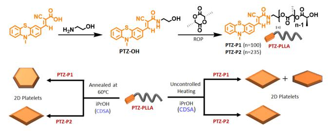
Scheme 1 Top: schematic representation of the synthesis of PTZ-PLLA by ROP; bottom: crystallization-driven self-assembly (CDSA) of poly(Llactide) homopolymers, PTZ-P1 and PTZ-P2 in isopropanol (iPrOH) under different conditions, and morphological modulation in PTZ-P1 2D platelets from a mixture of orange-emitting lozenge (diamond) and truncated-lozenge to hexagon.
