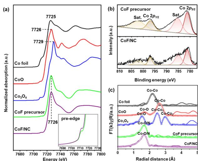
**Fig. 3** (a) XANES spectra of Co foil, CoO,  $\text{Co}_3\text{O}_4$ , CoF precursor, and CoF/NG. (b) Deconvoluted XPS Co 2p spectra of the CoF precursor and CoF/NG. (c) EXAFS fitting results of Co foil, CoO,  $\text{Co}_3\text{O}_4$ , CoF precursor, and CoF/NG.
