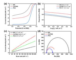
Fig. 4 Electrochemical performance of NG, CoF/NG, and Pt/C. (a) LSV polarization curves, (b) Tafel slopes, (c) double-layer capacitance measurements to determine ECSA, and (d) EIS curves.
