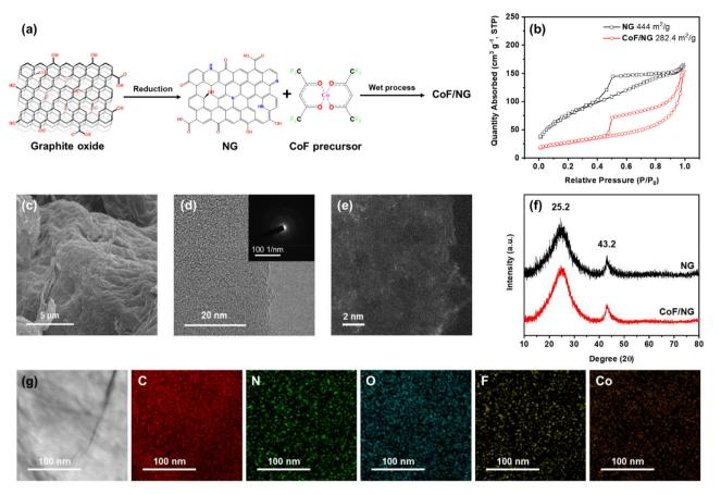
Fig. 1 (a) Scheme of this work. (b)  $N_2$  adsorption-desorption isotherm plots of NG and CoF/NG. Morphological characteristics of CoF/NG (c) SEM, (d) TEM, and (e) STEM images. (f) XRD patterns of NG and CoF/NG. (g) TEM elemental mapping images of CoF/NG.
