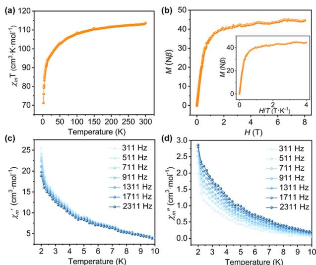
**Fig. 2** For **1**. (a) Temperature-dependence of  $\chi_m T$  in the temperature range of 2–300 K; (b) field-dependence of magnetization at 2 K. Inner: *M* vs. *H/T* plots. (c and d) Temperature-dependent behavior of the in-phase ( $\chi'_m$ ) and out-of-phase ( $\chi''_m$ ) in zero static fields at 2–10 K.
