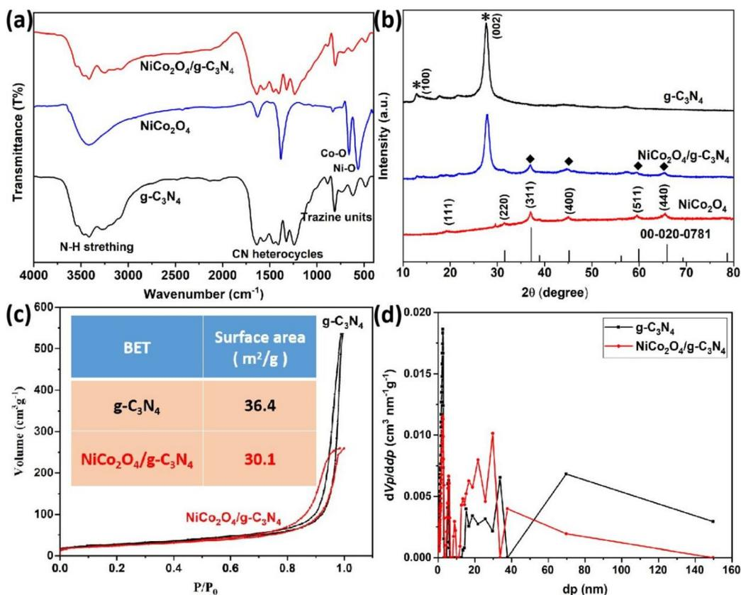
**Fig. 3** FT-IR spectra (a) and XRD pattern (b) of  $g\text{-C}_3\text{N}_4$ ,  $\text{NiCo}_2\text{O}_4$  and  $\text{NiCo}_2\text{O}_4/g\text{-C}_3\text{N}_4$ . The adsorption–desorption isotherm curves (c) and porosity scale distribution (d) of  $g\text{-C}_3\text{N}_4$  and  $\text{NiCo}_2\text{O}_4/g\text{-C}_3\text{N}_4$ .
