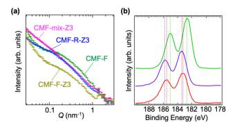
Fig. 4 (a) SANS patterns of CMF-F (green), CMF-F-Z3 (yellow), CMF-R-Z3 (purple), and CMF-mix-Z3 (pink), respectively. (b) XPS spectra of Zr 3d in CMF-F-Z3 (red), ZrCl<sub>2</sub>O·8H<sub>2</sub>O (purple), ZrO<sub>2</sub> (green). The red, purple, and green dashed lines represent the peak positions of CMF-F-Z3, ZrCl<sub>2</sub>O·8H<sub>2</sub>O, and ZrO<sub>2</sub>, respectively.
