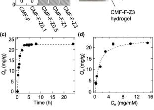
Fig. 5 (a)  $R_{\rm eff}$  values for CMF-F and CMF-F-Zx ( $x=0.1,\,0.5,\,1,\,{\rm or}$  3) in an aqueous solution of NaF (1 mmol L<sup>-1</sup>). (b) Photographs of CMF-F-Z3 during (left) and after (right) immersion in aqueous solution. (c)  $Q_{\rm e}$  values of CMF-F-Z3 in an aqueous solution of NaF (10 mmol L<sup>-1</sup>) with reaction time. (d) Fluoride adsorption isotherm analysis for CMF-F-Z3. The dashed line represents the fitting curve obtained using the Langmuir model.
