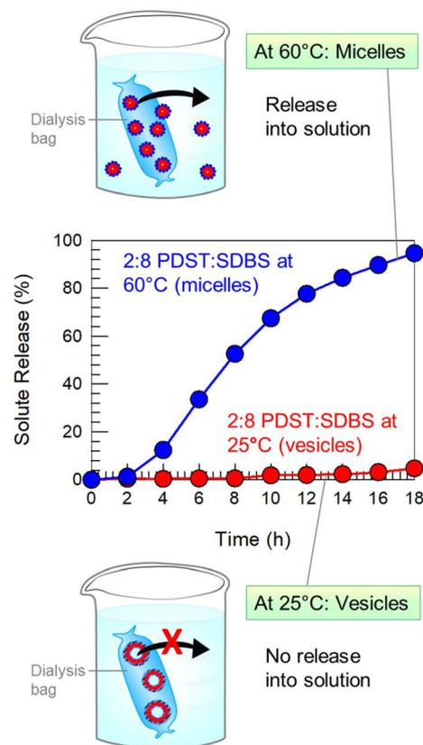
**Fig. 10** Switching on the release of solutes by exploiting a VMT. Cumulative release of the solute (a cationic dye) *vs.* time from dialysis bags containing 1% of 2:8 PDST–SDBS mixtures at 25 °C and 60 °C. At 25 °C, the dye is bound to vesicles, which are too large to pass through the bag. At 60 °C, a VMT occurs, *i.e.*, the vesicles transform into micelles (with bound dye), which leak out of the bag.
