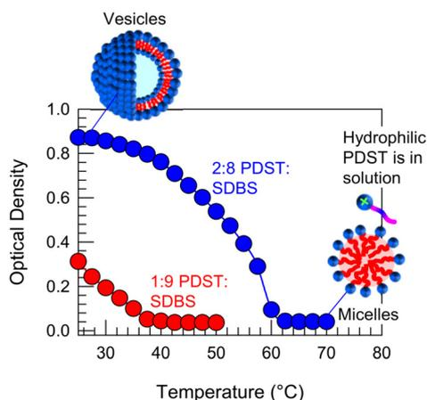
**Fig. 9** Heat-induced VMT in PDST–SDBS samples. Optical density (OD) *vs.* temperature for 1:9 and 2:8 PDST : SDBS vesicles. The OD decays to zero, indicating a VMT upon heating. The effect is reversible and the micelles revert to vesicles when cooled.
