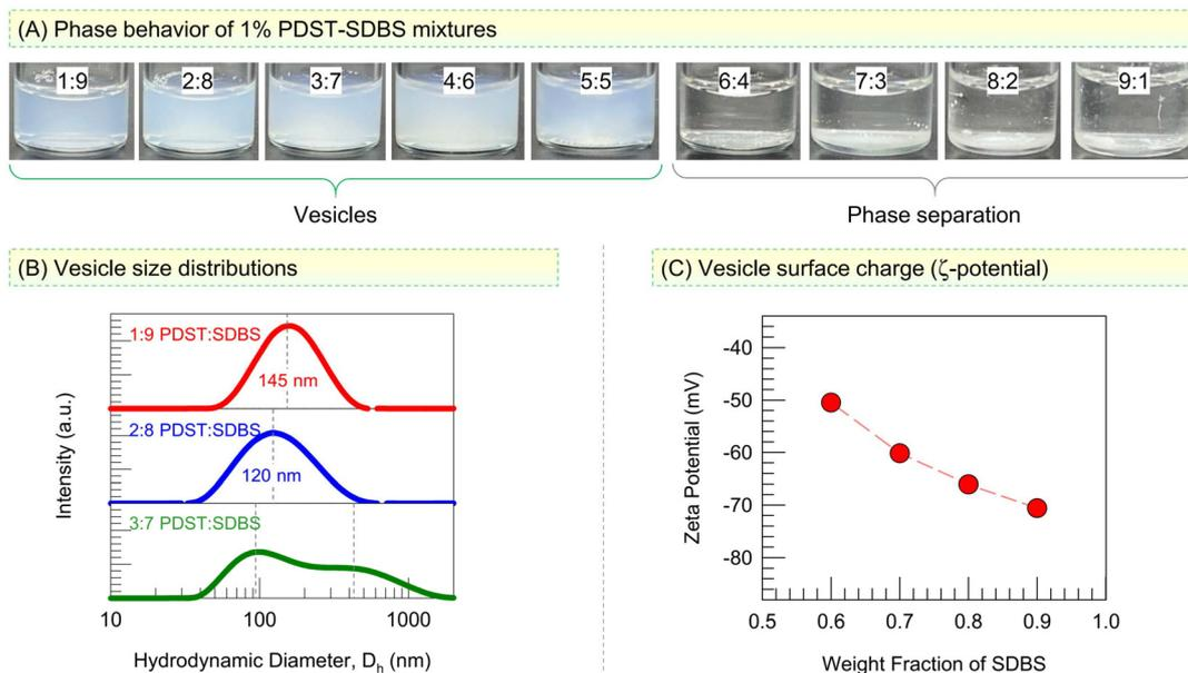
**Fig. 2** PDST–SDBS vesicles and their characterization. (A) Vial photos of 1% PDST–SDBS in phosphate buffer show that vesicles (bluish samples) form between 1 : 9 and 5 : 5 PDST : SDBS weight ratios. At higher PDST, phase separation occurs. (B) Size distributions from DLS give diameters around 120 to 150 nm for the vesicles. (C) The  $\zeta$ -potential of the vesicles is plotted vs. the fraction of anionic SDBS.
