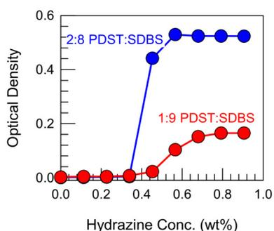
**Fig. 7** Reversal of VMT by a reducing agent. First, 1:9 and 2:8 PDST:SDBS vesicles are converted to micelles by adding 15% H<sub>2</sub>O<sub>2</sub> and incubating for 2 days. Then the reducing agent, hydrazine is added at different concentrations and the optical density (OD) is measured. OD increases in a sigmoidal fashion, reflecting the re-formation of vesicles.
