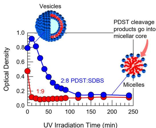
**Fig. 8** Light-induced VMT in PDST–SDBS samples. (A) UV light cleaves PDST into hydrophobic by-products and acid. Thus, PDST is no longer an amphiphile after this cleavage. (B) Optical density (OD) vs. UV irradiation time for 1:9 and 2:8 PDST:SDBS vesicles. The OD decays to zero, indicating a UV-induced VMT.
