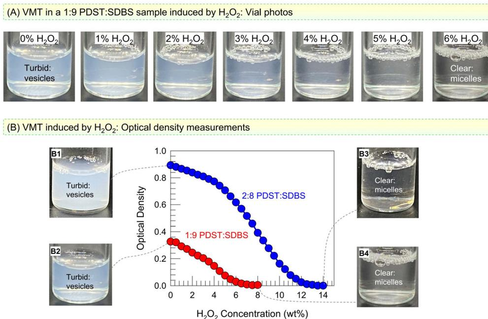
**Fig. 3** ROS-induced VMT in PDST–SDBS samples. (A) Photos of a 1:9 PDST–SDBS vesicle sample at various H<sub>2</sub>O<sub>2</sub> concentrations. The sample turns from turbid to clear, indicating a VMT. (B) Optical density (OD, a measure of turbidity) as a function of H<sub>2</sub>O<sub>2</sub> for 1:9 and 2:8 PDST:SDBS mixtures. In both cases, the turbidity decreases to zero, indicating VMTs. Photos of the end-points confirm the turbidity changes.
