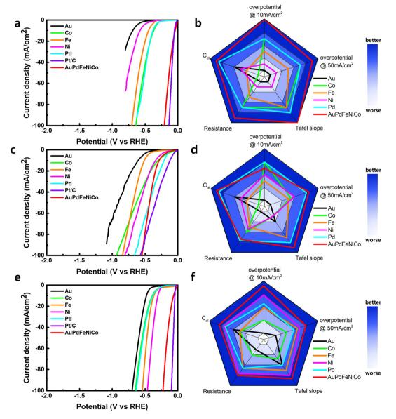
Fig. 4 HER electrocatalysis in acidic, neutral, and alkaline electrolyte. HER polarization curves of Au, Pd, Fe, Ni, Co, AuPdFeNiCo, and Pt/C in (a) 0.5M H<sub>2</sub>SO<sub>4</sub>, (c) 1M PBS, (e) 1M KOH, corresponding radar chart comparison of the potential characteristics of the electrocatalysts in(b) 0.5M H<sub>2</sub>SO<sub>4</sub>, (d) 1M PBS, and (f) 1M KOH.
