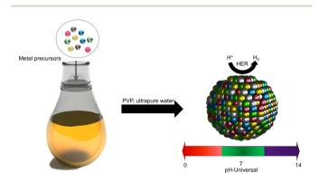
Scheme 1 The synthesis method for AuPdFeNiCo HEA nanoparticles.
