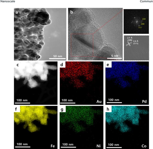
Fig. 1 HR-TEM and STEM-EDS characterization of AuPdFeNiCo HEA NPs. (a) Representative HR-TEM image of AuPdFeNiCo HEA NPs and (b) zoomed in view of the HR-TEM image with the insert shows the fast Fourier transformation (FFT). (c) STEM image of the corresponding energy dispersive spectroscopy (EDS) elemental mapping of (d) Au, (e) Pd, (f) Fe, (g) Ni, and (h) Co.
