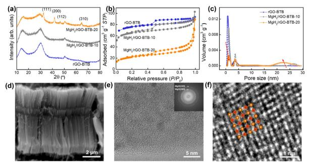
Fig. 2 (a) X-ray diffraction patterns, (b) N<sub>2</sub> adsorption-desorption isotherms and (c) NLDFT pore size distribution of rGO-BTB, MgH<sub>2</sub>/rGO-BTB-10 and MgH<sub>2</sub>/rGO-BTB-20. (d) SEM image of MgH<sub>2</sub>/rGO-BTB-10; (e) TEM image of MgH<sub>2</sub>/rGO-BTB-10, the insert shows the corresponding fast Fourier transform pattern; (f) HRTEM image of MgH<sub>2</sub>/rGO-BTB-10, overlay: MgO atomic structure.
