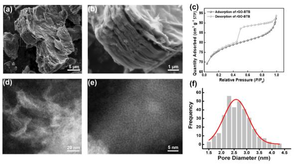
Fig. 1 (a) and (b) SEM images of rGO-BTB; (c)  $N_2$  adsorption—desorption isotherm of rGO-BTB, inset BJH pore size distribution of rGO-BTB. (d) STEM image of rGO-BTB. (e) STEM image zoomed in from (d). (f) The pore size distribution calculated from (e).
