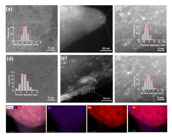
Fig. 3 (a) bright-field and (b) and (c) dark-field TEM images of  $MgH_2/rGO$ -BTB-10, the insets of (a) and (c) show the corresponding particle size distribution of the image. (d) bright-field and (e) and (f) dark-field TEM images of  $MgH_2/rGO$ -BTB-20, the insets of (d) and (f) show the corresponding particle size distribution of the image. The bottom panels: HAADF-STEM and EDS elemental maps for C, Mg, and C combined with Mg in  $MgH_2/rGO$ -BTB-10.
