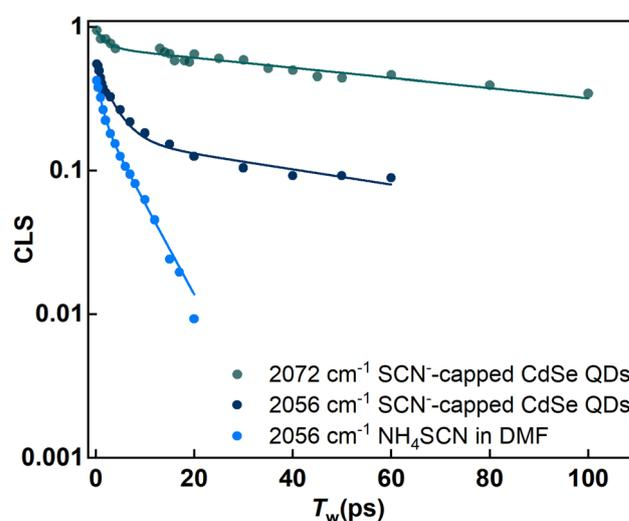
Fig. 4  $T_w$ -dependent CLS of the 2072 cm<sup>-1</sup> peak in SCN<sup>-</sup>-capped CdSe QDs corresponding to the bound ligands (green) shows the slowest decay and that of the 2056 cm<sup>-1</sup> peak corresponding to the free ions (blue) in the absence of QDs shows the fastest decay. The CLS decay of the 2056 cm<sup>-1</sup> peak in the presence of CdSe QDs shows a bi-exponential decay.
