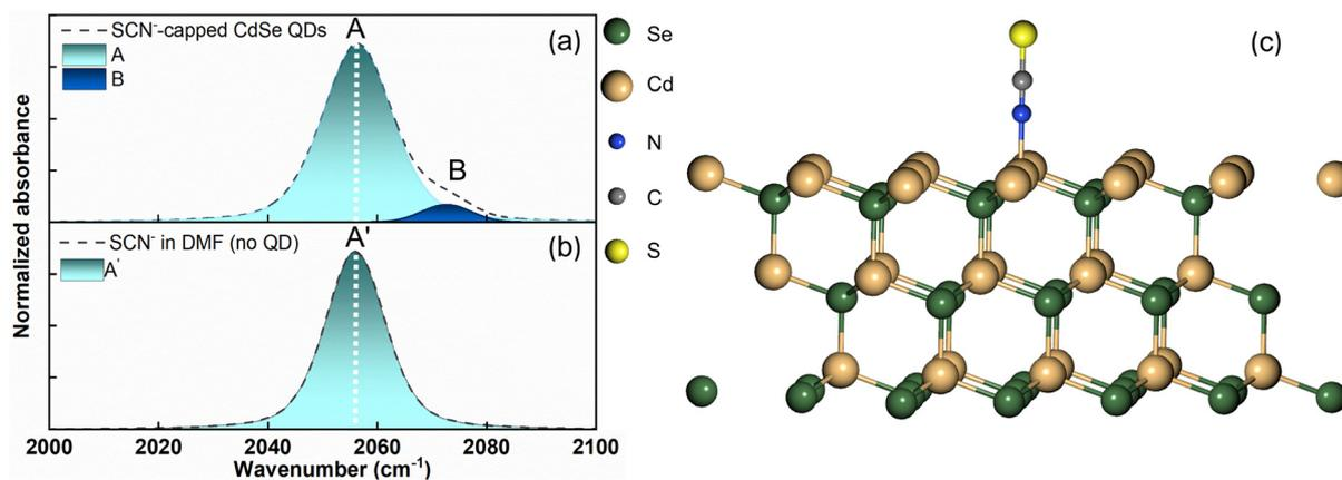
Fig. 2 (a) The FTIR spectrum of the C≡N stretching for SCN<sup>-</sup>-capped CdSe QD colloidal solution in DMF shows two overlapping transitions (A and B). (b) The FTIR spectrum of the C≡N stretching for SCN<sup>-</sup> in the absence of QDs shows a single symmetric peak (A'). (c) The optimized slab structure of the nitrogen terminated SCN<sup>-</sup>-capped (111) facet of the CdSe crystal.
