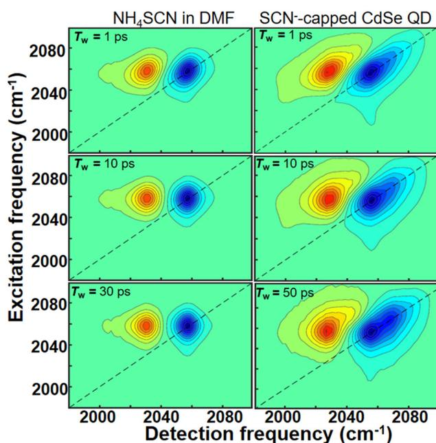
Fig. 3 2D IR spectra of NH<sub>4</sub>SCN (left column) and CdSe-SCN (right column) in DMF at three different waiting times ( $T_w$ ).  $T_w$  increases from the top to the bottom along each column.
