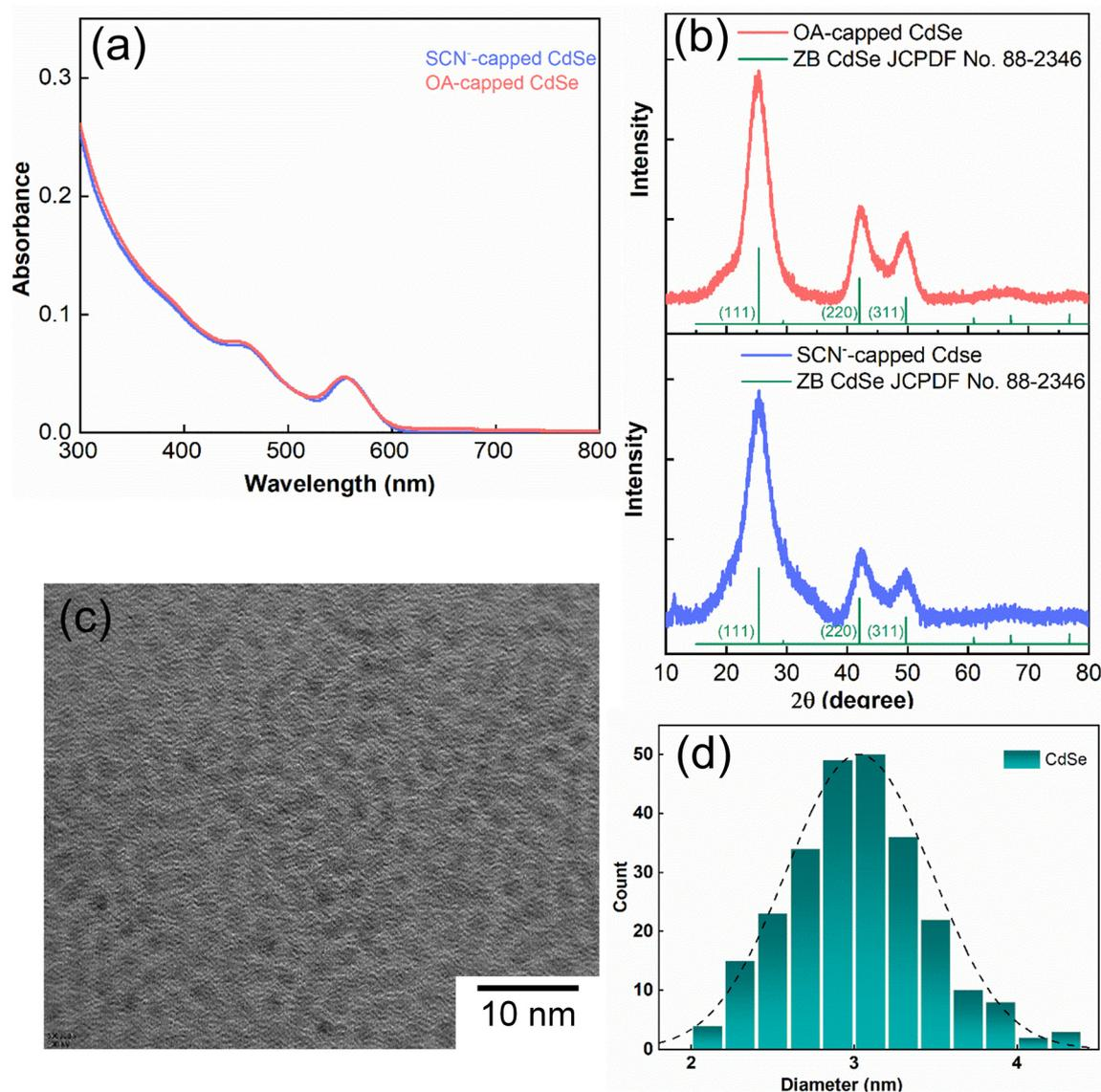
**Fig. 1** (a) UV-vis absorption spectra of oleate-capped CdSe QD colloidal solution in hexane and thiocyanate  $\text{SCN}^-$ -capped CdSe QD colloidal solution in DMF. (b) Diffraction patterns of QDs before and after ligand exchange revealing identical crystallinity. (c) HRTEM image of CdSe QDs before ligand exchange. (d) Particle size distributions with peaks at around  $\sim 3$  nm are obtained from the HRTEM analysis of CdSe QDs.
