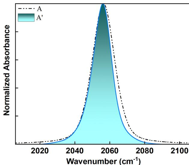
**Fig. 5** The  $\text{C}\equiv\text{N}$  stretching peak of free  $\text{SCN}^-$  in the absence of CdSe QDs (peak A') has been overlaid with the Gaussian fit of the peak at  $2056\text{ cm}^{-1}$  in the presence of QDs (peak A). The two spectra overlap well on the low-frequency side. In the presence of QDs, the Gaussian fit shows a broadening on the high-frequency side.
