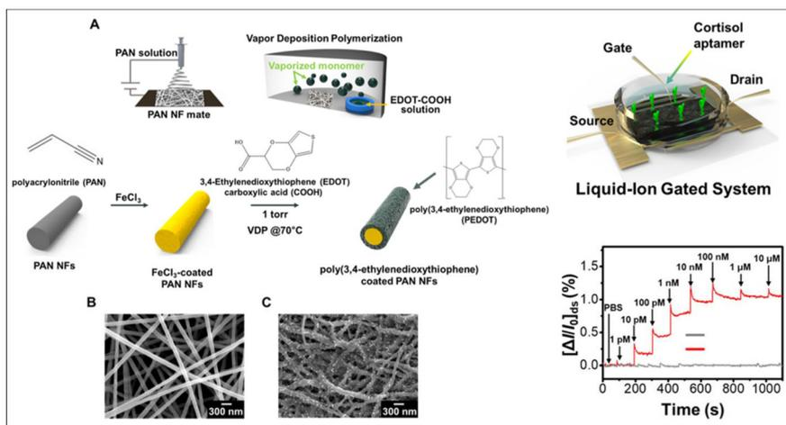
**Fig. 16** Overview of the detection of different metabolites using PEDOT-derived nano-biosensors (continued). (A) Cortisol aptasensor design through polyacrylonitrile (PAN-NF) by electrospinning method followed by modification with carboxylated PEDOT through vapor deposition. SEM images of the (B) pristine PAN template and (C) polymerized PEDOT coated on the PAN NF surface. Adapted from ref. 143 with permission. Copyright 2022, ACS.
