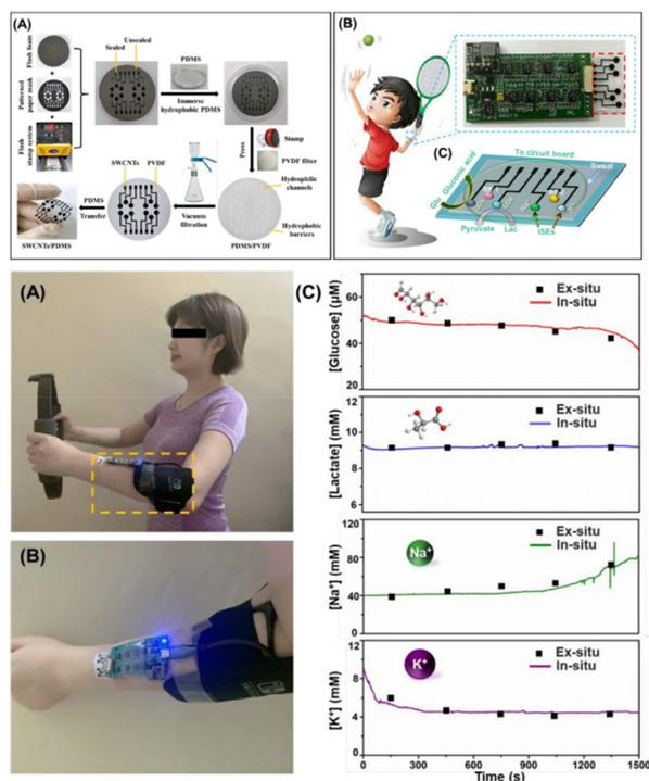
**Fig. 13** Different PEDOT nano-biosensors developed for the detection of lactate. Flexible electrode array consists of SWCNT material, Pt nanoparticles and PEDOT layers. Schematic illustration of PS-inspired flexible sensor array design, signal acquisition system (A)-(C) top images) and real-time monitoring of sweat markers in a non-invasive way (A)-(C) bottom images). Adapted from ref. 136 with permission. Copyright 2022, ACS.
