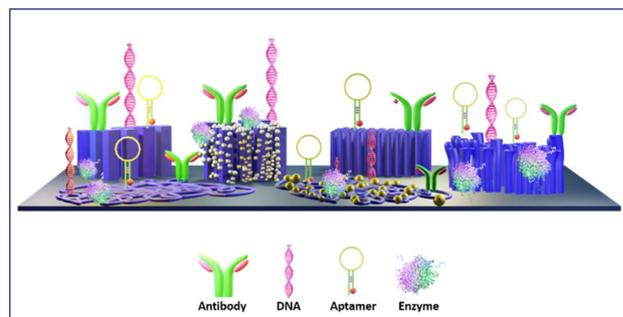
**Scheme 3** Design strategy of PEDOT/PProDOT nano-biosensors. Diverse nanostructures of PEDOT/PProDOT derivatives and nano-composites deposited on the electrode platform. Sensor probes such as antibody, aptamers, DNA, and enzymes for specific target recognition can be conjugated on polymeric nano-surfaces through different coupling chemistry.
