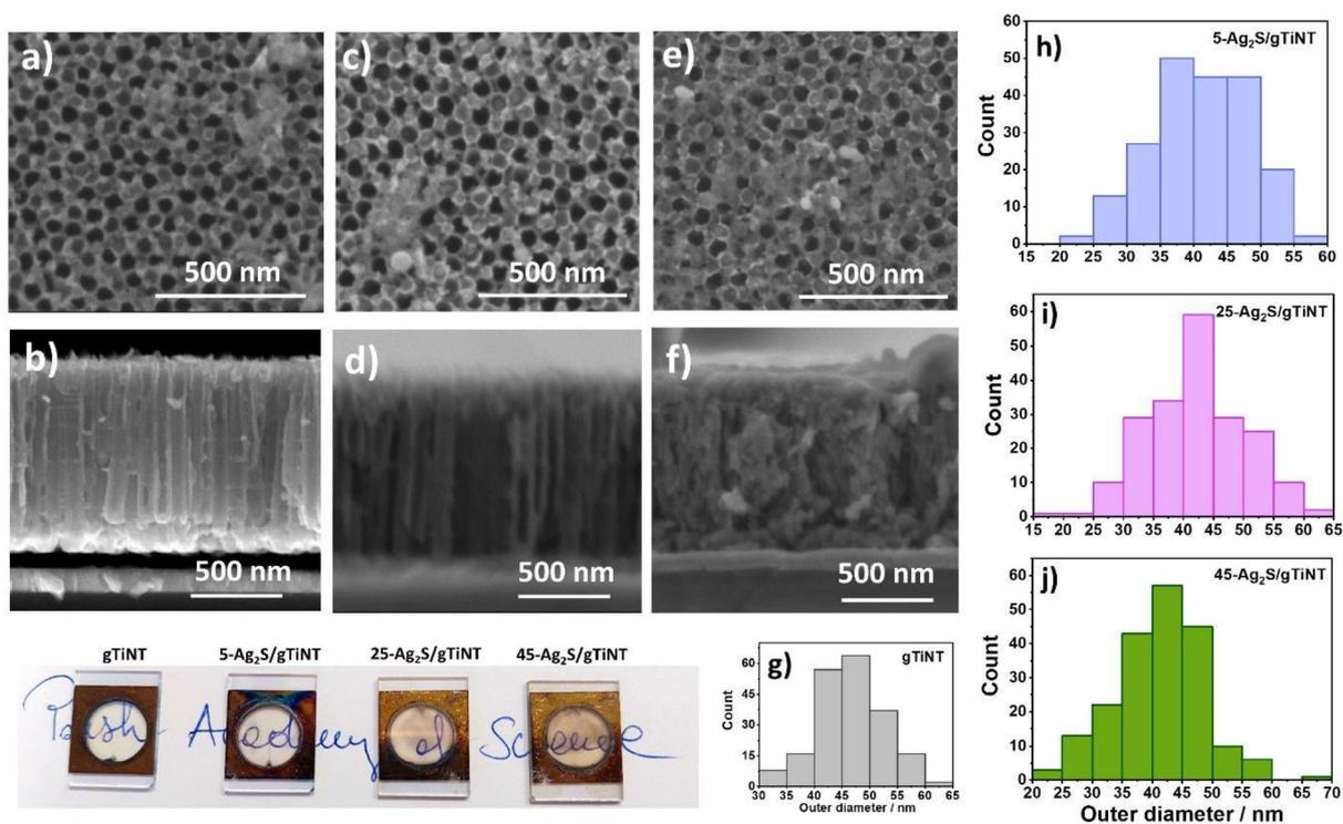
Fig. 3 SEM images of (a and b) 5-Ag<sub>2</sub>S/gTiNT, (c and d) 25-Ag<sub>2</sub>S/gTiNT, (e and f) 45-Ag<sub>2</sub>S/gTiNT, and size distribution of TiO<sub>2</sub> nanotubes outer diameter (g) gTiNT, (h) 5-Ag<sub>2</sub>S/gTiNT, (i) 25-Ag<sub>2</sub>S/gTiNT, (j) 45-Ag<sub>2</sub>S/gTiNT.
