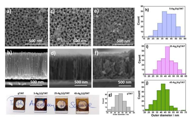
Fig. 3 SEM images of (a and b) 5-Ag<sub>2</sub>S/gTiNT, (c and d) 25-Ag<sub>2</sub>S/gTiNT, (e and f) 45-Ag<sub>2</sub>S/gTiNT, and size distribution of TiO<sub>2</sub> nanotubes outer diameter (g) gTiNT, (h) 5-Ag<sub>2</sub>S/gTiNT, (i) 25-Ag<sub>2</sub>S/gTiNT, (j) 45-Ag<sub>2</sub>S/gTiNT.
