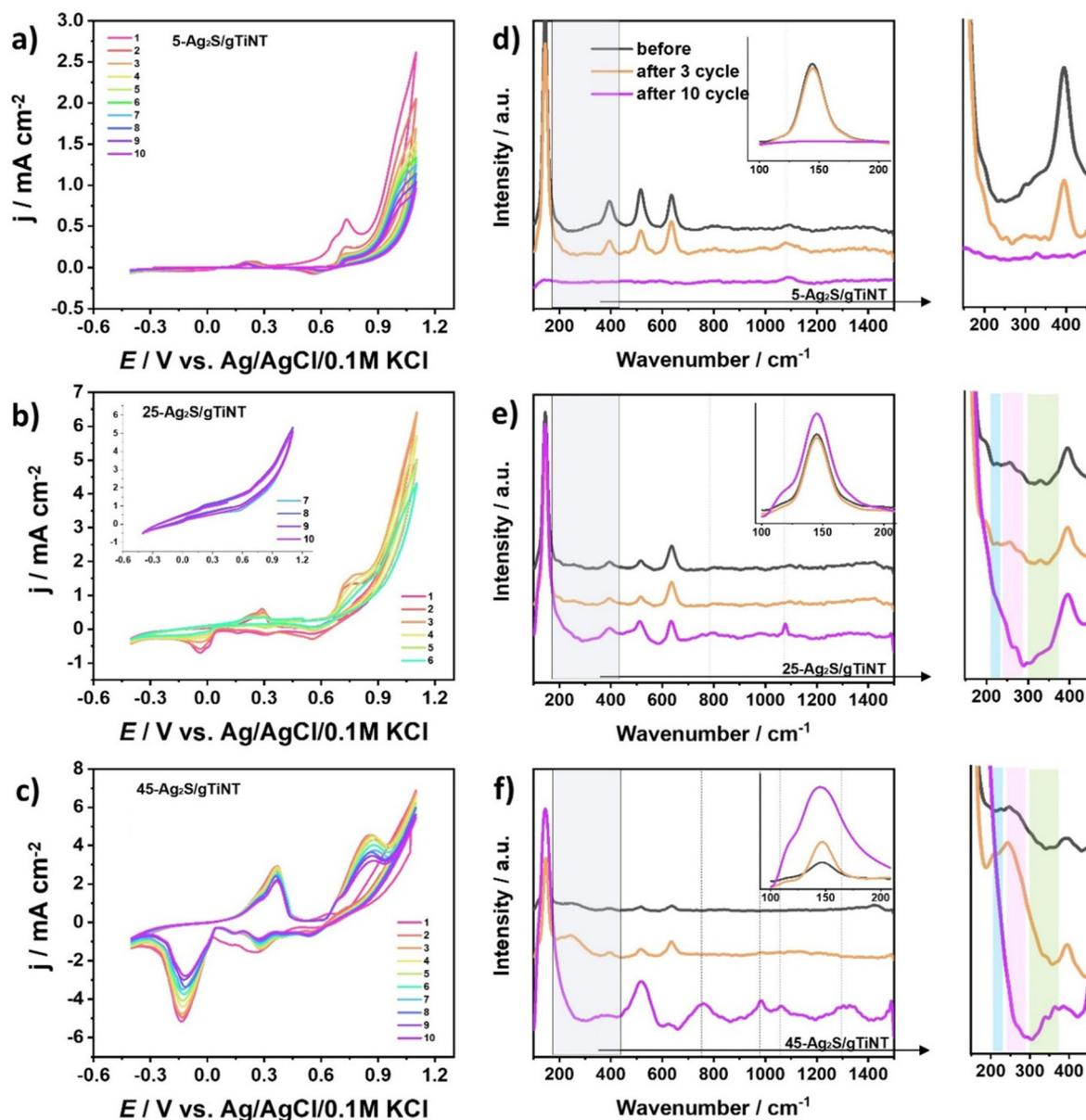
Fig. 9 Cyclic voltammograms of (a) 5- $\text{Ag}_2\text{S}/\text{gTiNT}$ , (b) 25- $\text{Ag}_2\text{S}/\text{gTiNT}$ , (c) 45- $\text{Ag}_2\text{S}/\text{gTiNT}$  and Raman spectra before CVs and after 3 or 10 CVs cycles for (d) 5- $\text{Ag}_2\text{S}/\text{gTiNT}$ , (e) 25- $\text{Ag}_2\text{S}/\text{gTiNT}$ , (f) 45- $\text{Ag}_2\text{S}/\text{gTiNT}$  in 0.5 M NaOH electrolyte (scan rate  $50 \text{ mV s}^{-1}$ ). All the graphs on the right are insets of the Raman graphs.
