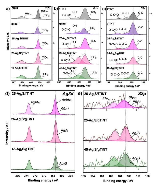
Fig. 5 XPS high resolution spectra registered for the fTiNT, gTiNT, 25-Ag<sub>2</sub>S/fTiNT, 25-Ag<sub>2</sub>S/gTiNT, 45-Ag<sub>2</sub>S/gTiNT (a) Ti 2p, (b) O 1s, (c) C 1s, (d) Ag 3d, (e) S 2p.
