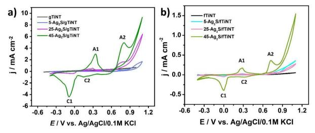
Fig. 8 Cyclic voltammetry curves for (a) Ag<sub>2</sub>S-coated and non-coated gTiNT and (b) Ag<sub>2</sub>S-coated and non-coated fTiNT in 0.5 M NaOH electrolyte (scan rate 50 mV s<sup>-1</sup>).
