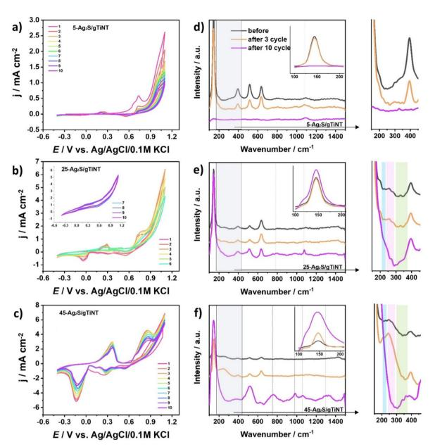
Fig. 9 Cyclic voltammetry curves of (a)  $5-Ag_2S/gTiNT$ , (b)  $25-Ag_2S/gTiNT$ , (c)  $45-Ag_2S/gTiNT$  and Raman spectra before CVs and after 3 or 10 CVs cycles for (d)  $5-Ag_2S/gTiNT$ , (e)  $25-Ag_2S/gTiNT$ , (f)  $45-Ag_2S/gTiNT$  in 0.5 M NaOH electrolyte (scan rate 50 mV s<sup>-1</sup>). All the graphs on the right are insets of the Raman graphs.
