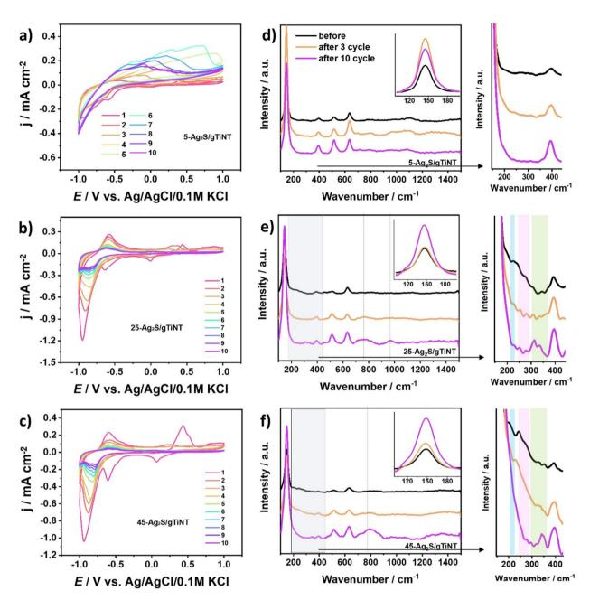
Fig. 7 Cyclic voltammetry curves of (a)  $5-Ag_2S/gTiNT$ , (b)  $25-Ag_2S/gTiNT$ , (c)  $45-Ag_2S/gTiNT$  and Raman spectra before CVs and after 3 or 10 CVs cycles for (d)  $5-Ag_2S/gTiNT$ , (e)  $25-Ag_2S/gTiNT$ , (f)  $45-Ag_2S/gTiNT$  in 0.5 M  $Na_2SO_4$  electrolyte (scan rate 50 mV s<sup>-1</sup>). All the graphs on the right are insets of the Raman graphs.
