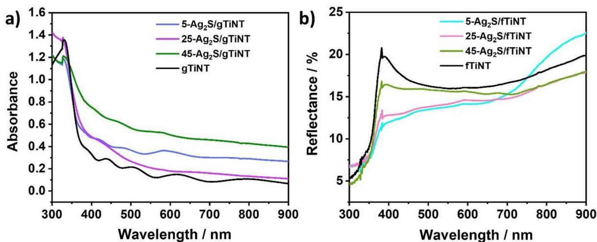
Fig. 4 UV-vis (a) absorbance spectra for Ag<sub>2</sub>S-coated and non-coated gTiNT and (b) reflectance spectra for Ag<sub>2</sub>S-coated and non-coated fTiNT.
