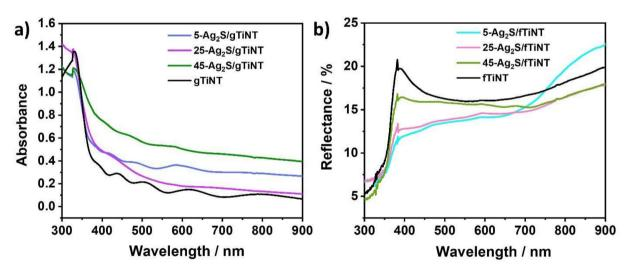
Fig. 4 UV-vis (a) absorbance spectra for Ag<sub>2</sub>S-coated and non-coated gTiNT and (b) reflectance spectra for Ag<sub>2</sub>S-coated and non-coated fTiNT.
