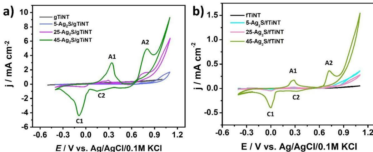
Fig. 8 Cyclic voltammetry curves for (a)  $\text{Ag}_2\text{S}$ -coated and non-coated gTiNT and (b)  $\text{Ag}_2\text{S}$ -coated and non-coated fTiNT in 0.5 M NaOH electrolyte (scan rate  $50 \text{ mV s}^{-1}$ ).
