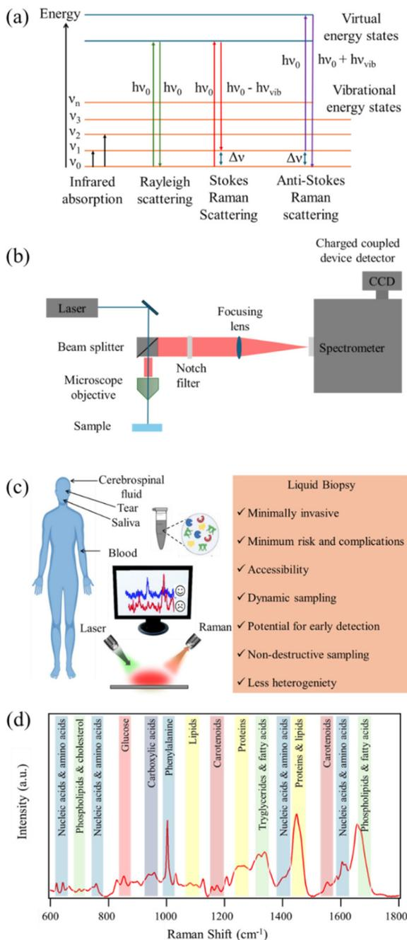
**Fig. 1** (a) Schematic representation of the energy level diagram of Raman scattering process. (b) Generic setup for a Raman microspectroscopy system. (c) Illustrative diagram depicting the use of RS in analyzing liquid biopsy for the detection and diagnosis of brain disorders. (d) Raman spectra of human serum from a healthy donor highlighting the peak assignment for various metabolic groups and biomolecules.
