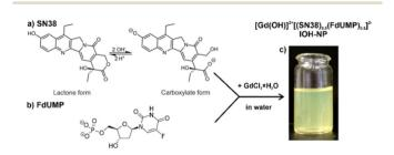
illustrating the aqueous synthesis Fig. 1 Scheme  $(OH)]^{2+}[(SN-38)_{0.5}(FdUMP)_{0.5}]^{2-}$  IOH-NPs with SN-38 (a) and FdUMP (b) as drug anions as well as a photo of the resulting aqueous suspension
