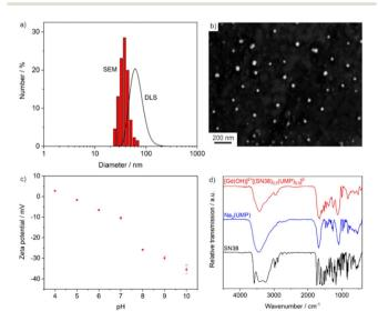
**Fig. 2** Particle features of  $[Gd(OH)]^{2+}[(SN-38)_{0.5}(FdUMP)_{0.5}]^{2-}$  IOH-NPs: (a) size and size distribution according to DLS (in water) and SEM; (b) SEM overview image; (c) zeta potential of aqueous suspension; (d) FT-IR spectra (Na<sub>2</sub>(UMP) and SN-38 as references).
