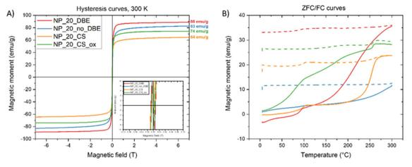
Fig. 4 (A) Magnetization curves (insert: zoom between -0.1 and 0.1 T) and (B) ZFC/FC curve of four types of IONPs
