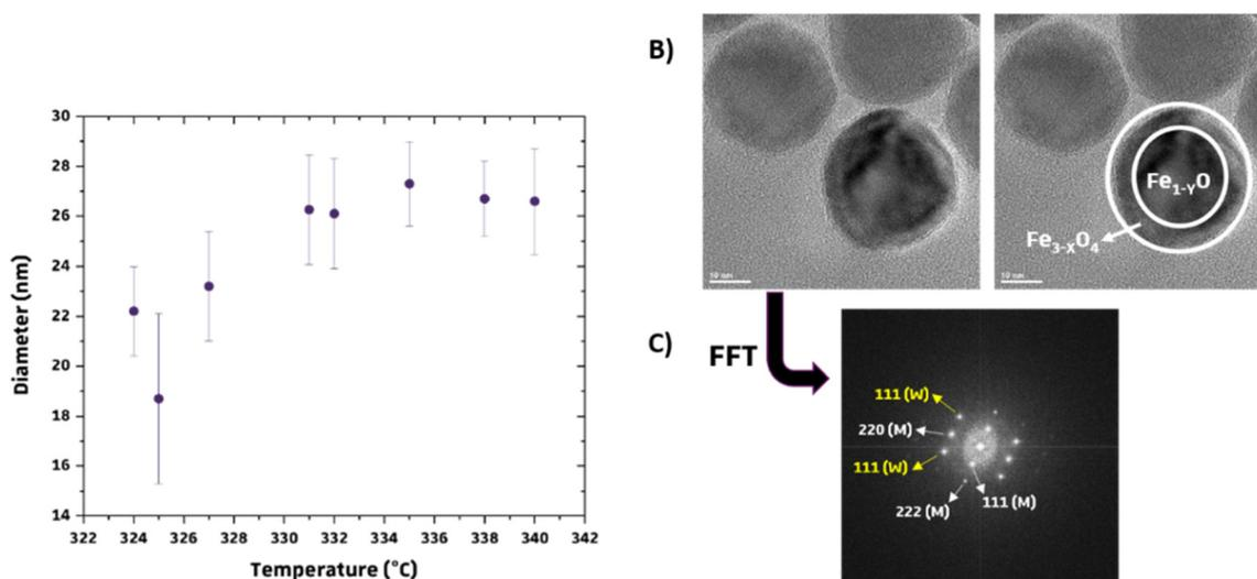
Fig. 2 (A) Mean diameter of IONPs synthesized using protocol P20\_2 as a function of the reaction temperature, (B) HRTEM images of core-shell Fe<sub>1-x</sub>O@Fe<sub>3-x</sub>O<sub>4</sub> IONPs and (C) its corresponding FFT pattern with plane indication (W = wüstite plane, M = magnetite plane) (A).
