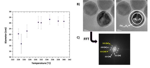
Fig. 2 (A) Mean diameter of IONPs synthesized using protocol P20\_2 as a function of the reaction temperature, (B) HRTEM images of core-shell  $Fe_{1-X}O@Fe_{3-X}O_4$  IONPs and (C) its corresponding FFT pattern with plane indication (W = wüstite plane, M = magnetite plane) (A).
