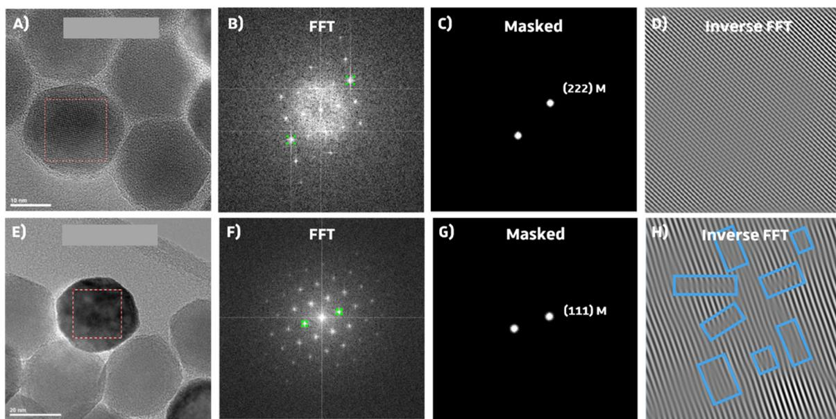
**Fig. 3** Upper row corresponds to IONPs synthesized with protocol P20\_2 and the lower row corresponds to IONPs synthesized with protocol P20\_3\_no\_DBE. (A) and (E) High resolution TEM images of IONPs, (B) and (F) the corresponding FFT images, (C) and (G) applied masked on two reflections plans, and (D) and (H) inverse FFT to visualize the crystallographic planes and eventual defects. Blue squares show crystallographic defects.
