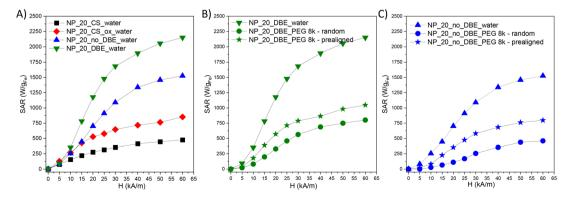
Fig. 5 (A) SAR values for NP\_P20\_DBE, NP\_P20\_no\_DBE, NP\_20\_CS and NP\_20\_CS\_ox suspensions in water and of (B) NP\_20\_DBE and (C) NP\_20\_no\_DBE suspended in water and in a PEG8k matrix, random or prealigned, at a concentration of 1 mg<sub>Fe</sub> mL<sup>-1</sup>.
