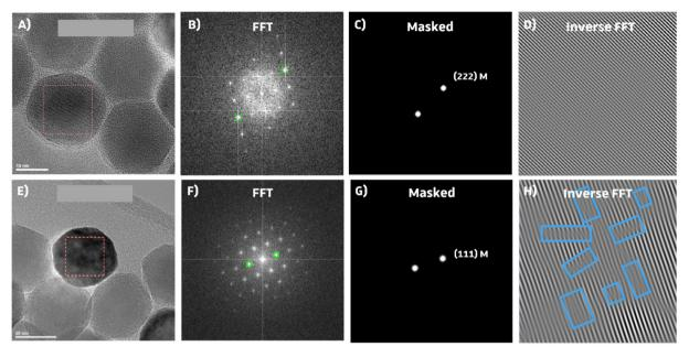
Fig. 3 Upper row corresponds to IONPs synthesized with protocol P20\_2 and the lower row corresponds to IONPs synthesized with protocol P20\_3\_no\_DBE. (A) and (E) High resolution TEM images of IONPs, (B) and (F) the corresponding FFT images, (C) and (G) applied masked on two reflections plans, and (D) and (H) inverse FFT to visualize the crystallographic planes and eventual defects. Blue squares show crystallographic defects
