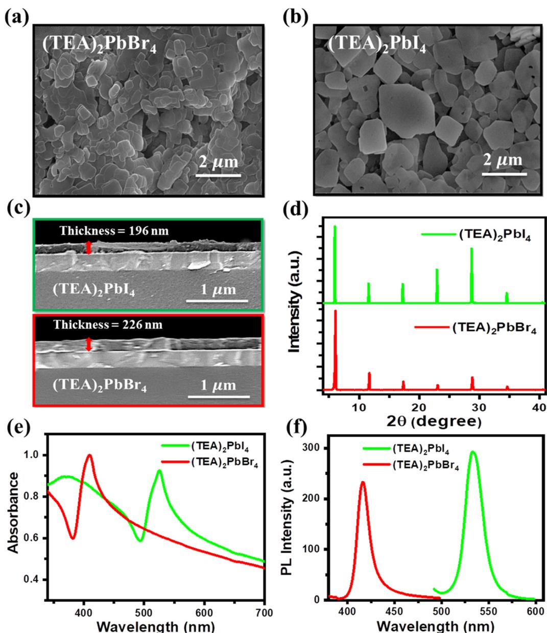
Fig. 1 Top-view SEM images of (a)  $(\text{TEA})_2\text{PbBr}_4$  and (b)  $(\text{TEA})_2\text{PbI}_4$  perovskites. (c) Cross-sectional SEM images, (d) XRD patterns, (e) UV-vis absorption spectra, and (f) PL spectra of  $(\text{TEA})_2\text{PbBr}_4$  and  $(\text{TEA})_2\text{PbI}_4$  perovskite films.
