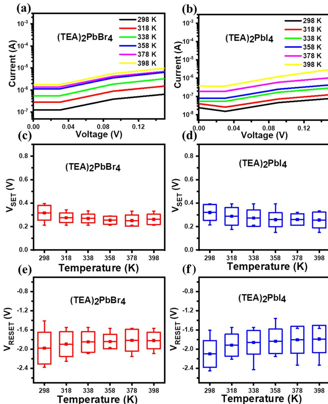
Fig. 5 (a and b) Temperature dependence of the  $I$ - $V$  characteristics of the HRS before the SET process, (c and d) SET, and (e and f) RESET voltage distributions measured at various temperatures for  $(\text{TEA})_2\text{PbBr}_4$  and  $(\text{TEA})_2\text{PbI}_4$  devices.
