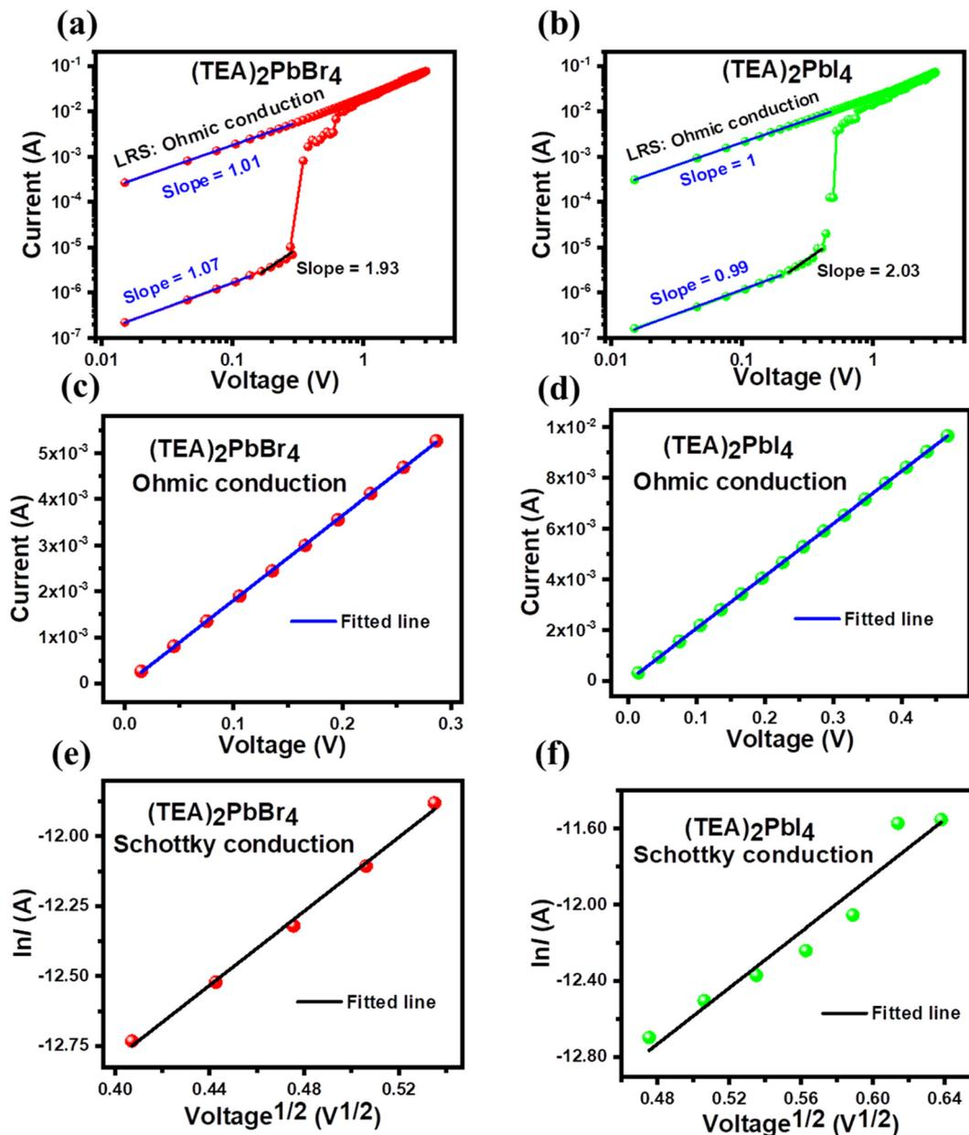
Fig. 4 (a and b) Double-logarithmic plots of  $I$ - $V$  curves, (c and d) proportional relation between  $I$  and  $V$  in LRS, and (e and f)  $\ln I$ - $V^{1/2}$  plots in the HRS for  $(\text{TEA})_2\text{PbBr}_4$  and  $(\text{TEA})_2\text{PbI}_4$  devices. The straight lines are the results of linear fittings.
