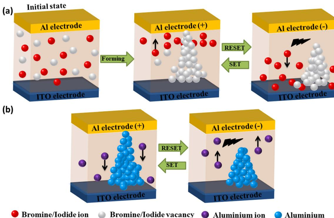
Fig. 6 Diagrams explaining the RS mechanism via formation of a conductive filament of (a) halide anions and (b) electrochemically active metal cations.
