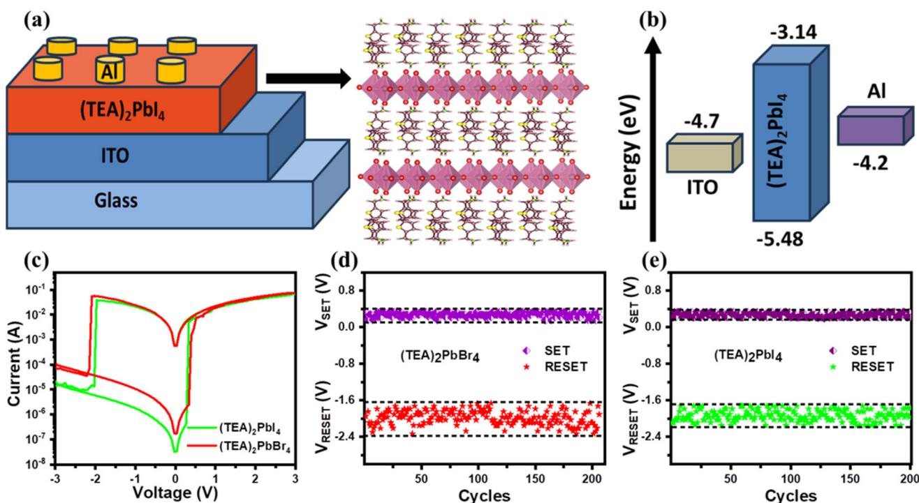
Fig. 2 (a) Schematic illustration of the  $(\text{TEA})_2\text{PbI}_4$  PRM device structure showing the 2D perovskite layer. (b) Band alignment with the energy levels of every component in the device. (c) Typical  $I$ - $V$  curves of  $(\text{TEA})_2\text{PbBr}_4$  and  $(\text{TEA})_2\text{PbI}_4$  PRM devices. Statistically analyzed SET and RESET voltages for 200 cycles of one (d)  $(\text{TEA})_2\text{PbBr}_4$ - and (e)  $(\text{TEA})_2\text{PbI}_4$ -based device.
