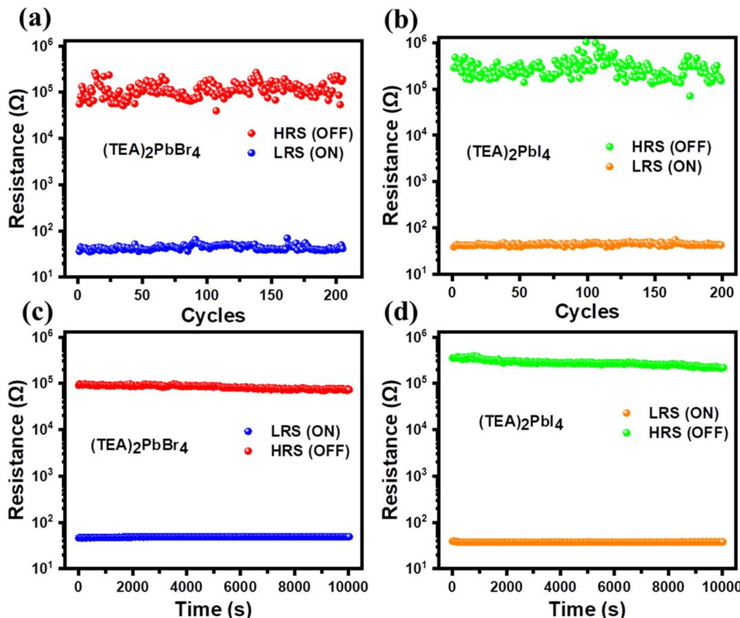
Fig. 3 Endurance characteristics of (a)  $(\text{TEA})_2\text{PbBr}_4$  and (b)  $(\text{TEA})_2\text{PbI}_4$  PRM devices over 200 cycles. Retention properties of the ON and OFF states for (c)  $(\text{TEA})_2\text{PbBr}_4$  and (d)  $(\text{TEA})_2\text{PbI}_4$  cells.
