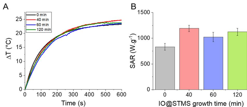
Fig. 11 (A) Temperature profiles as a function of time for the different IO@STMS- $t$  NPs at  $0.5 \text{ mgFe mL}^{-1}$  under NIR light irradiation. (B) Corresponding SAR values. These results were obtained with the IO@STMS- $t$  obtained from series 2.
