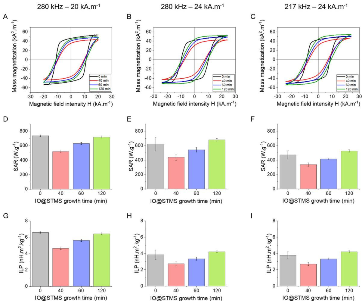
**Fig. 10** (A)–(C) Representative hysteresis cycles for the different IO@STMS-*t* NPs (IO@STMS-0 and for IO@STMS-*t* (*t* = 40, 60, 120 min)) obtained from series 2 at different frequency–amplitude conditions. (D)–(F) Corresponding SAR values. (G)–(I). Corresponding ILP values.
