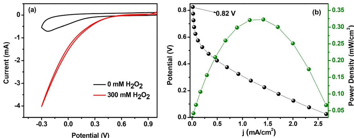
Fig. 7 (a) Current vs. potential plots and (b) the corresponding current density vs. potential/power density plots (with 300 mM H<sub>2</sub>O<sub>2</sub>) for a single compartment peroxide fuel cell with ATO/FTO as the cathode and nickel foam as the anode in 0.05 M H<sub>2</sub>SO<sub>4</sub> electrolyte solution at a scan rate of 10 mV s<sup>-1</sup>.
