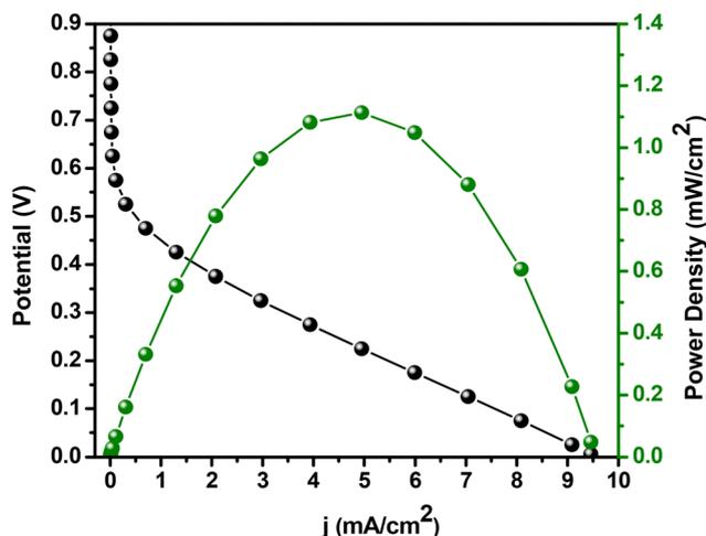
Fig. 8 Current density vs. potential/power density plot for a two-electrode system with an ATO/FTO cathode and a nickel foam anode in 0.05 M H<sub>2</sub>SO<sub>4</sub> electrolyte containing 300 mM H<sub>2</sub>O<sub>2</sub> and 1 M NaCl at a scan rate of 10 mV s<sup>-1</sup>.
