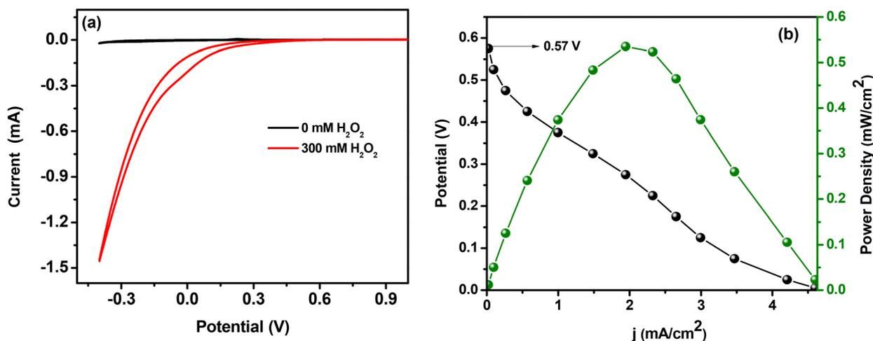
Fig. 5 (a) Short circuit current vs. potential plots and (b) the corresponding current density vs. potential/power density plots (with  $300 \text{ mM H}_2\text{O}_2$ ) for a two-electrode cell with ATO/GCE as the cathode and Ni foam as the anode in  $0.05 \text{ M H}_2\text{SO}_4$  electrolyte solution at a scan rate of  $10 \text{ mV s}^{-1}$ . Currents and powers were normalized to the geometric surface area of the working electrode.
