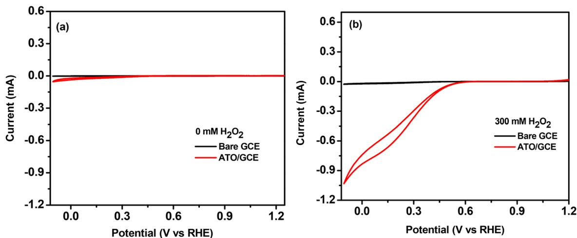
Fig. 4 CV of ATO/GCE and bare GCE (a) without  $\text{H}_2\text{O}_2$  and (b) with 300 mM  $\text{H}_2\text{O}_2$  in 0.05 M  $\text{H}_2\text{SO}_4$  solution at a scan rate of  $10 \text{ mV s}^{-1}$  using Ag/AgCl and platinum wire as reference and counter electrodes, respectively.
