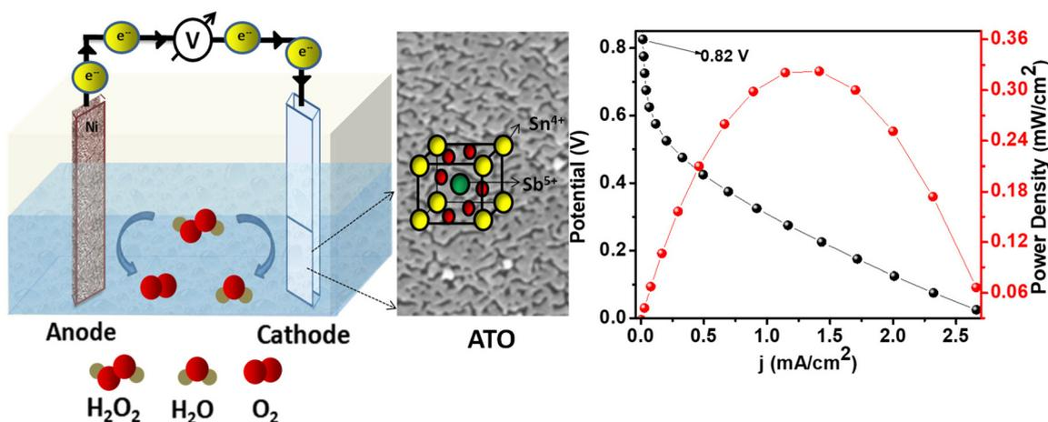
**Scheme 1** Schematic representation of the single-compartment  $\text{H}_2\text{O}_2$  fuel cell along with the obtained current density vs. potential/power density plots. The fuel cell is developed with antimony doped tin oxide (ATO) coated on FTO as the cathode and Ni foam as the anode.
