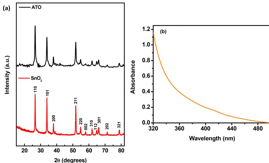
Fig. 3 (a) Powder XRD patterns of undoped  $\text{SnO}_2$  (red, lower panel) and 6 mol% Sb doped  $\text{SnO}_2$  (ATO) nanopowder (black, upper panel) samples and (b) the UV-visible absorption spectrum of the prepared ATO coated FTO electrode.
