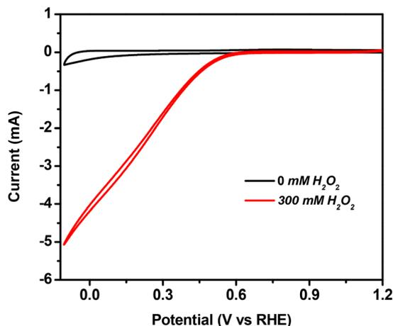
Fig. 6 CV of the ATO/FTO electrode without and with 300 mM  $\text{H}_2\text{O}_2$  in 0.05 M  $\text{H}_2\text{SO}_4$  at a scan rate of  $10 \text{ mV s}^{-1}$  with Ag/AgCl and platinum wire as reference and counter electrodes, respectively.
