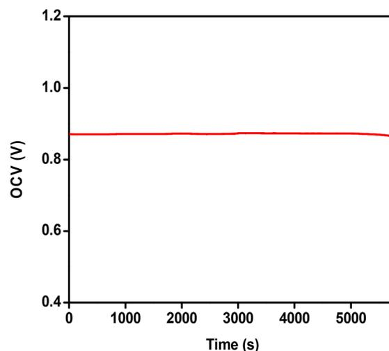
Fig. 9 Open circuit voltage (OCV) recorded as a function of time for a two-electrode cell with ATO/FTO as the cathode and Ni foam as the anode in 0.05 M H<sub>2</sub>SO<sub>4</sub> electrolyte solution at a scan rate of 10 mV s<sup>-1</sup> with 300 mM H<sub>2</sub>O<sub>2</sub>.
