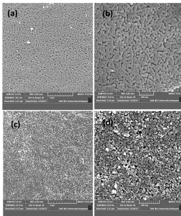
**Fig. 1** Field emission scanning electron microscopy images of ATO nanopowder (a and b) and ATO coated FTO slides (c and d). Scale bars are  $1 \text{ } \mu\text{m}$ ,  $200 \text{ nm}$ ,  $2 \text{ } \mu\text{m}$  and  $500 \text{ nm}$  in a, b, c, and d respectively.
