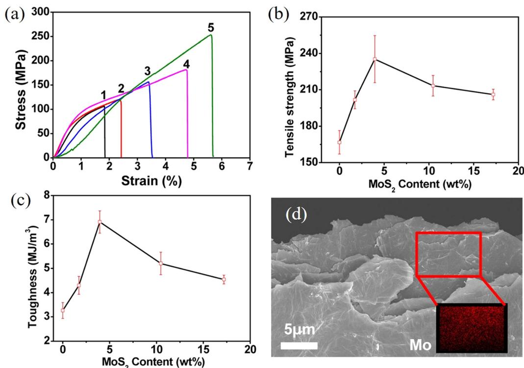
**Fig. 32** (a) Stress–strain curves of GO/ $\text{MoS}_2$ /TPU nanocomposites. 1 to 5 represent GO film, GO/TPU, rGO/TPU, GO/ $\text{MoS}_2$ /TPU, and rGO/ $\text{MoS}_2$ /TPU composites, respectively. Dependence of the (b) tensile strength and (c) toughness of the composites with the loading of  $\text{MoS}_2$ . (d) Fracture surface of the rGO/ $\text{MoS}_2$ /TPU composites. Reproduced with permission from ref. 317. Copyright 2015 American Chemical Society.
