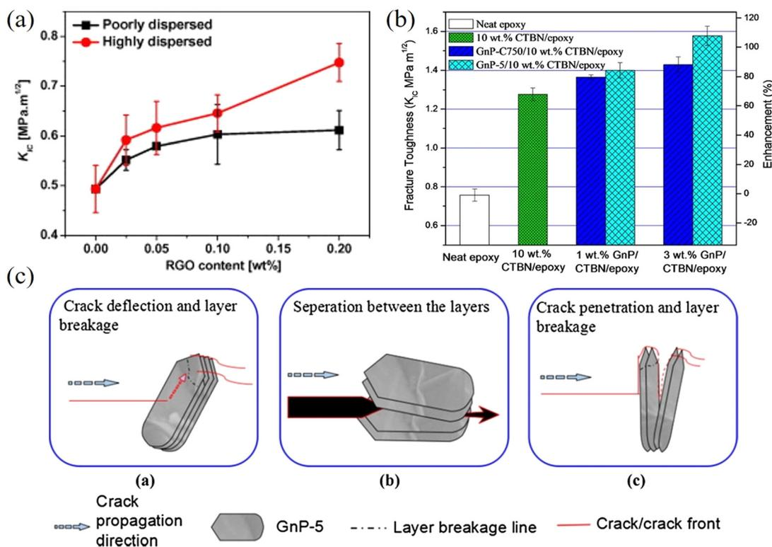
**Fig. 22** (a) Variations of  $K_{IC}$  of rGO/epoxy nanocomposites with rGO loading. Reproduced with permission from ref. 178. Copyright 2013 Elsevier. (b) Effects of CTBN and GNP on the fracture toughness of epoxy composites. (c) Crack propagation in GnP-5 flakes. Reproduced with permission from ref. 179. Copyright 2016 Elsevier.
