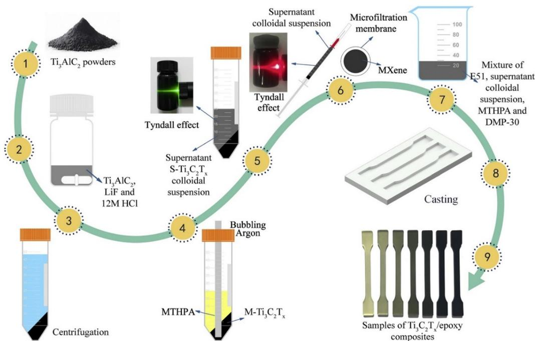
**Fig. 28** Preparation process of Ti<sub>3</sub>C<sub>2</sub>T<sub>x</sub>/epoxy nanocomposites. Reproduced with permission from ref. 262. Copyright 2020 Elsevier.
