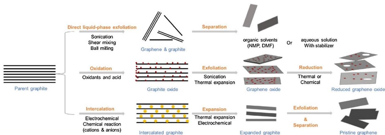
**Fig. 2** Liquid exfoliation methods for the preparation of graphene and related 2D nanosheets, including mechanical force-assisted, oxidation-assisted and intercalation-assisted exfoliation. Reproduced with permission from ref. 11. Copyright 2018 Elsevier.
