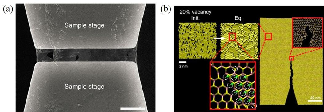
**Fig. 4** (a) Suspended monolayer graphene over a tension stage for fracture toughness measurement. Scale bar, 5  $\mu\text{m}$ . Reproduced with permission from ref. 81. Copyright 2014 Nature Publishing Group. (b) Crack propagation in monolayer  $\text{MoS}_2$  with line defects. Reproduced with permission from ref. 82. Copyright 2016 American Chemical Society.
