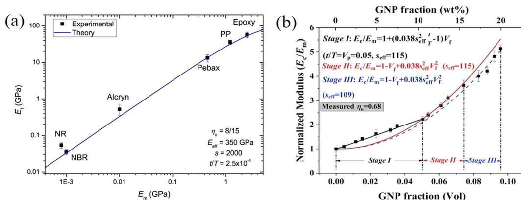
**Fig. 19** (a) Variation of the modulus of graphene nanoplatelets (GNPs) with the modulus of the matrices (dots: experiment data; blue line: theory predictions from eqn (16) and (19)). Reproduced with permission from ref. 171. Copyright 2018 Elsevier. (b) Three stages for the reinforcement of GNPs on elastomers. Reproduced with permission from ref. 153. Copyright 2019 Elsevier.
