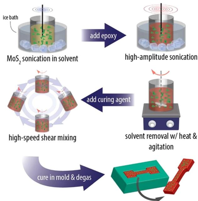
Fig. 13 Solution casting method for the preparation of MoS<sub>2</sub>/epoxy composites. Reproduced with permission from ref. 143. Copyright 2014 American Chemical Society.
