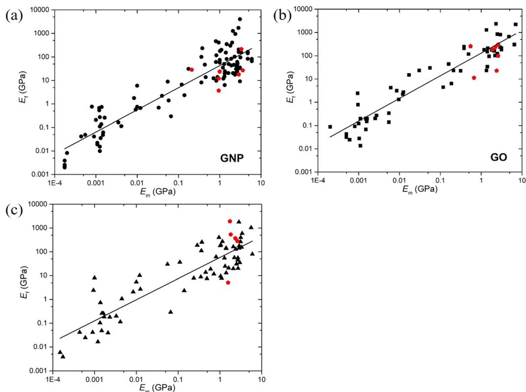
**Fig. 21** Variations of the Young's modulus of (a) GNP, (b) GO and (c) rGO with the modulus of matrices. The red dots correspond to new data published after 2017 and provide an update to the previous figure presented in ref. 16. Reproduced with permission from ref. 16. Copyright 2017 Elsevier.
