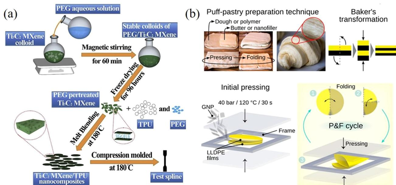
**Fig. 14** (a) Melt mixing method for the preparation of MXene/TPU composites. Reproduced with permission from ref. 149. Copyright 2019 Elsevier. (b) Puff-pastry preparation inspired pressing-and-folding method and illustration of this method for the fabrication of a GNP/LLDPE composite film. Reproduced with permission from ref. 155. Copyright 2018 America Chemical Society.
