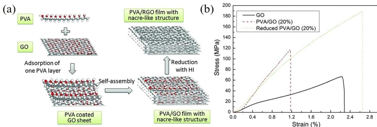
**Fig. 23** (a) Preparation of GO/PVA and rGO/PVA composites with nacre-like structures. (b) Stress-strain curves of GO films, GO/PVA and rGO/PVA composites. Reproduced with permission from ref. 180. Copyright 2012 Wiley-VCH Verlag GmbH & Co. KGaA.
