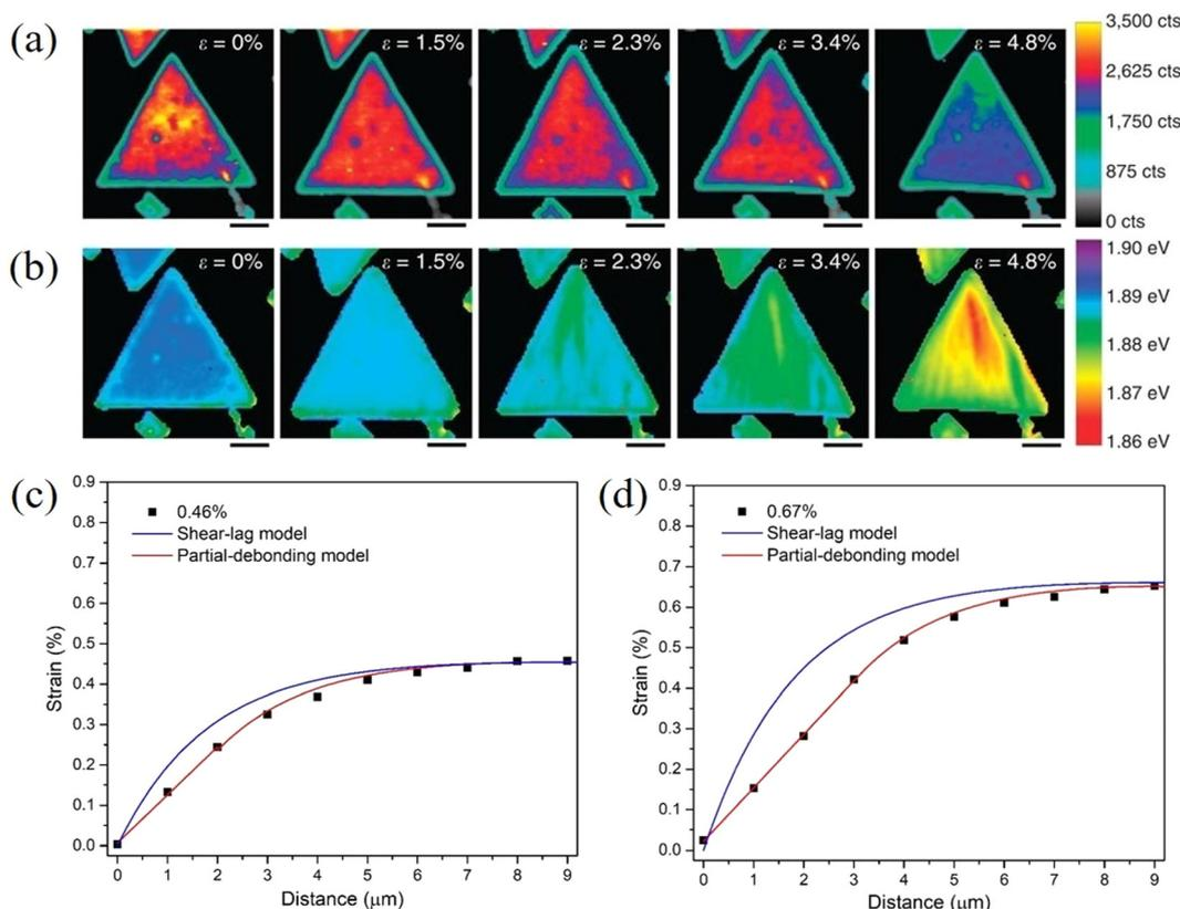
**Fig. 8** PL A exciton (a) intensity and (b) peak mapping of MoS<sub>2</sub> with applied strain increasing from 0 to 4.8%. (Scale bar, 4 μm). Reproduced with permission from ref. 114. Copyright 2014 Nature Publishing Group. Strain distribution in monolayer MoS<sub>2</sub> at (c) 0.46% and (d) 0.67% strain. Both shear-lag model and partial-debonding model were used to fit the experimental results. Reproduced with permission from ref. 115. Copyright 2023 Elsevier.
