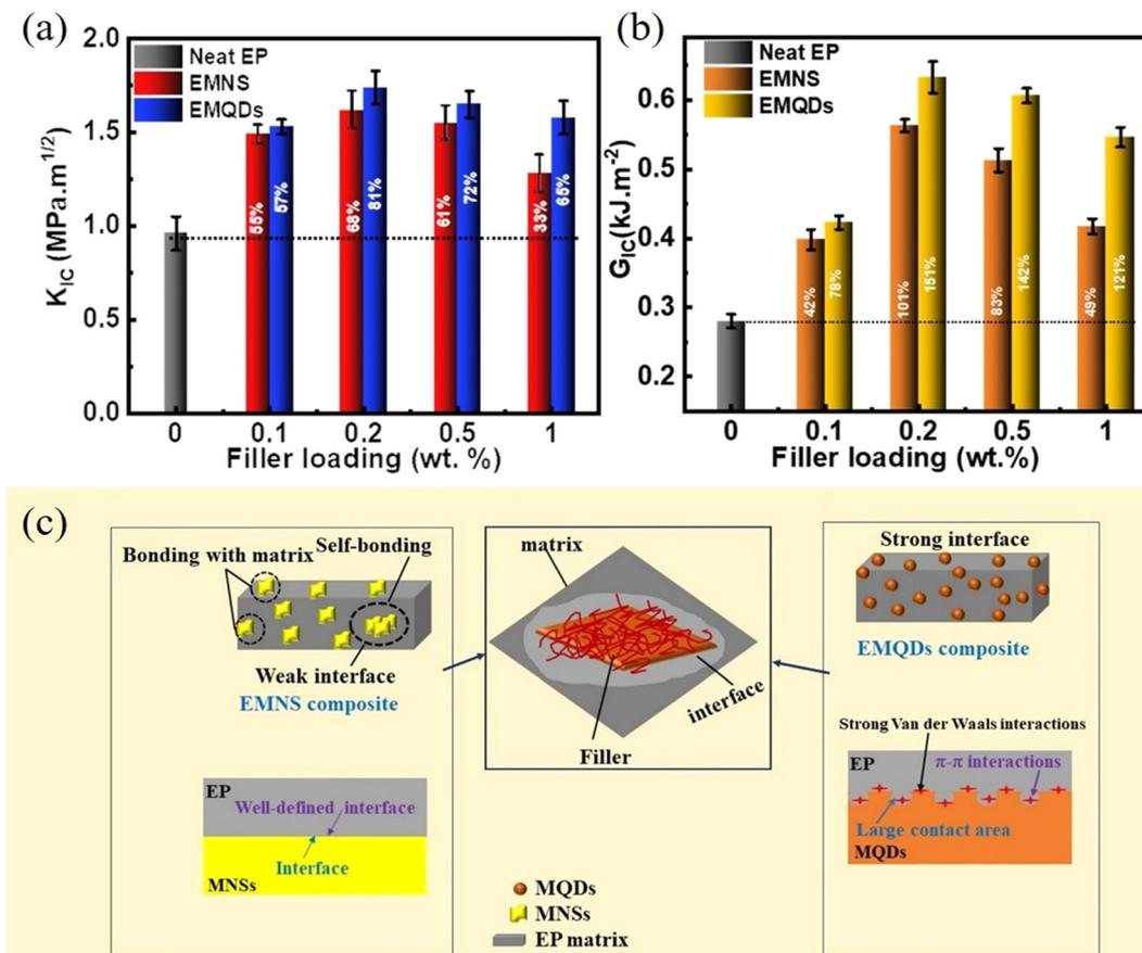
Fig. 26 (a)  $K_{IC}$  and (b)  $G_{IC}$  of neat epoxy, epoxy/MNSs (EMNS) and epoxy/MQDs (EMQDs) nanocomposites. (c) Interfacial interactions of EMNS and EMQDs. Reproduced with permission from ref. 241. Copyright 2021 Elsevier.
