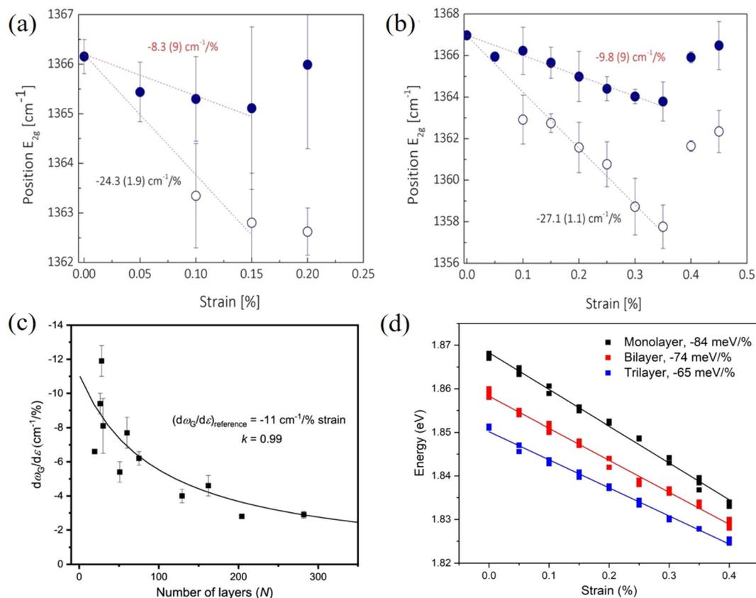
**Fig. 11** Raman G peak shifts of (a) bilayer and (b) four-layer h-BN under uniaxial tension. Reproduced with permission from ref. 100. Copyright 2018 American Physical Society. (c) Raman G band shift rate of h-BN as a function of layer number. Reproduced with permission from ref. 131. Copyright 2021 IOP Publishing Ltd. (d) Evolution of the PL A peak of monolayer, bilayer and trilayer MoS<sub>2</sub> with strain. Reproduced with permission from ref. 115. Copyright 2023 Elsevier.
