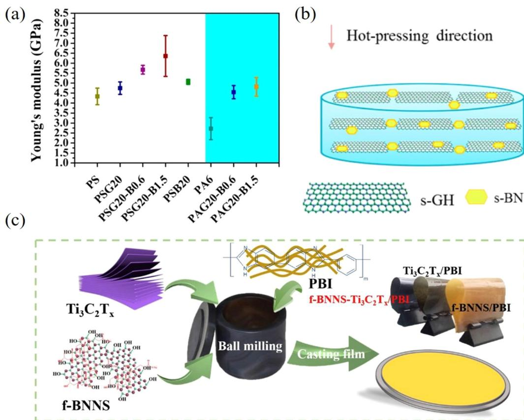
**Fig. 31** (a) Variation of the Young's modulus of PS and PA composites with the addition of graphene and BN. (b) Scheme for the stacking of graphene (s-GH) and BN (s-BN). Reproduced with permission from ref. 311. Copyright 2015 American Chemical Society. (c) Preparation process of PBI-based composite films. Reproduced with permission from ref. 319. Copyright 2019 Elsevier.
