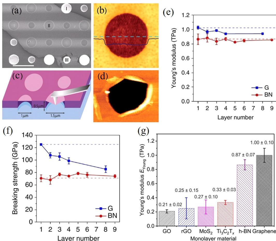
**Fig. 3** (a–d) AFM indentation method for the measurement of stiffness and strength of graphene. Reproduced with permission from ref. 15. Copyright 2008 AAAS. (e and f) Variations of Young's modulus and breaking strength with layer number of graphene (G) and BN. Reproduced with permission from ref. 17 Copyright 2017 Nature Publishing Group. (g) Young's modulus of various 2D materials. Reproduced with permission from ref. 47. Copyright 2018 AAAS.
