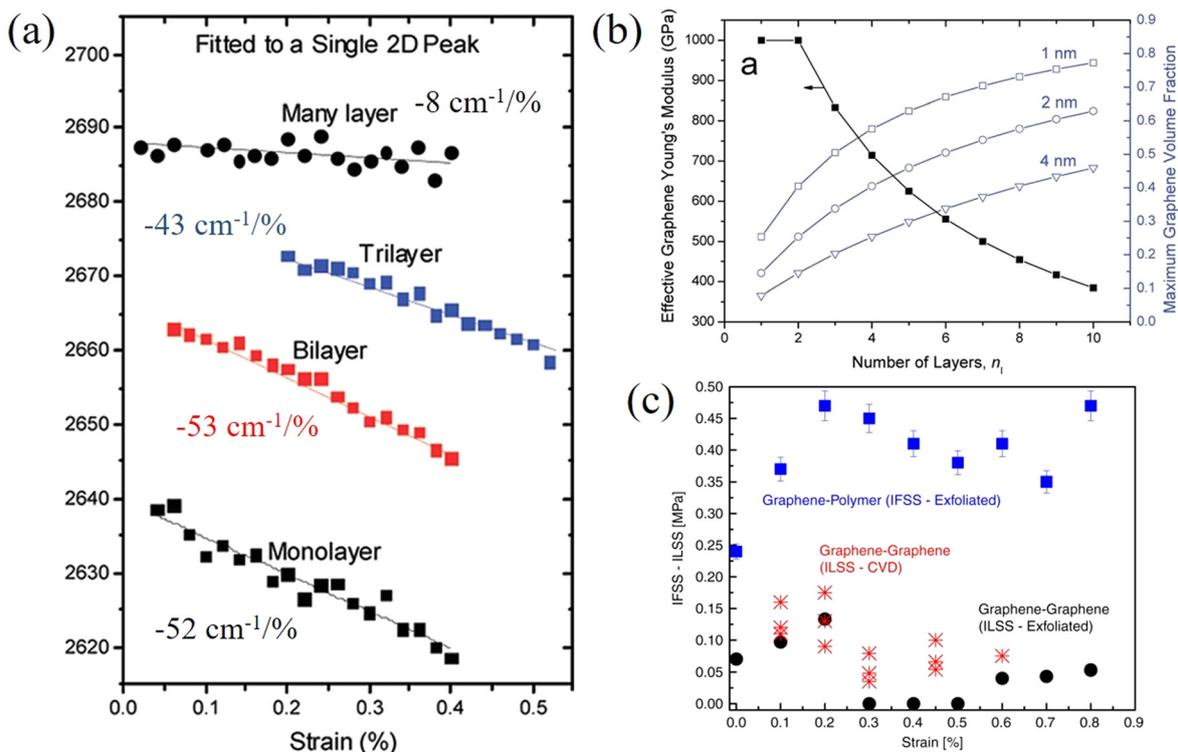
**Fig. 10** (a) Raman 2D shifts of monolayer, bilayer, trilayer and multilayer graphene in a polymer/graphene/polymer model composite. (b) Variations of effective elastic modulus of graphene with layer number. Reproduced with permission from ref. 128. Copyright 2012 American Chemical Society. (c) Interfacial shear stress of graphene-polymer and graphene-graphene. Reproduced with permission from ref. 129. Copyright 2020 Nature Publishing Group.
