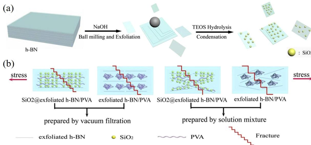
Fig. 35 (a) Preparation of boron nitride nanosheets and SiO<sub>2</sub>@BN hybrids. (b) Fracture behaviour of PVA composites with h-BN and SiO<sub>2</sub>@h-BN prepared by solution casting and vacuum filtration. Reproduced with permission from ref. 384. Copyright 2018 Elsevier.
