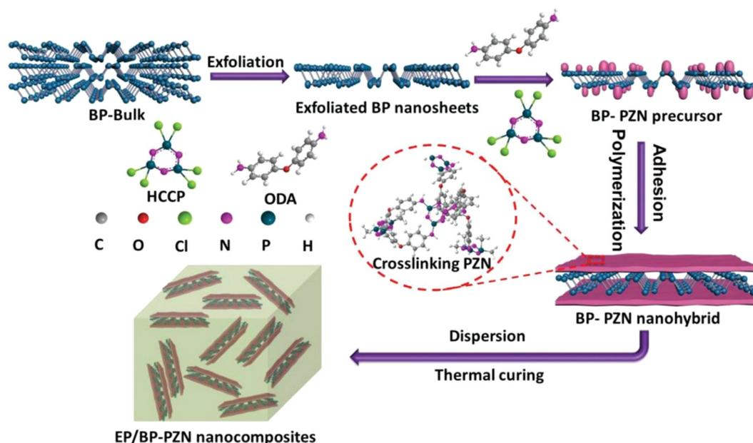
**Fig. 30** Preparation of PZN-functionalized BP nanosheets and BP/epoxy nanocomposites. Reproduced with permission from ref. 289. Copyright 2019 WILEY-VCH Verlag GmbH & Co. KGaA.
