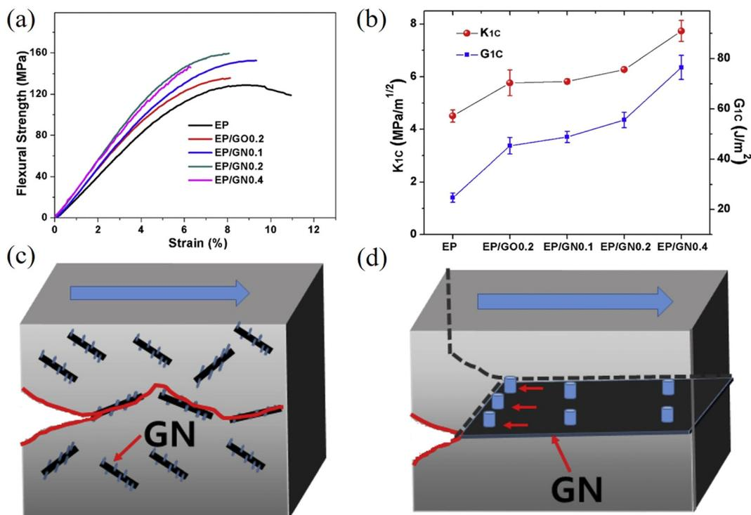
**Fig. 36** (a) Flexural stress–strain curves of epoxy and its nanocomposites. (b) Variation of fracture toughness of epoxy/GO/ND composites with filler content. (c and d) Crack propagation in epoxy/GO/ND composites. Reproduced with permission from ref. 397. Copyright 2017 Elsevier.
