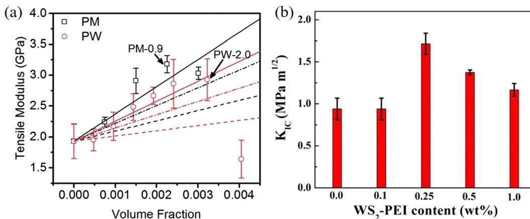
Fig. 27 (a) Tensile modulus for the PVA composites based on MoS<sub>2</sub> (PM) and WS<sub>2</sub> (PW). Reproduced with permission from ref. 245. Copyright 2014 Royal Society of Chemistry. (b) Variation of fracture toughness of WS<sub>2</sub>/epoxy composites with volume fraction. Reproduced with permission from ref. 246. Copyright 2017 American Chemical Society.
