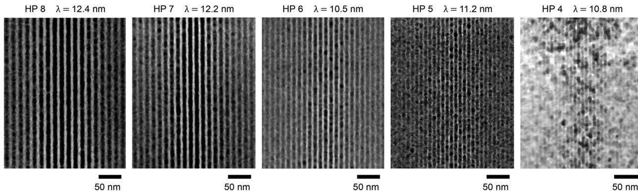
**Fig. 7** MIL exposures at shorter wavelengths. SEM images of HSQ photoresist lines of HP between 4 and 8 nm obtained with wavelengths below 13.5 nm. According to eqn (3), HP depends on the grazing angle  $\alpha$  and the wavelength  $\lambda$ . By tuning the undulator of the beamline, one can set the wavelength so that it gives the desired HP for a given MIL device.
