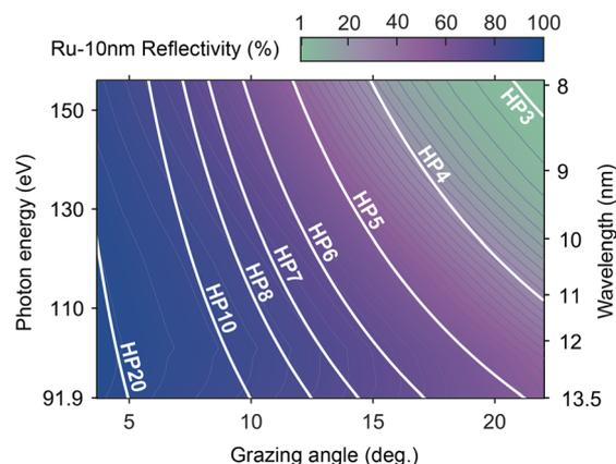
**Fig. 6** MIL at the BEUV spectrum. Calculated reflectivity (%) for a 10 nm Ru film as a function of photon energy and grazing angle.<sup>35</sup> White lines show the combinations of grazing angles and wavelengths that produce the marked HP values.
