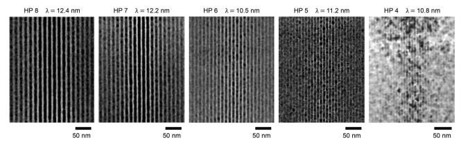
Fig. 7 MIL exposures at shorter wavelengths. SEM images of HSQ photoresist lines of HP between 4 and 8 nm obtained with wavelengths below 13.5 nm. According to eqn (3), HP depends on the grazing angle  $\alpha$  and the wavelength  $\lambda$ . By tuning the undulator of the beamline, one can set the wavelength so that it gives the desired HP for a given MIL device.
