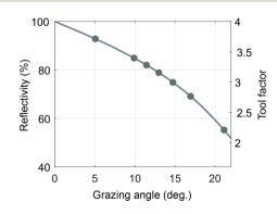
Fig. 3 Mirror reflectivity. Calculated reflectivity as a function of grazing angle for a low-roughness, 10 nm Ru film and a photon energy that corresponds to EUV light with wavelength of 13.5 nm. The markers show the grazing angles of the MIL devices used in this study.
