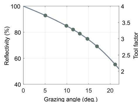
**Fig. 3** Mirror reflectivity. Calculated reflectivity as a function of grazing angle for a low-roughness, 10 nm Ru film and a photon energy that corresponds to EUV light with wavelength of 13.5 nm. The markers show the grazing angles of the MIL devices used in this study.
