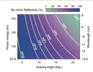
Fig. 6 MIL at the BEUV spectrum. Calculated reflectivity (%) for a 10 nm Ru film as a function of photon energy and grazing angle.<sup>35</sup> White lines show the combinations of grazing angles and wavelengths that produce the marked HP values.
