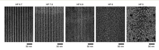
Fig. 4 MIL exposures using the industry standard EUV wavelength of 13.5 nm. SEM images of exposed HSQ photoresist using the MIL devices that are designed for sub-10 nm HP patterning. The HP that is linked to the grazing angle  $\alpha$  (see Fig. 1) is unique for each MIL device at the 13.5 nm wavelength. The imaging area is centered at the maximum-contrast centerline (NILS =  $\pi$ ) and shows the effect of contrast loss away from the centerline.
