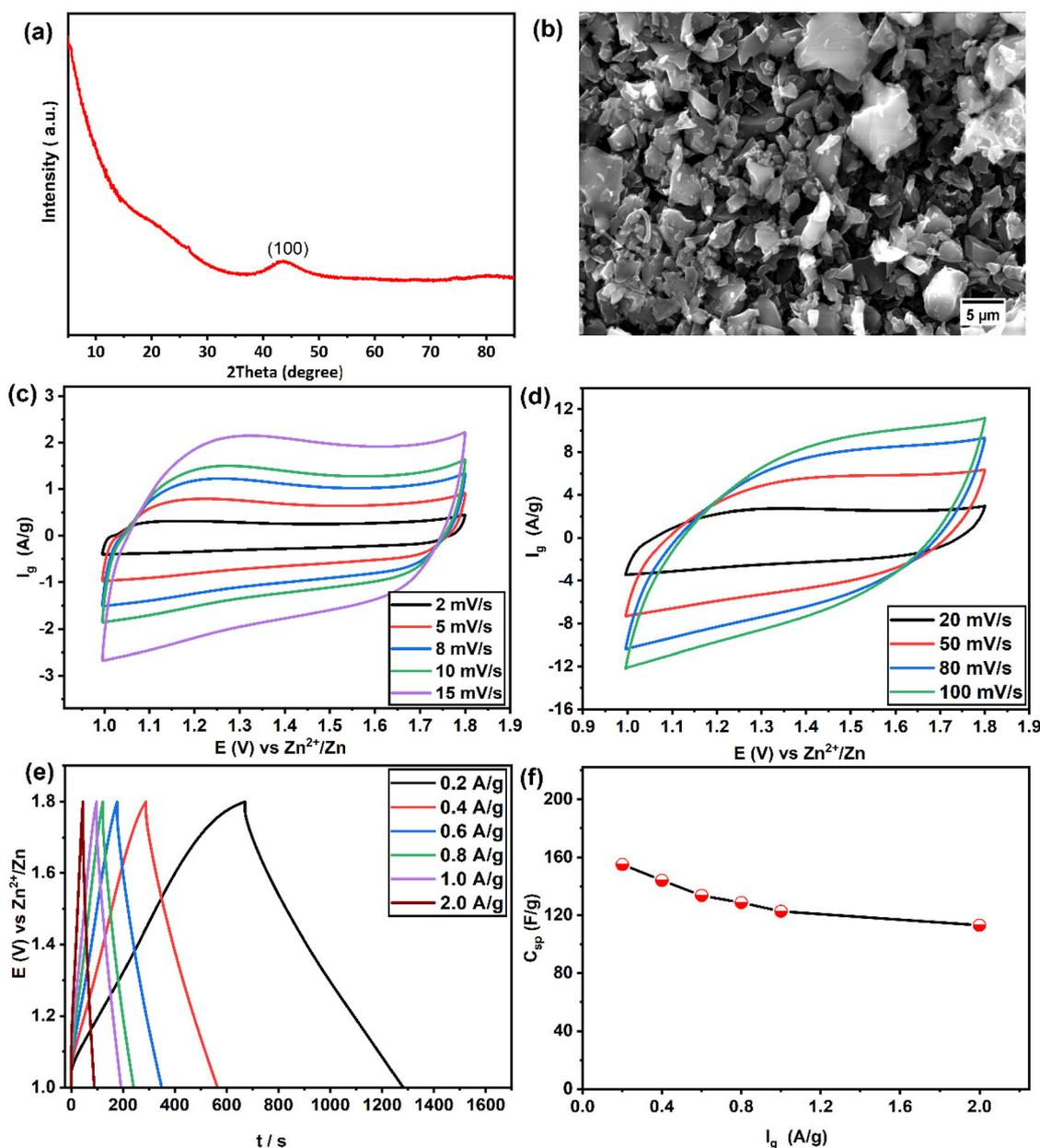
**Fig. 6** Structural characterisation and electrochemical performance of YEC-8A. (a) XRD pattern; (b) SEM image; (c and d) Cyclic voltammograms as a function of scan rate; (e) GCD curves at current densities from 0.2 to 2 A g<sup>-1</sup>; (f) Specific capacitance as a function of current density.
