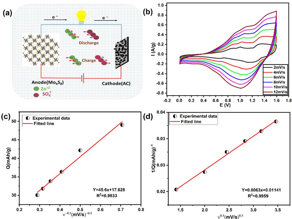
Fig. 7 Schematic and charge storage mechanism of the fabricated energy storage system. (a) Schematic diagram of Mo<sub>6</sub>S<sub>8</sub>/YEC-8A ZIHSC. (b) CVs of Mo<sub>6</sub>S<sub>8</sub>/YEC-8A at different scan rates from 2 to 12 mV s<sup>-1</sup>. Voltammetric charge (*Q*) calculated as a function of scan rate according to Trasatti's method: (c) *Q* vs.  $\nu^{-1/2}$  plot and (d)  $1/Q$  vs.  $\nu^{1/2}$  plot.
