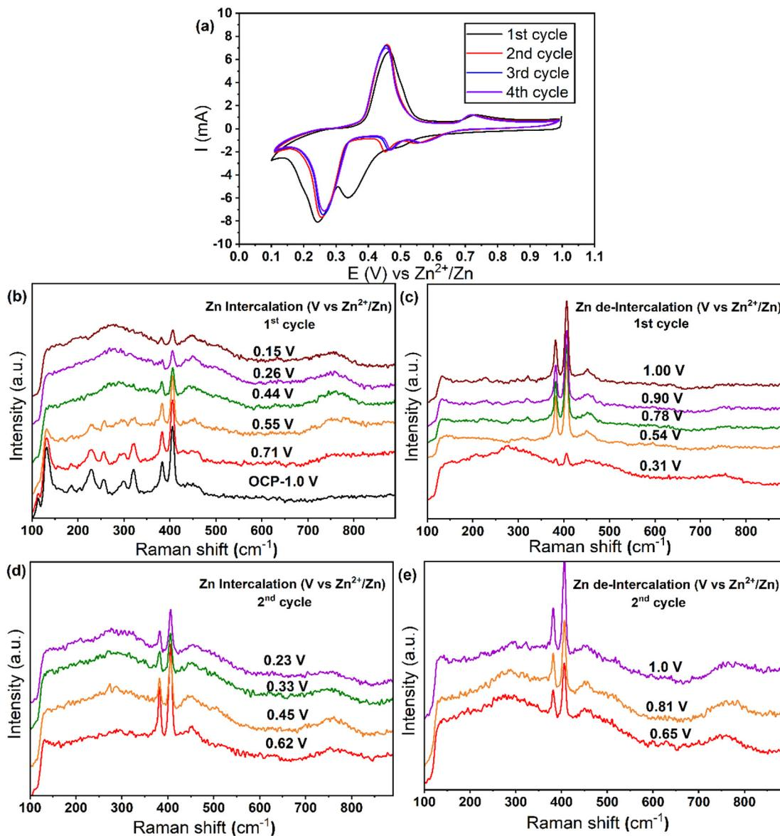
Fig. 4 *In situ* Raman spectra of  $\text{Mo}_6\text{S}_8$  electrode at different charge and discharge potential in 2 M  $\text{ZnSO}_4$ . (a) Cyclic voltammograms of  $\text{Zn}/\text{Mo}_6\text{S}_8$  cell at  $1 \text{ mV s}^{-1}$  during 1<sup>st</sup>, 2<sup>nd</sup>, 3<sup>rd</sup>, and 4<sup>th</sup> cycle: (b, c), and (d, e) Raman spectra of the first and second cycle during the intercalation/de-intercalation process, respectively.
