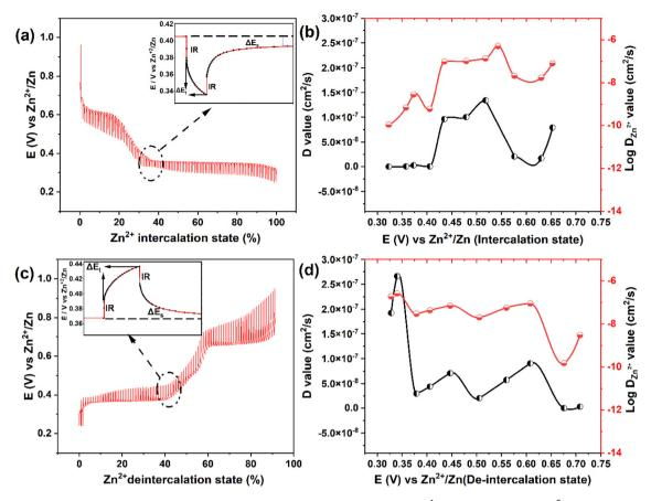
Fig. 5 Galvanostatic intermittent titration technique (GITT) curves of in 2 M ZnSO<sub>4</sub> at 0.1 A g<sup>-1</sup> recorded during the Zn<sup>2+</sup> intercalation (a) and deintercalation process (c) as a function of state of (de)intercalation process. The insets in (a and c) scheme for a single step of a GITT experiment. The corresponding Zn<sup>2+</sup> diffusion coefficients values among the selected steps during intercalation (b) and deintercalation (d) process.
