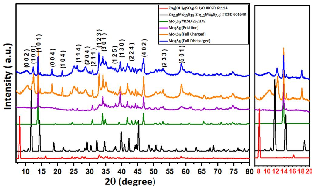
Fig. 2 Post-mortem powder-XRD pattern recorded on the pristine, fully charged to 0.15 V vs.  $\text{Zn}^{2+}/\text{Zn}$ , and fully discharged to 1 V vs.  $\text{Zn}^{2+}/\text{Zn}$   $\text{Mo}_6\text{S}_8$  electrode, along with the standard pattern of  $\text{Mo}_6\text{S}_8$  (ICSD#252376),  $\text{Zn}_4(\text{OH})_6(\text{SO}_4)\cdot 5\text{H}_2\text{O}$  (ICSD#61114), and  $\text{Zn}_{2.9}\text{Mo}_{15}\text{S}_{19}$  (ICSD#601649).
