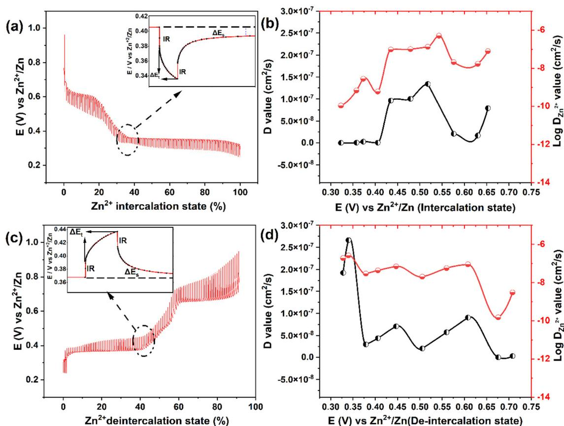
**Fig. 5** Galvanostatic intermittent titration technique (GITT) curves of in 2 M  $\text{ZnSO}_4$  at  $0.1 \text{ A g}^{-1}$  recorded during the  $\text{Zn}^{2+}$  intercalation (a) and deintercalation process (c) as a function of state of (de)intercalation process. The insets in (a) and (c) scheme for a single step of a GITT experiment. The corresponding  $\text{Zn}^{2+}$  diffusion coefficients values among the selected steps during intercalation (b) and deintercalation (d) process.
