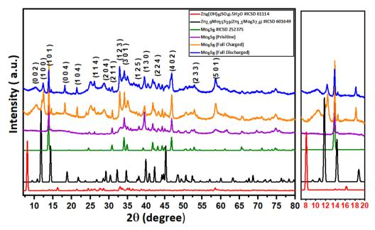
Fig. 2 Post-mortem powder-XRD pattern recorded on the pristine, fully charged to 0.15 V vs.  $Zn^{2+}/Zn$ , and fully discharged to 1 V vs.  $Zn^{2+}/Zn$  Mo<sub>6</sub>S<sub>8</sub> electrode, along with the standard pattern of Mo<sub>6</sub>S<sub>8</sub> (ICSD#252376), Zn<sub>4</sub>(OH)<sub>6</sub>(SO<sub>4</sub>)-5H<sub>2</sub>O (ICSD#61114), and Zn<sub>2.9</sub>Mo<sub>15</sub>S<sub>19</sub> (ICSD#601649).
