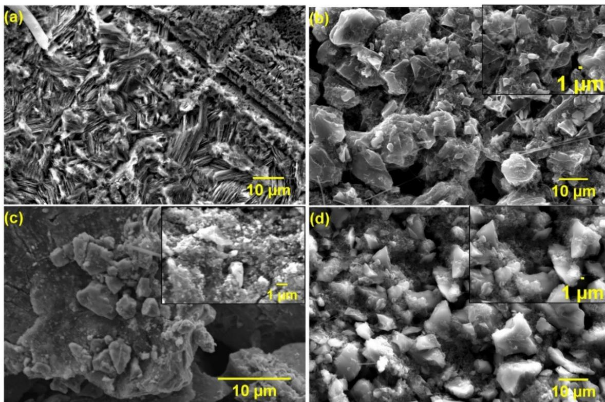
**Fig. 9** Post-mortem SEM characterization of the electrodes examined after cycling in 2 M ZnSO<sub>4</sub> at a gravimetric current of 3 A g<sup>-1</sup>. SEM images of (a) zinc foil, and (b) YEC-8A electrode in Zn/YEC-8A system after 100 cycles. SEM images of (c) Mo<sub>6</sub>S<sub>8</sub> electrode, and (d) YEC-8A electrode in Mo<sub>6</sub>S<sub>8</sub>/YEC-8A coin cell after 8000 cycles.
