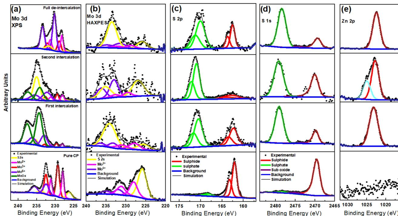
**Fig. 3** High resolution HAXPES and XPS spectra results of the fully/partially charged and fully discharged  $\text{Mo}_6\text{S}_8$  electrode in 2 M  $\text{ZnSO}_4$  half-cell in the region of (a) Mo 3d/S 2s (XPS), (b) Mo 3d/S 2s (HAXPES), (c) S 2p, (d) S 1s (HAXPES), and (e) Zn 2p (HAXPES). Data panels start from bottom to up as follow: pure CP, first intercalation, second intercalation, and full-deintercalation.
