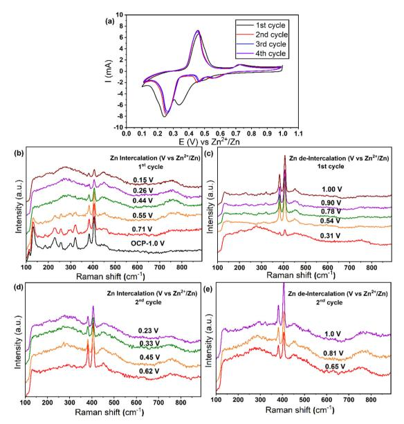
Fig. 4 In situ Raman spectral of  $Mo_6S_8$  electrode at different charge and discharge potential in 2 M ZnSO<sub>4</sub>. (a) Cyclic voltammograms of Zn/ $Mo_6S_8$  cell at 1 mV s<sup>-1</sup> during 1<sup>st</sup>, 2<sup>nd</sup>, 3<sup>rd</sup>, and 4<sup>th</sup> cycle: (b, c), and (d, e) Raman spectra of the first and second cycle during the intercalation/de-intercalation process, respectively.
