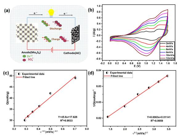
Fig. 7 Schematic and charge storage mechanism of the fabricated energy storage system. (a) Schematic diagram of Mo<sub>6</sub>S<sub>8</sub>/YEC-8A ZIHSC. (b) CVs of Mo<sub>6</sub>S<sub>8</sub>/YEC-8A at different scan rates from 2 to 12 mV s<sup>-1</sup>. Voltammetric charge (Q) calculated as a function of scan rate according to Trasatti's method: (c) Q vs.  $\nu^{-1/2}$  plot and (d) 1/Q vs.  $\nu^{1/2}$  plot.
