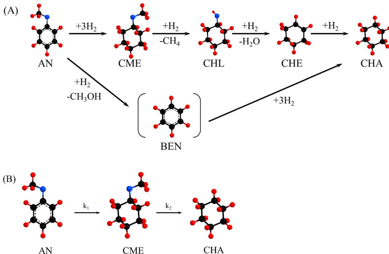
**Scheme 1** (A) Proposed reaction mechanism for the hydrodeoxygenation of anisole with prepared mono- and bimetallic catalysts. (B) Simplified reaction mechanism used for the kinetic study. AN, anisole; BEN, benzene; CME, cyclohexyl methyl ether; CHL, cyclohexanol; CHE, cyclohexene and CHA, cyclohexane.
