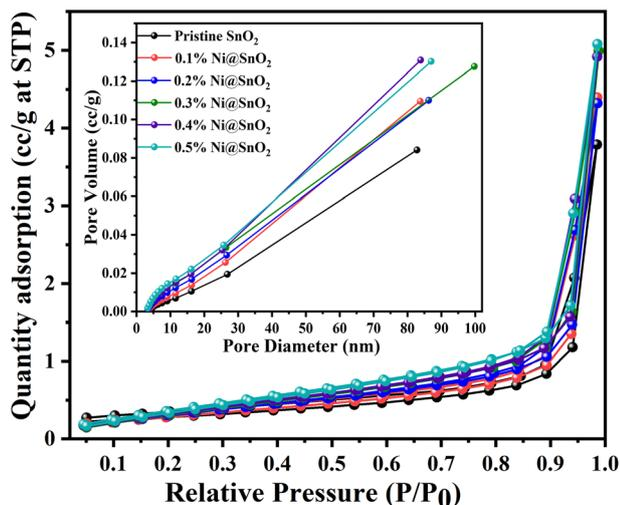
Fig. 11 BET surface area graphs corresponding to the relative pressure for pristine SnO<sub>2</sub> and Ni@SnO<sub>2</sub> nanostructures (inset: pore size distribution curve).
