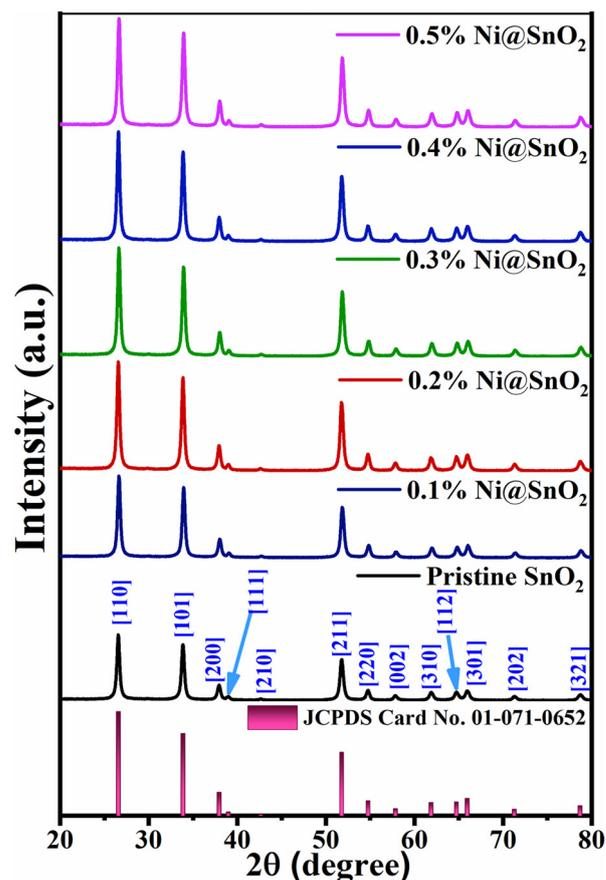
Fig. 2 X-ray diffractograms of the prepared pristine  $\text{SnO}_2$  and  $\text{Ni@SnO}_2$  nanostructure samples.
