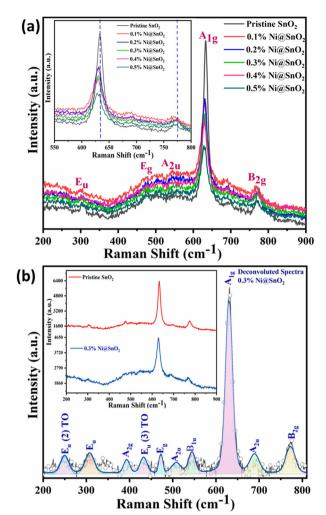
Fig. 4 Raman spectra of the prepared pristine SnO2 and Ni@SnO2 nanostructure in the (a) 200-900 cm<sup>-1</sup> range (inset: 550-800 cm<sup>-1</sup> range) and (b) spectra of  $0.3\%Ni@SnO_2$  nanostructures (inset: 200-900 cm<sup>-1</sup> range for pristine SnO<sub>2</sub> and 0.3%Ni@SnO<sub>2</sub> nanostructure).
