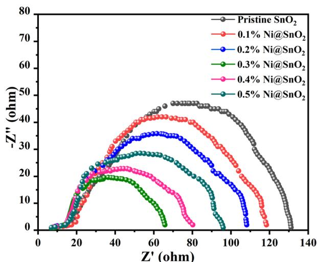
Fig. 12 Nyquist plot for SnO<sub>2</sub> and 0.1 to 0.5% Ni@SnO<sub>2</sub> nanostructures.
