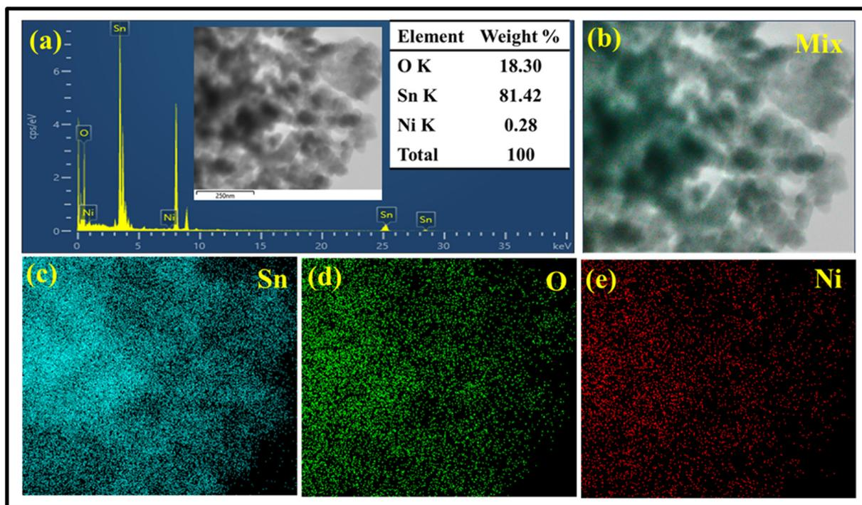
Fig. 10 FETEM-EDS-elemental mapping images of 0.3% Ni@SnO<sub>2</sub> nanostructures. (a) EDS graph and elemental mapping images: (b) mix, (c) Sn, (d) O and (e) Ni.
