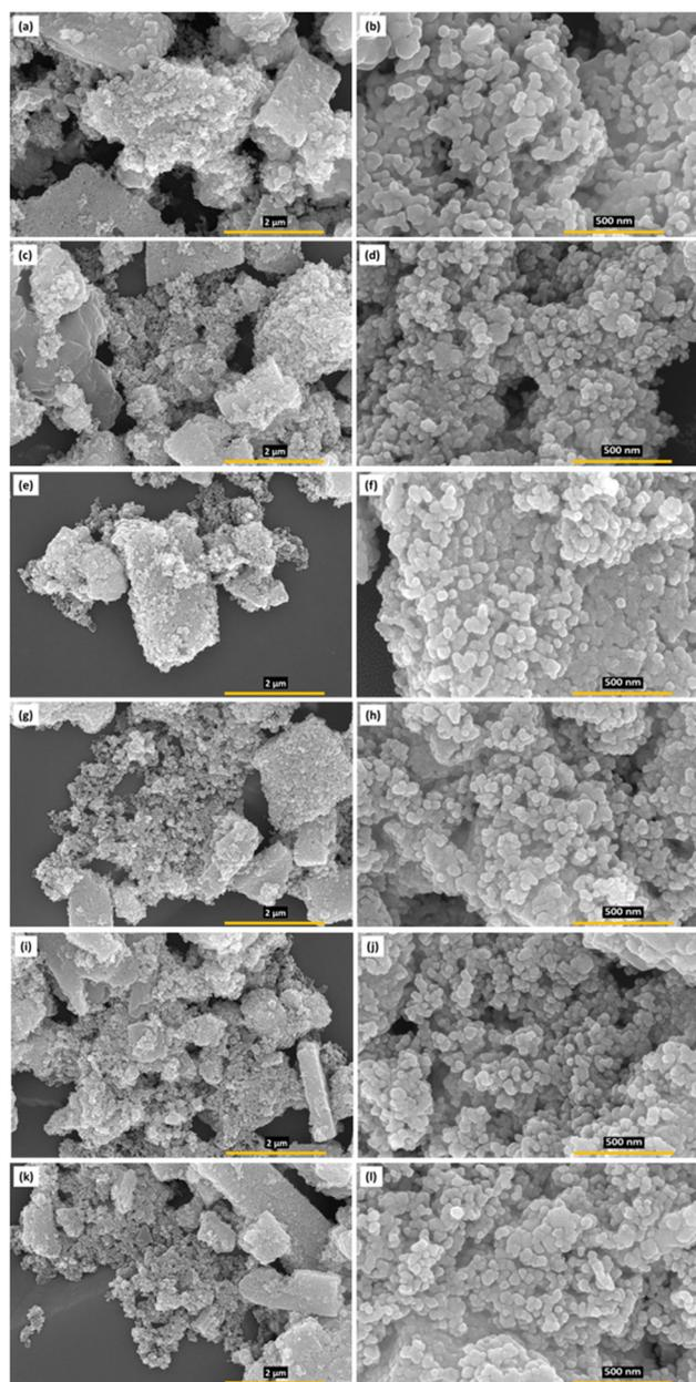
**Fig. 8** FESEM images of pristine SnO<sub>2</sub> (a and b) and 0.1 to 0.5% Ni@SnO<sub>2</sub> nanostructure powders corresponding to Ni loadings of (c and d) 0.1, (e and f) 0.2, (g and h) 0.3, (i and j) 0.4, and (k and l) 0.5% at low and high magnifications, respectively.
