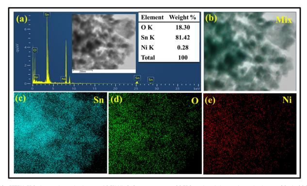
Fig. 10 FETEM-EDS-elemental mapping images of 0.3% Ni@SnO<sub>2</sub> nanostructures. (a) EDS graph and elemental mapping images: (b) mix, (c) Sn, (d) O and (e) Ni.
