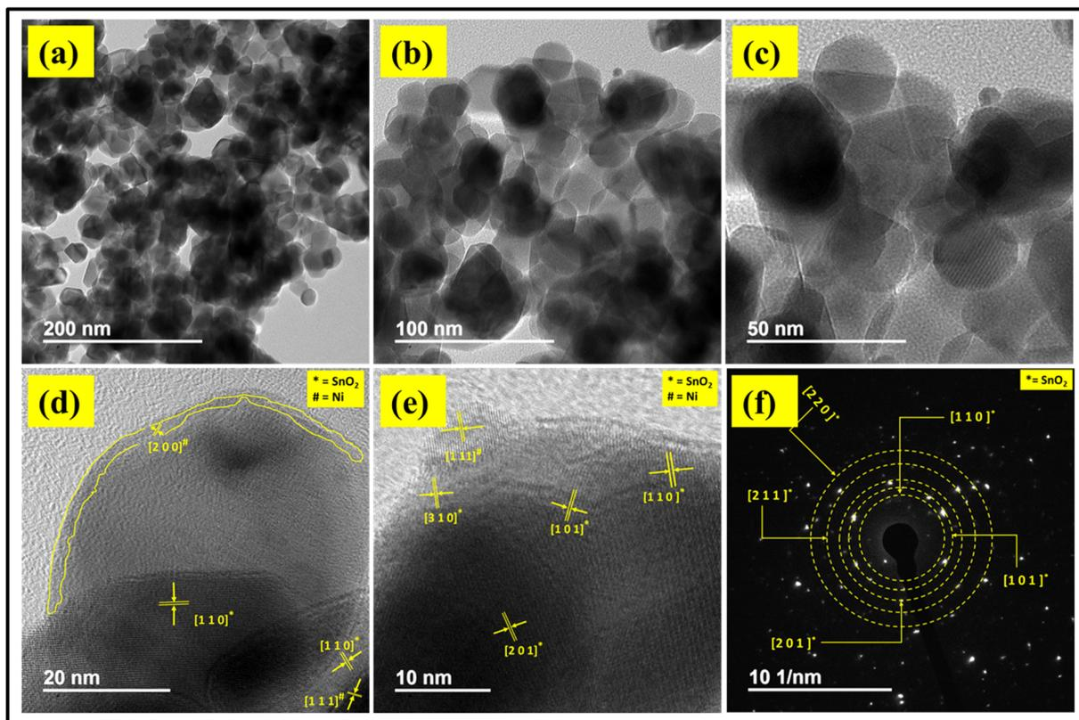
Fig. 9 FETEM images of 0.3% Ni@SnO<sub>2</sub> nanostructures at low magnification (a); their HRTEM images (b), (c), (d) and (e); and the corresponding SAED patterns (f).
