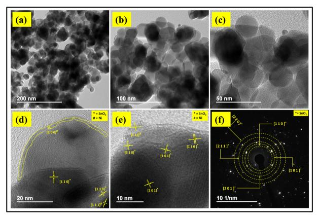
Fig. 9 FETEM images of 0.3% Ni@SnO<sub>2</sub> nanostructures at low magnification (a); their HRTEM images (b), (c), (d) and (e); and the corresponding SAED patterns (f).
