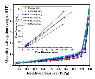
Fig. 11 BET surface area graphs corresponding to the relative pressure for pristine SnO2 and Ni@SnO2 nanostructures (inset: pore size distribution curve).
