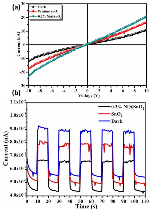
Fig. 13 (a)  $I$ - $V$  characteristics and (b) photo-response of pristine SnO<sub>2</sub> and 0.3% Ni@SnO<sub>2</sub> photodetectors.
