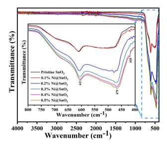
Fig. 7 FTIR spectrum of pristine  ${\rm SnO_2}$  and 0.1 to 0.5% Ni@ ${\rm SnO_2}$  nanostructures.
