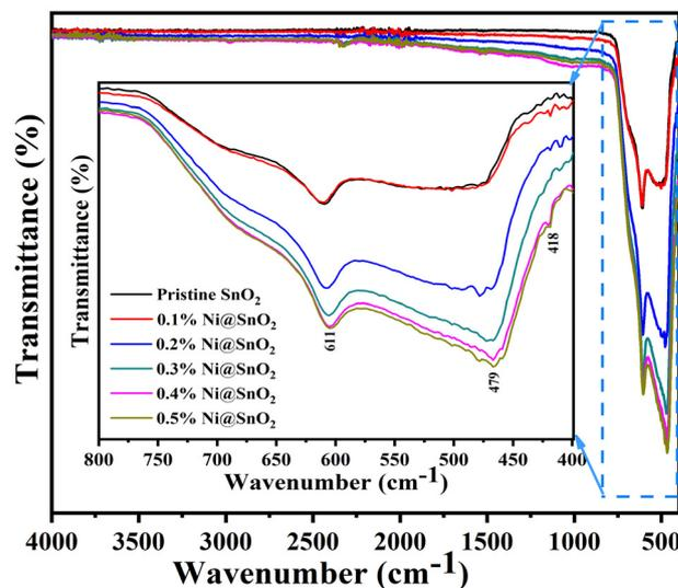
Fig. 7 FTIR spectrum of pristine SnO<sub>2</sub> and 0.1 to 0.5% Ni@SnO<sub>2</sub> nanostructures.
