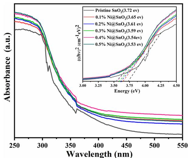
**Fig. 5** UV-DRS spectra (inset: Tauc plot) of pristine-SnO<sub>2</sub> and Ni@SnO<sub>2</sub> nanostructures.
