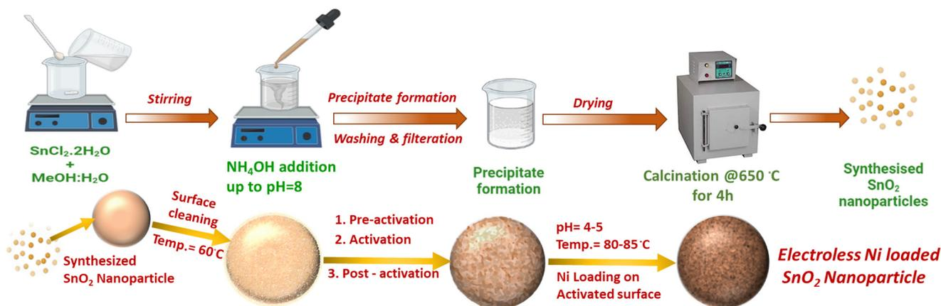
**Fig. 1** Process schematic for the synthesis of SnO<sub>2</sub> nanoparticles and their electroless loading with Ni.
