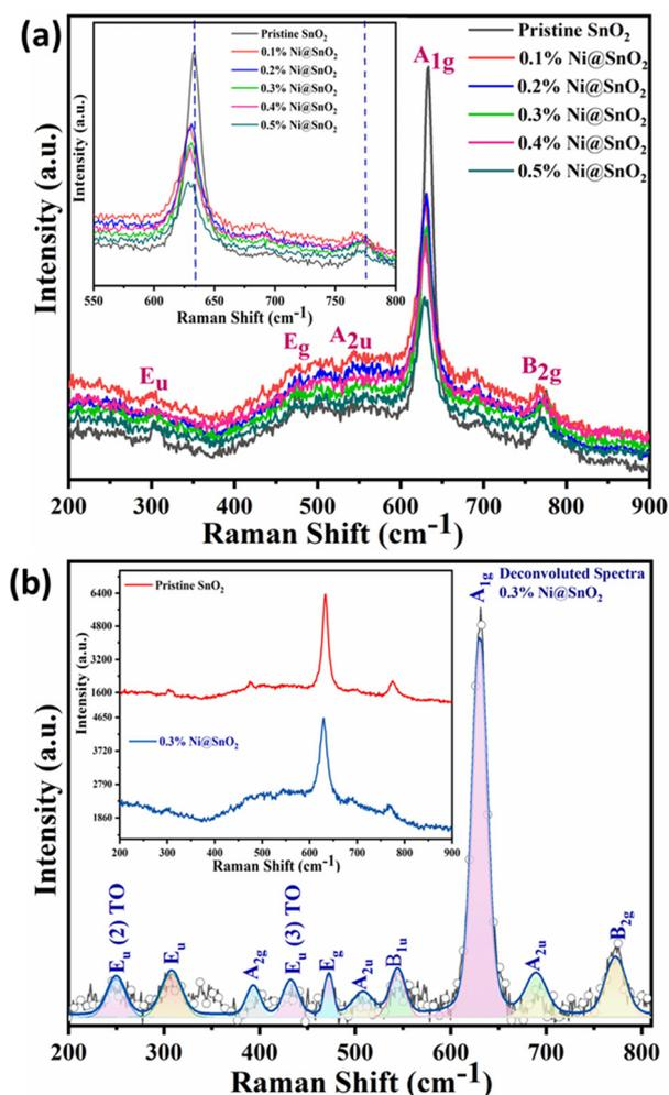
**Fig. 4** Raman spectra of the prepared pristine SnO<sub>2</sub> and Ni@SnO<sub>2</sub> nanostructure in the (a) 200–900 cm<sup>-1</sup> range (inset: 550–800 cm<sup>-1</sup> range) and (b) spectra of 0.3%Ni@SnO<sub>2</sub> nanostructures (inset: 200–900 cm<sup>-1</sup> range for pristine SnO<sub>2</sub> and 0.3%Ni@SnO<sub>2</sub> nanostructure).
