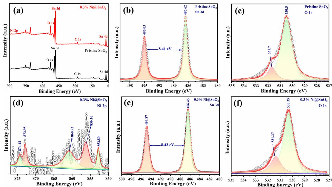
**Fig. 3** XPS spectra of pristine SnO<sub>2</sub> and 0.3% Ni@SnO<sub>2</sub> nanostructure samples. (a) Survey scan for both samples, and deconvoluted high-resolution scans corresponding to the elements (b) Sn 3d and (c) O 1s for Pristine SnO<sub>2</sub> and (d) Ni 2p, (e) Sn 3d and (f) O 1s for the 0.3% Ni@SnO<sub>2</sub> nanostructure.
