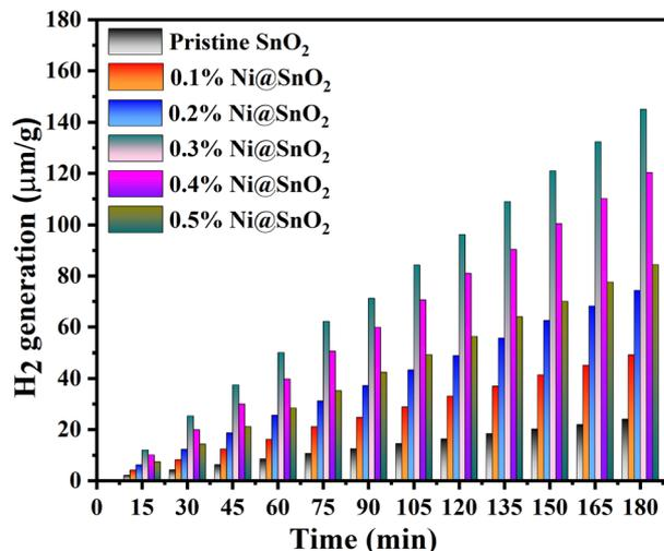
Fig. 15 Photocatalytic hydrogen generation rates of the prepared pristine SnO<sub>2</sub> and Ni@SnO<sub>2</sub> nanostructures.
