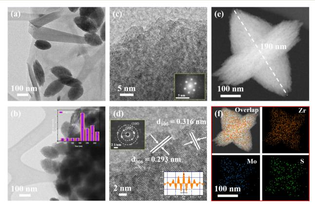
Fig. 2 TEM analysis of the Mo@ZrS<sub>2</sub>/rGO nanocomposite; (a and b) TEM images (inset image; size distribution of seed structures), (c and d) HR-TEM images, (inset image; FFT pattern, SAED, and lattice spacings of 006 and 100 planes), (e) HAADF-STEM image, and (f) TEM-EDS elemental mapping images of Zr, Mo, and S elements, respectively.
