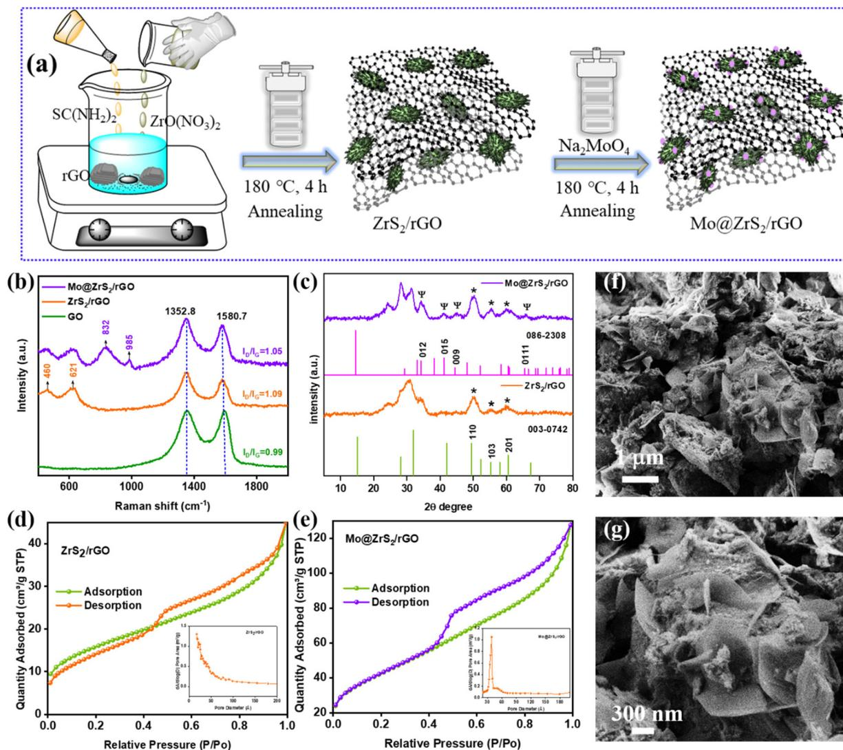
**Fig. 1** (a) Schematic illustration of the synthesis of  $\text{ZrS}_2/\text{rGO}$  and  $\text{Mo@ZrS}_2/\text{rGO}$  nanocomposites. (b) Raman spectra, (c) XRD patterns, (d and e)  $\text{N}_2$  sorption isotherms of  $\text{ZrS}_2/\text{rGO}$  and  $\text{Mo@ZrS}_2/\text{rGO}$  nanocomposites, and (f and g) SEM images of the  $\text{Mo@ZrS}_2/\text{rGO}$  nanocomposite.
