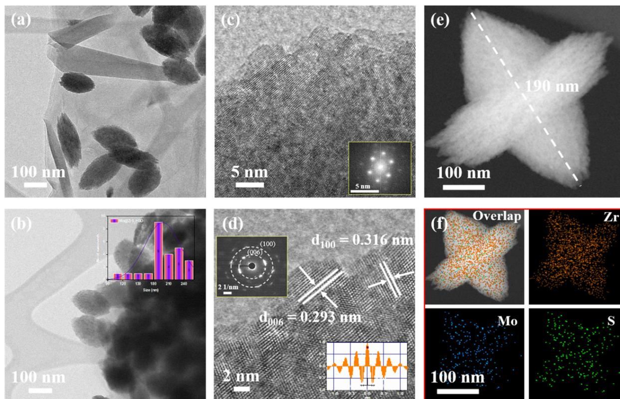
**Fig. 2** TEM analysis of the Mo@ZrS<sub>2</sub>/rGO nanocomposite; (a and b) TEM images (inset image; size distribution of seed structures), (c and d) HR-TEM images, (inset image; FFT pattern, SAED, and lattice spacings of 006 and 100 planes), (e) HAADF-STEM image, and (f) TEM-EDS elemental mapping images of Zr, Mo, and S elements, respectively.
