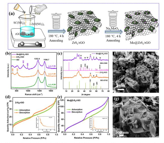
Fig. 1 (a) Schematic illustration of the synthesis of ZrS2/rGO and Mo@ZrS2/rGO nanocomposites. (b) Raman spectra, (c) XRD patterns, (d and e) N2 sorption isotherms of ZrS2/rGO and Mo@ZrS2/rGO nanocomposites, and (f and g) SEM images of the Mo@ZrS2/rGO nanocomposite.
