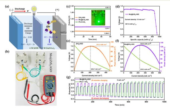
Fig. 5 (a) Schematic illustration of the ZAB setup, (b) image of the battery with an OCV, (c) OCV curve with an inset image of using LED light in ZABs, (d) specific capacity curve of the Mo@ZrS2/rGO air cathode electrode, (e and f) power density curves of ZrS2/rGO and Mo@ZrS2/rGO air cathode electrodes, (g) galvanostatic charge-discharge curve at a current density of 5 mA of commercial Pt-C + IrO2 and Mo@ZrS2/rGO air cathode electrodes, respectively.
