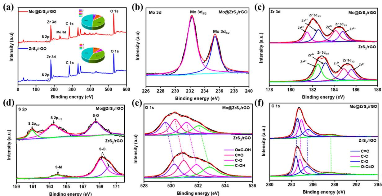
Fig. 3 XPS analysis of  $\text{ZrS}_2/\text{rGO}$  and  $\text{Mo@ZrS}_2/\text{rGO}$  nanocomposites: (a) survey spectra and high-resolution XPS spectra of (b) Mo 3d, (c) Zr 3d, (d) S 2p, (e) O 1s, and (f) C 1s.
