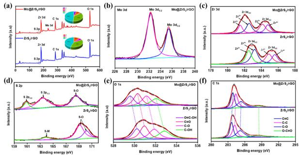
Fig. 3 XPS analysis of ZrS2/rGO and Mo@ZrS2/rGO nanocomposites: (a) survey spectra and high-resolution XPS spectra of (b) Mo 3d, (c) Zr 3d, (d) S 2p, (e) O 1s, and (f) C 1s.
