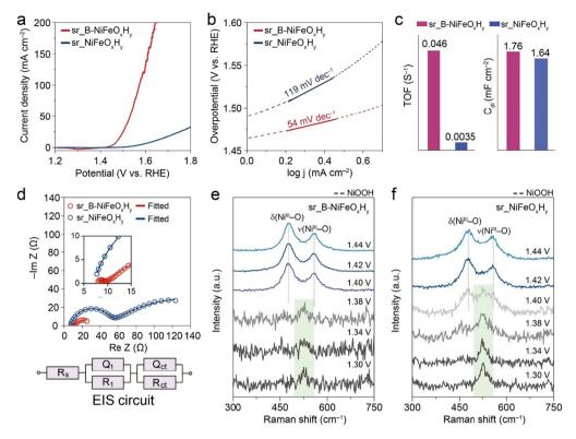
Fig. 2 Electrocatalytic performances: (a) LSV curves, (b) Tafel slopes, (c) turnover frequencies (TOFs), and (d) Nyquist plots of sr\_B-NiFeO<sub>v</sub>H<sub>v</sub> and  $sr_NiFeO_xH_v$ . In situ Raman spectra of (e)  $sr_B-NiFeO_xH_v$  and (f)  $sr_NiFeO_xH_v$  in 1.0 M KOH at the various applied potentials.
