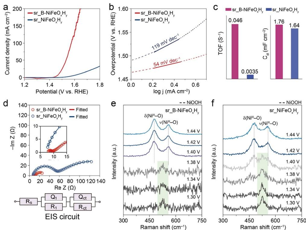
Fig. 2 Electrocatalytic performances: (a) LSV curves, (b) Tafel slopes, (c) turnover frequencies (TOFs), and (d) Nyquist plots of  $\text{sr\_B-NiFeO}_x\text{H}_y$  and  $\text{sr\_NiFeO}_x\text{H}_y$ . *In situ* Raman spectra of (e)  $\text{sr\_B-NiFeO}_x\text{H}_y$  and (f)  $\text{sr\_NiFeO}_x\text{H}_y$  in 1.0 M KOH at the various applied potentials.
