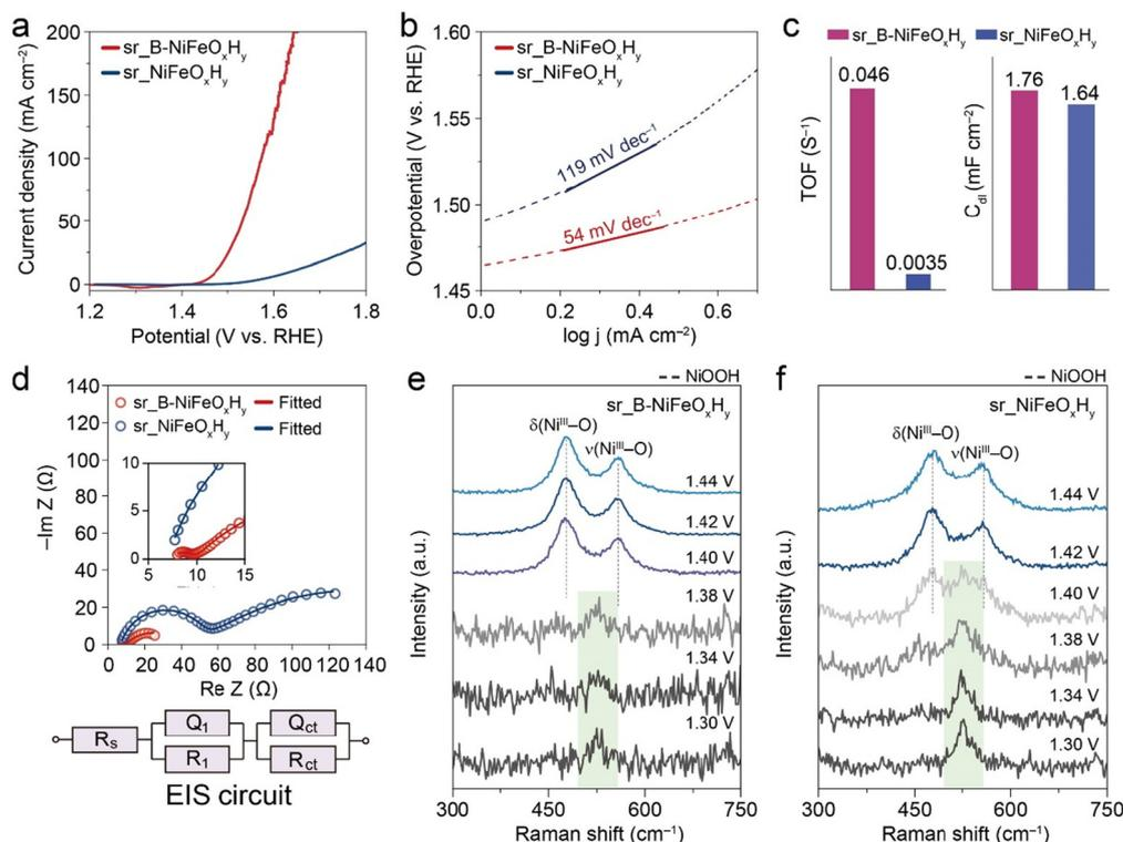
**Fig. 2** Electrocatalytic performances: (a) LSV curves, (b) Tafel slopes, (c) turnover frequencies (TOFs), and (d) Nyquist plots of sr\_B-NiFeO<sub>x</sub>H<sub>y</sub> and sr\_NiFeO<sub>x</sub>H<sub>y</sub>. *In situ* Raman spectra of (e) sr\_B-NiFeO<sub>x</sub>H<sub>y</sub> and (f) sr\_NiFeO<sub>x</sub>H<sub>y</sub> in 1.0 M KOH at the various applied potentials.
