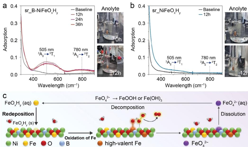
Fig. 3 Detection of Fe<sup>VI</sup>O<sub>4</sub><sup>2-</sup> species using *in situ* UV-vis spectroscopy of the anolyte during OER. (a) sr\_B-NiFeO<sub>x</sub>H<sub>y</sub>, (b) sr\_NiFeO<sub>x</sub>H<sub>y</sub>. (c) The proposed dissolution/redeposition mechanism for the high-valent Fe species in the sr\_B-NiFeO<sub>x</sub>H<sub>y</sub> catalyst.
