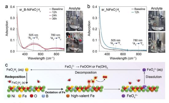
Fig. 3 Detection of  ${\rm Fe^{VI}O_4}^2$  species using in situ UV-vis spectroscopy of the anolyte during OER. (a)  ${\rm sr\_B-NiFeO_xH_{yr}}$  (b)  ${\rm sr\_NiFeO_xH_{yr}}$  (c) The proposed dissolution/redeposition mechanism for the high-valent Fe species in the  ${\rm sr\_B-NiFeO_xH_{yr}}$  catalyst.
