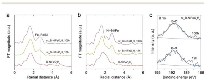
**Fig. 5** The normalized (a) Fe and (b) Ni K-edge EXAFS analyses of pristine B-NiFeO<sub>x</sub>H<sub>y</sub>, after 12 h (sr\_B-NiFeO<sub>x</sub>H<sub>y</sub>, 12 h) and 100 h (B-NiFeO<sub>x</sub>H<sub>y</sub>, 100 h) of long-term stability. (c) The B 1s XPS spectra of sr\_B-NiFeO<sub>x</sub>H<sub>y</sub> after 12 h and 100 h of long-term stability.
