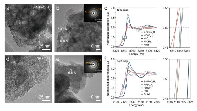
Fig. 1 TEM and HR-TEM images of (a and b) B-NiFeO<sub>x</sub>H<sub>v</sub> and (d and e) NiFeO<sub>x</sub>H<sub>v</sub>, respectively (inset: corresponding SAED patterns of the catalysts). The normalized (c) Ni and (f) Fe K-edge XANES analyses of B-NiFeO<sub>x</sub>H<sub>v</sub> and NiFeO<sub>x</sub>H<sub>v</sub>.
