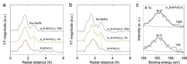
**Fig. 5** The normalized (a) Fe and (b) Ni K-edge EXAFS analyses of pristine B-NiFeO<sub>x</sub>H<sub>y</sub>, after 12 h (sr\_B-NiFeO<sub>x</sub>H<sub>y</sub>, 12 h) and 100 h (B-NiFeO<sub>x</sub>H<sub>y</sub>, 100 h) of long-term stability. (c) The B 1s XPS spectra of sr\_B-NiFeO<sub>x</sub>H<sub>y</sub> after 12 h and 100 h of long-term stability.
