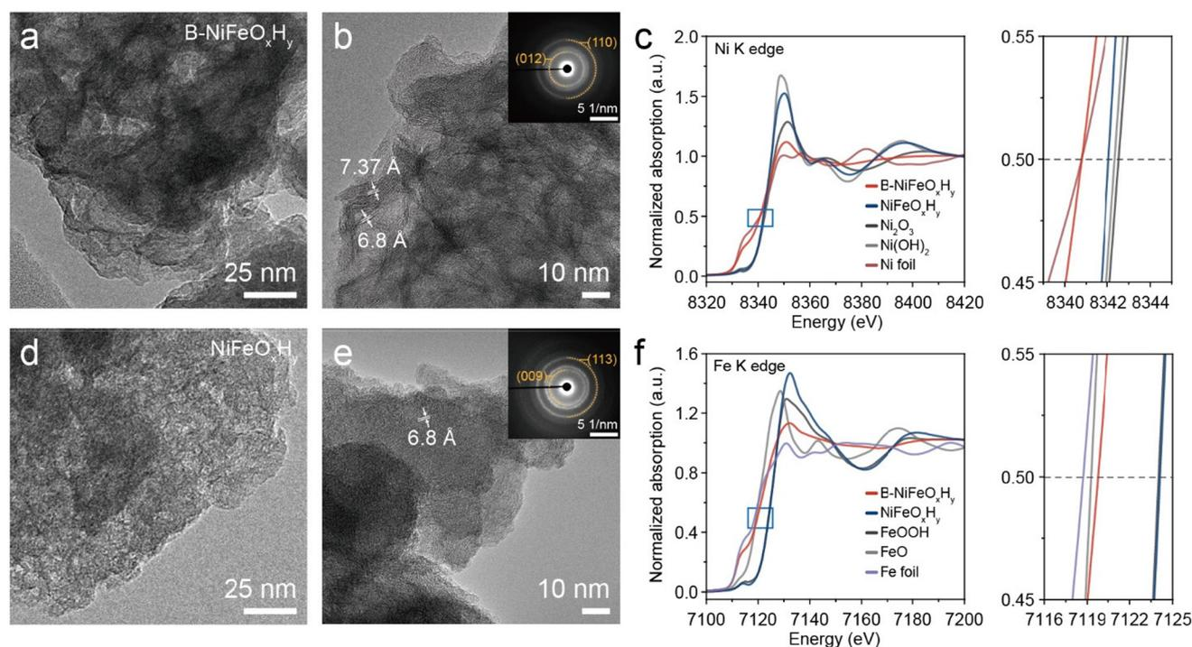
**Fig. 1** TEM and HR-TEM images of (a and b) B- $\text{NiFeO}_x\text{H}_y$  and (d and e)  $\text{NiFeO}_x\text{H}_y$ , respectively (inset: corresponding SAED patterns of the catalysts). The normalized (c) Ni and (f) Fe K-edge XANES analyses of B- $\text{NiFeO}_x\text{H}_y$  and  $\text{NiFeO}_x\text{H}_y$ .
