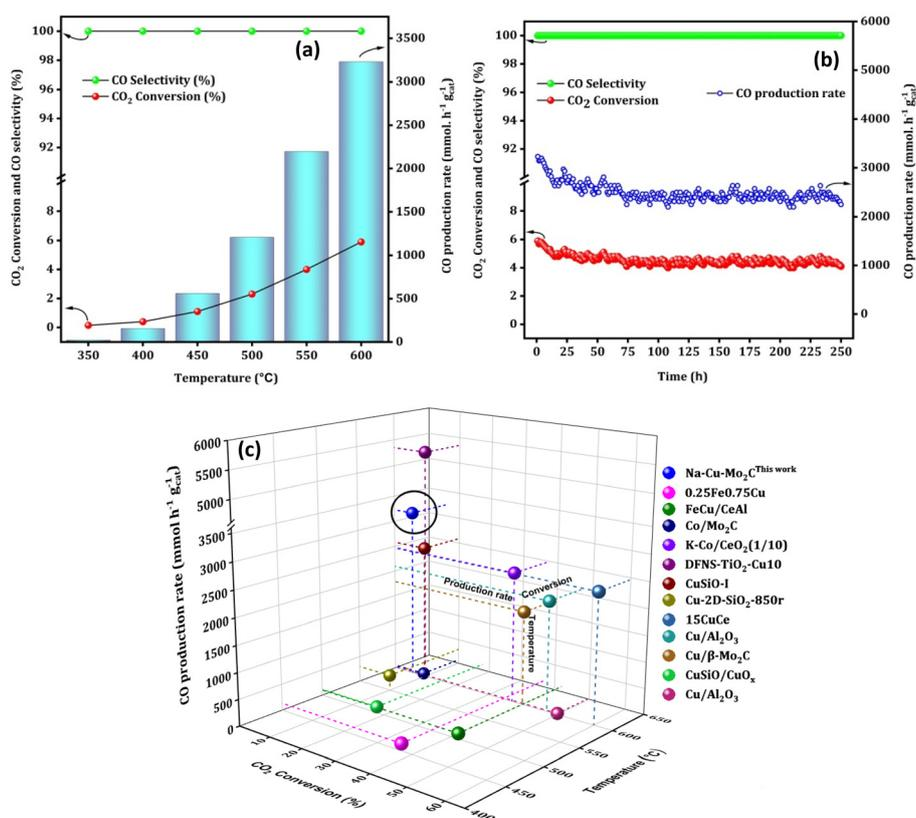
Fig. 9 The high space velocity test (a), stability test at 600 °C (b) over the Na–Cu–Mo<sub>2</sub>C catalyst and comparison with the best reported Fe, Co and Cu based catalysts (c).
