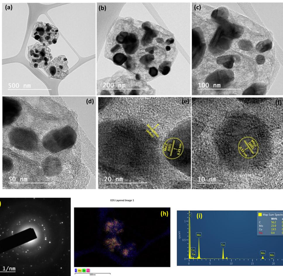
Fig. 12 TEM analysis of the Na–Cu–Mo<sub>2</sub>C catalyst after the 100 h stability test at 800 °C; TEM images (a–f), SAED pattern (g) and EDX/elemental mapping (h and i).
