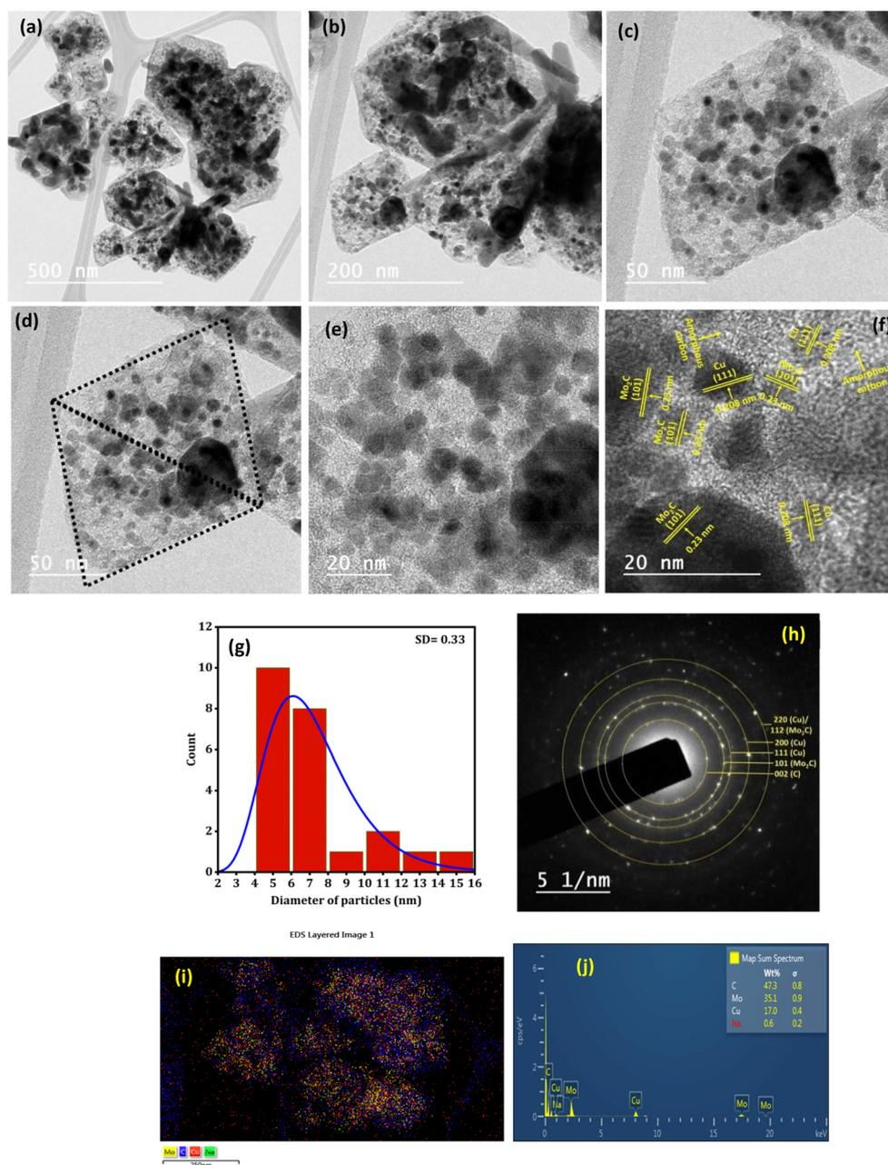
Fig. 5 TEM analysis of the Na-Cu-Mo<sub>2</sub>C catalyst; TEM images (a–f), (g) particle size distribution of image (f), SAED pattern (h) and EDX/elemental mapping (i and j).
