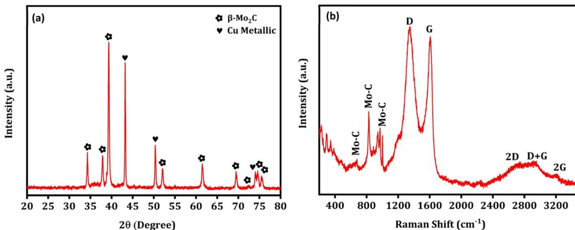
Fig. 11 The XRD pattern (a) and Raman spectra (b) after the stability test for 100 h at 800 °C over the Na–Cu–Mo<sub>2</sub>C catalyst.
