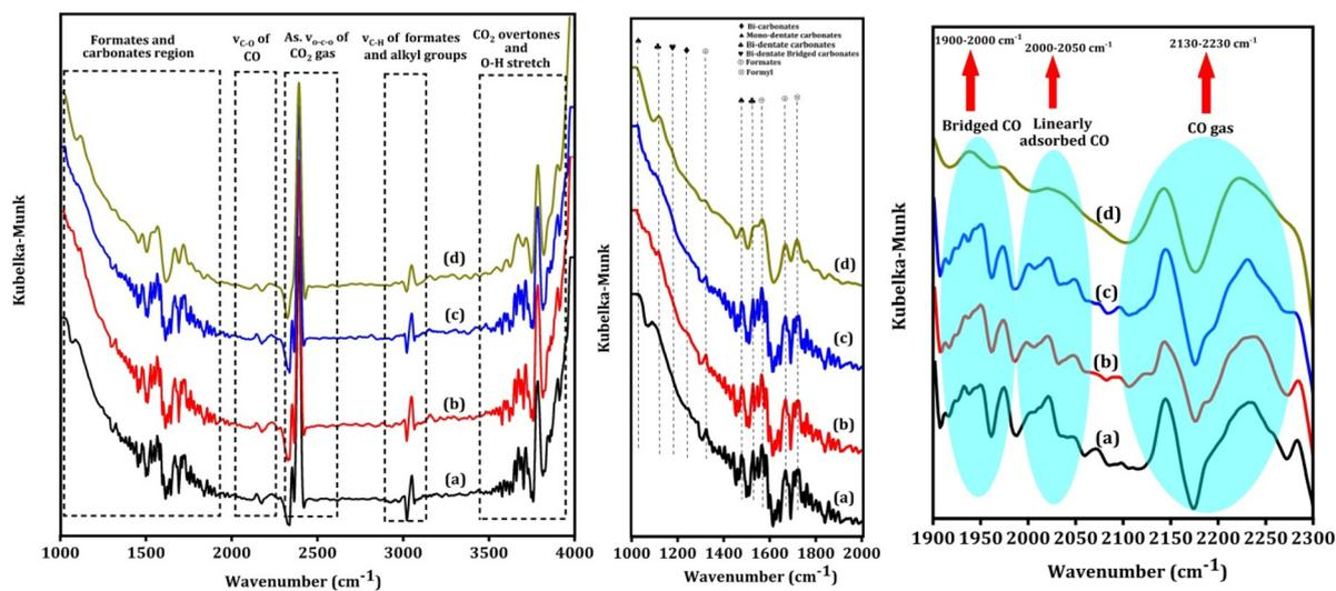
Fig. 7 *In situ* CO<sub>2</sub> DRIFT spectra over the Na-Cu-Mo<sub>2</sub>C catalyst, at 550 °C after 5 ml min<sup>-1</sup> CO<sub>2</sub> + 20 ml min<sup>-1</sup> H<sub>2</sub> flow for 60 min (a) 120 min (b), 180 min (c) and 240 min (d).
