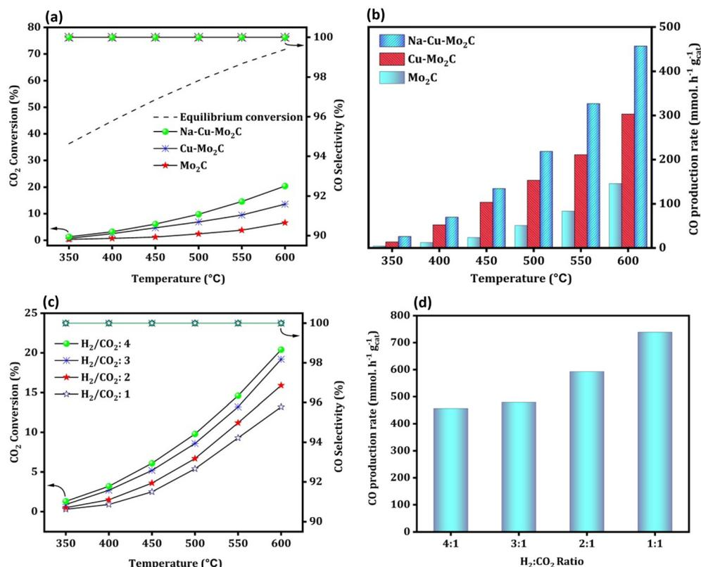
**Fig. 8** RWGS activity of the derived catalysts; CO<sub>2</sub> conversion, CO selectivity, and CO production rate (a and b); the effect of different H<sub>2</sub>:CO<sub>2</sub> ratios over the Na-Cu-Mo<sub>2</sub>C catalyst on CO<sub>2</sub> conversion and CO production rate (c and d).
