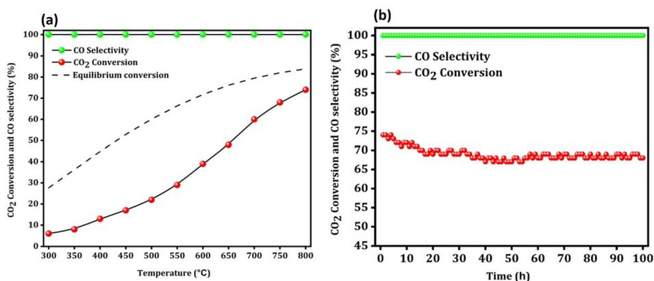
Fig. 10 The low space velocity test with a wide temperature range (a) and the stability test at 800 °C (b) over the Na–Cu–Mo<sub>2</sub>C catalyst.
