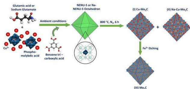
**Scheme 1** Synthesis scheme for the nano-structured porous Na-Cu-Mo<sub>2</sub>C catalyst.
