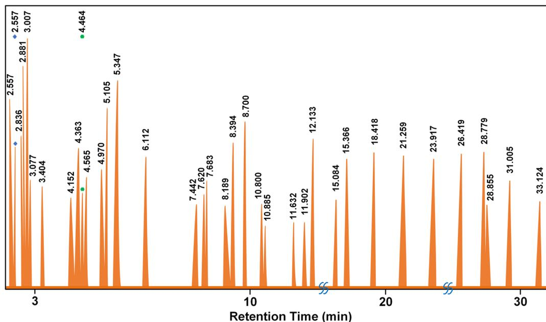
Fig. 10 Graphical analysis of pyrolysis oil with GC-MS.
