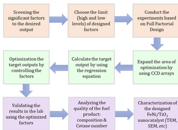
Fig. 1 The general step to design the Fe–Ni/TiO<sub>2</sub> nanocatalyst in this work.
