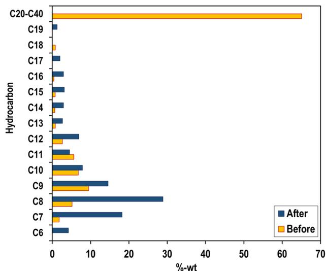
**Fig. 11** Hydrocarbon composition before and after pyrolysis.
