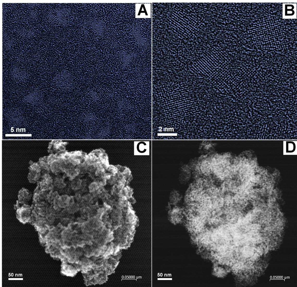
**Fig. 12** HRTEM images of the Fe–Ni NPs with different magnifications (A) and (B); STEM images of FeNi/TiO<sub>2</sub> using Secondary Electron Imaging (SEI) for observing the morphology (C), and High-Angle Annular Dark Field (HAADF) (D). The nanocatalysts were analyzed using HRTEM (“TITAN 80-300 Berlin Holography Special”).
