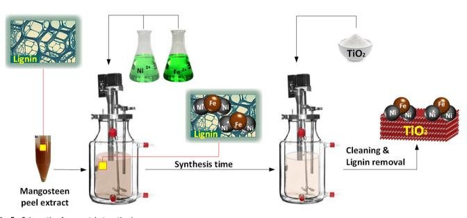
Fig. 3 Schematic of nanocatalyst synthesis.
