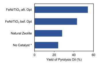
Fig. 16 Comparison of oil yields in the pyrolysis of waste lubricating oil using the optimized Fe-Ni/TiO<sub>2</sub>, natural zeolite, and the catalyst-free process (\* the catalyst-free process was carried out at 650 °C).
