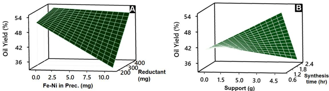
Fig. 8 Surface plots of the oil yields that resulted from the interaction between the metal amount and the reductant amount (A) and from the interaction between the support amount and the synthesis time (B).
