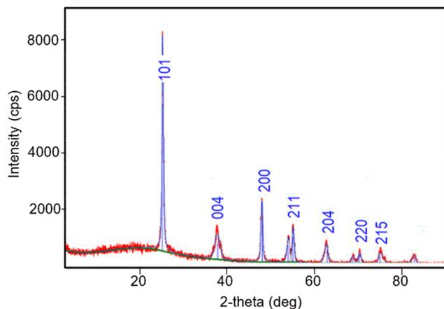
Fig. 15 XRD analysis of Fe-Ni/TiO<sub>2</sub>.
