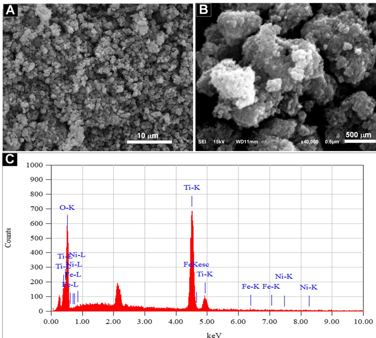
Fig. 14 SEM images of the Fe–Ni/TiO<sub>2</sub> nanocatalyst at magnifications of 3000× (A) and 40 000× (B). The corresponding EDS analysis (C) confirms the presence of Fe–Ni nanoparticles in the catalyst.
