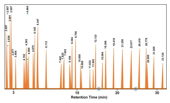
Fig. 10 Graphical analysis of pyrolysis oil with GC-MS.
