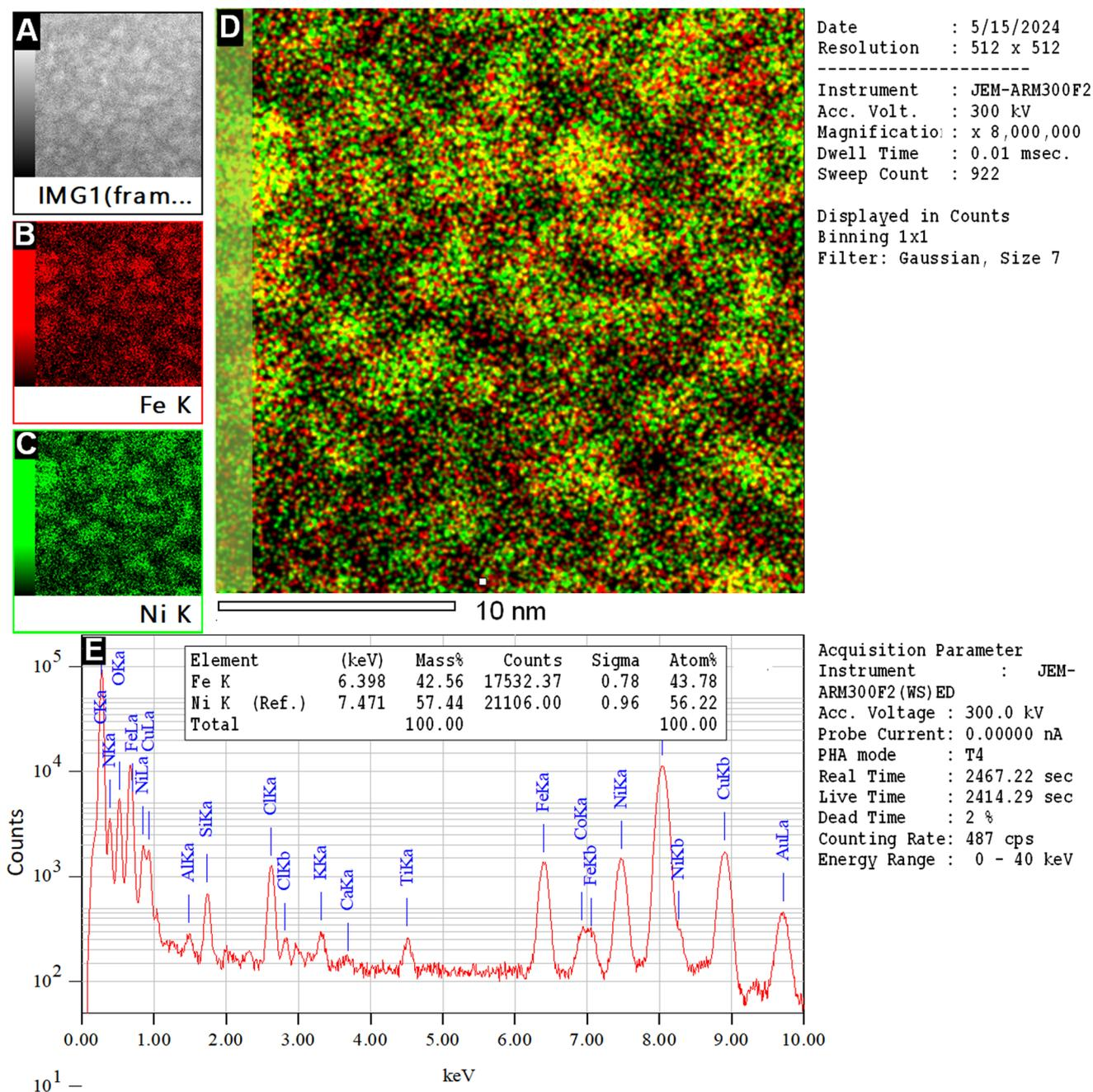
**Fig. 13** EDX mapping of the Fe–Ni NPs. (A) Initial HAADF image; (B) mapping of Fe; (C) mapping of Ni; (D) overlay of Fe and Ni revealing homogeneously distributed Fe–Ni nanoparticles; (E) EDS analysis of the entire area and quantification. The composition was analyzed using HRSTEM analysis on a probe-corrected JEM-RM300F2 at ZELMI of TU-Berlin.
