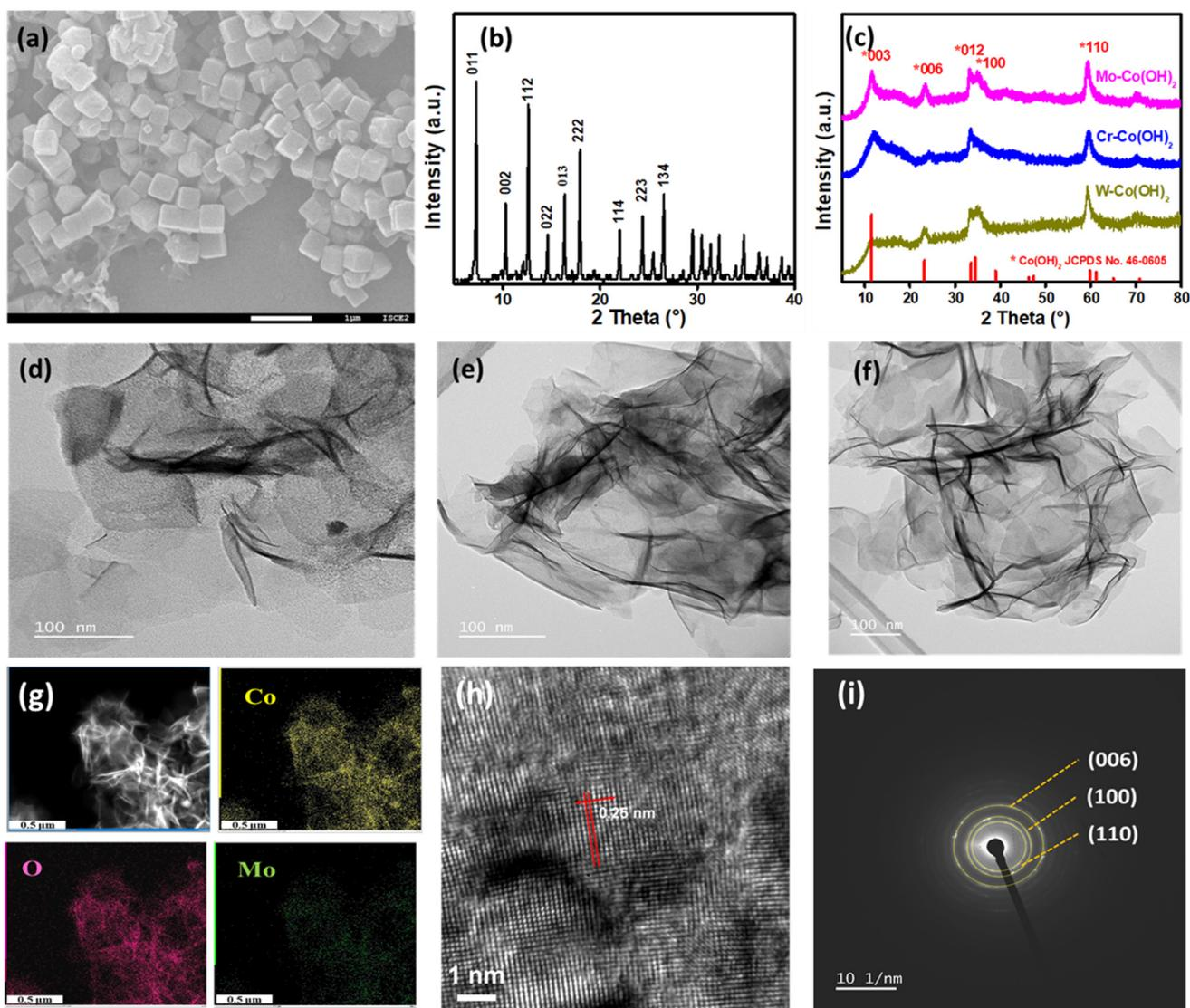
**Fig. 1** (a) SEM image and (b) XRD pattern of the ZIF-67 template. (c) XRD patterns of Mo-Co(OH)<sub>2</sub>, Cr-Co(OH)<sub>2</sub> and W-Co(OH)<sub>2</sub>. (d–f) TEM images of Mo-Co(OH)<sub>2</sub>, Cr-Co(OH)<sub>2</sub> and W-Co(OH)<sub>2</sub> 2D nanosheets. (g) TEM mapping images of Mo-Co(OH)<sub>2</sub>. (h) High-resolution TEM (HRTEM) image of Mo-Co(OH)<sub>2</sub> and (i) selected-area electron diffraction pattern of Mo-Co(OH)<sub>2</sub>.
