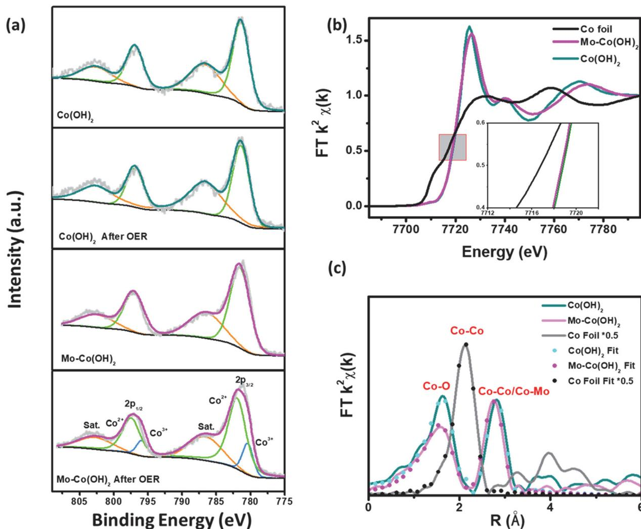
Fig. 3 (a) Co 2p XPS absorption spectra of Mo-Co(OH)<sub>2</sub> and Co(OH)<sub>2</sub>. (b) Co K-edge XAFS absorption spectra of Mo-Co(OH)<sub>2</sub>, Co(OH)<sub>2</sub> and Co foil and (c) k<sub>2</sub>-weighted Fourier transform spectra of the Co K-edge EXAFS absorption spectra.
