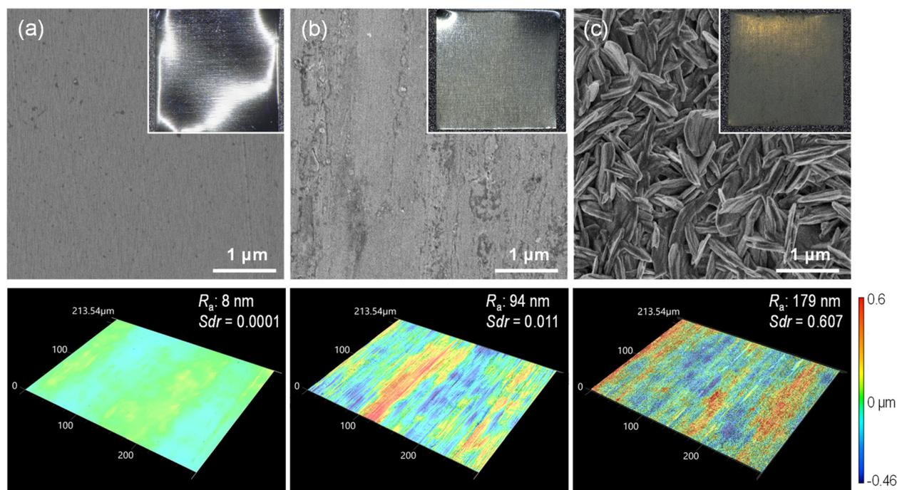
Fig. 2 SEM and 3D laser scanning confocal microscope images of the surfaces of (a) Pt/p-SUS, (b) Pt/SUS, and (c) Pt/Al<sub>2</sub>O<sub>3</sub>/SUS. Insets in the upper images depict the overall foil samples sized 30  $\times$  30 mm<sup>2</sup>.  $R_a$  and Sdr values (insets of the bottom images) denote surface roughness and surface area ratio, respectively. Pt was deposited onto SUS foils using 2000-shot AP pulses.
