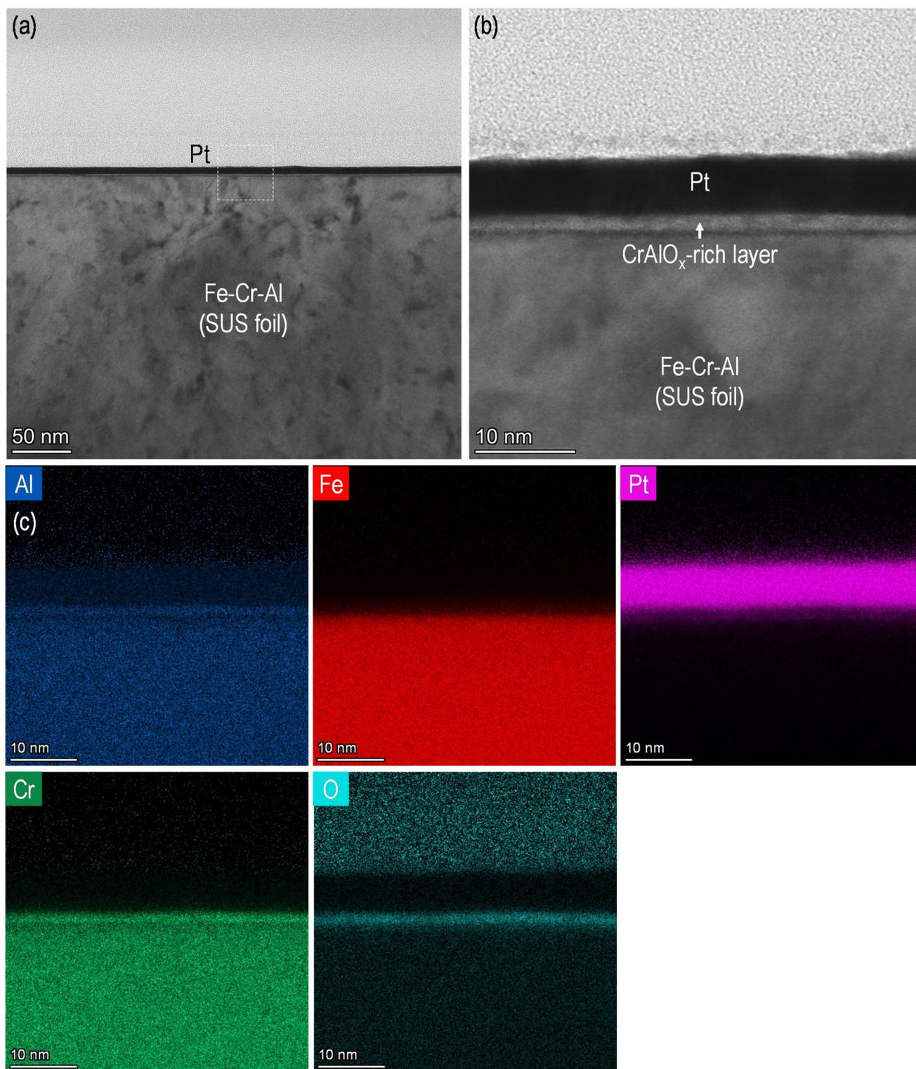
**Fig. 3** (a) STEM image of the cross-sectional Pt overlayer structure formed on the p-SUS foil. (b) An enlarged image was obtained from a dashed square region of (a). (c) X-ray images obtained from a square region of (a). Pt was deposited onto the SUS foil using 8000-shot AP pulses to enhance visibility.
