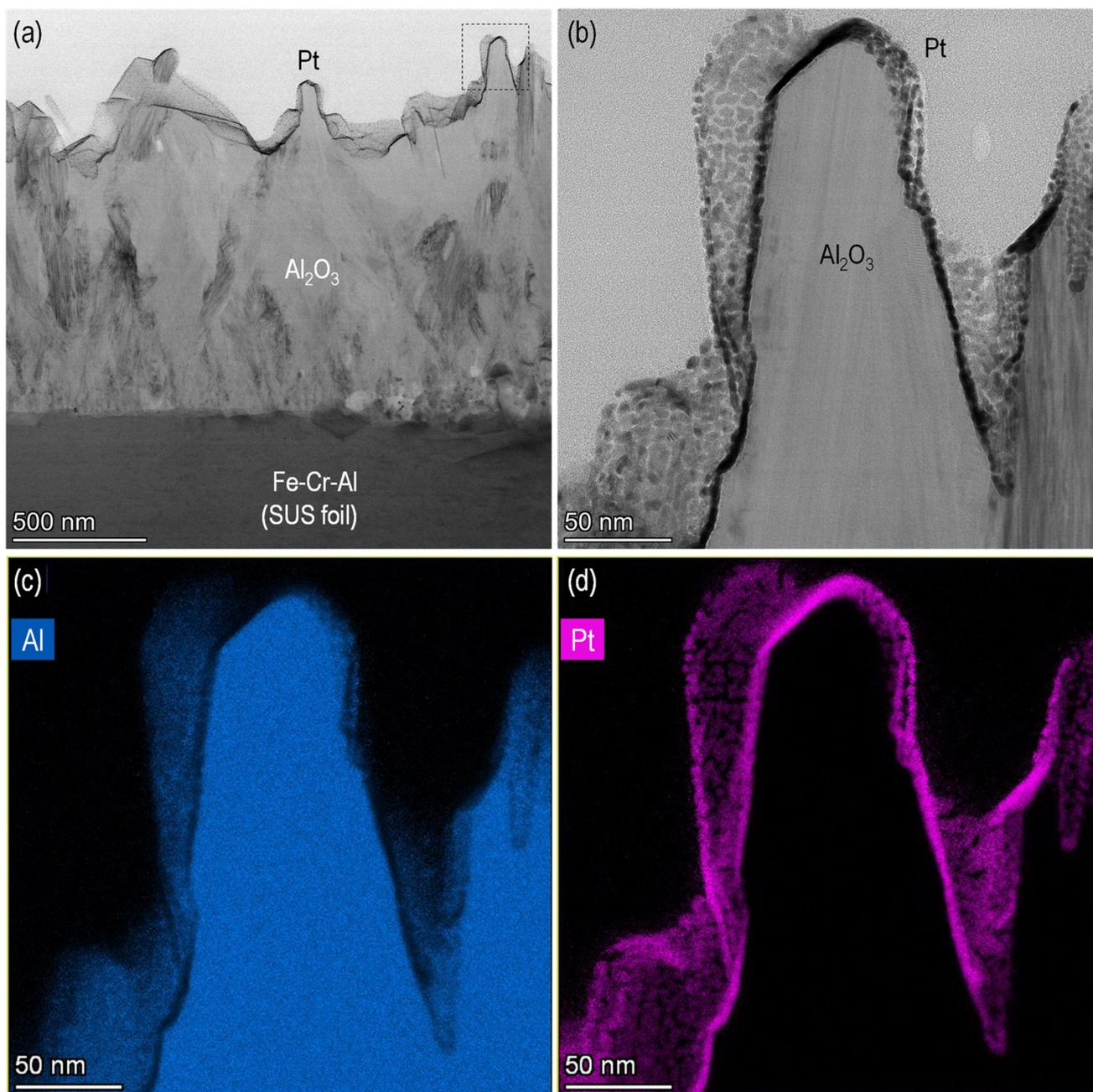
**Fig. 4** (a) STEM image of the cross-sectional Pt overlayer structure formed on the  $\text{Al}_2\text{O}_3$ /SUS foil. (b) An enlarged image was obtained from a dashed square region of (a). (c) Al and (d) Pt X-ray images obtained from a square region of (a). Pt was deposited onto the  $\text{Al}_2\text{O}_3$ /SUS foil using 8000-shot AP pulses to enhance visibility.
