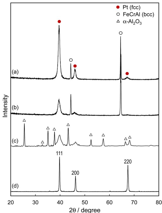
**Fig. 1** XRD patterns of film catalysts on SUS (Fe–Cr–Al) foil. (a) Pt/p-SUS, (b) Pt/SUS, (c) Pt/Al<sub>2</sub>O<sub>3</sub>/SUS and (d) polycrystalline Pt plate. To enhance reflection intensity, Pt was coated onto SUS foils using 8000-shot AP pulses.
