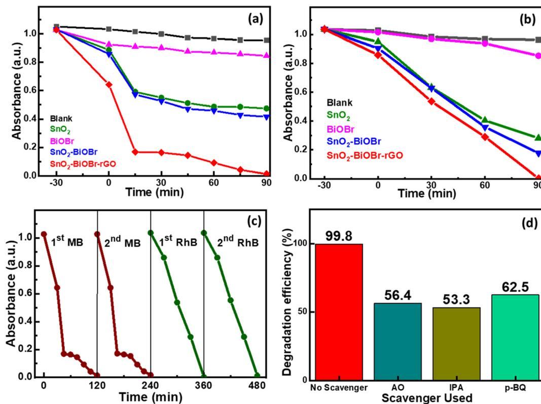
Fig. 8 Kinetics for (a) MB dye and (b) RhB dye degradation using  $\text{SnO}_2$ , BiOBr,  $\text{SnO}_2\text{-BiOBr}$ , and  $\text{SnO}_2\text{-BiOBr-rGO}$  as photocatalysts. (c) Repeatability test for two cycles for MB and RhB dyes and (d) the effect of adding *p*-BQ, IPA, and AO as scavengers in RhB dye.
