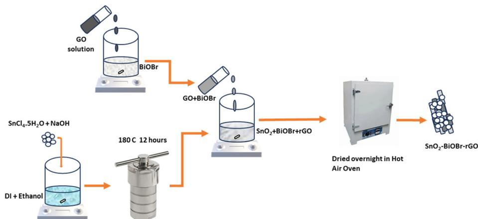
**Scheme 1** Schematic showing the proposed synthesis route of the ternary nanocomposite.
