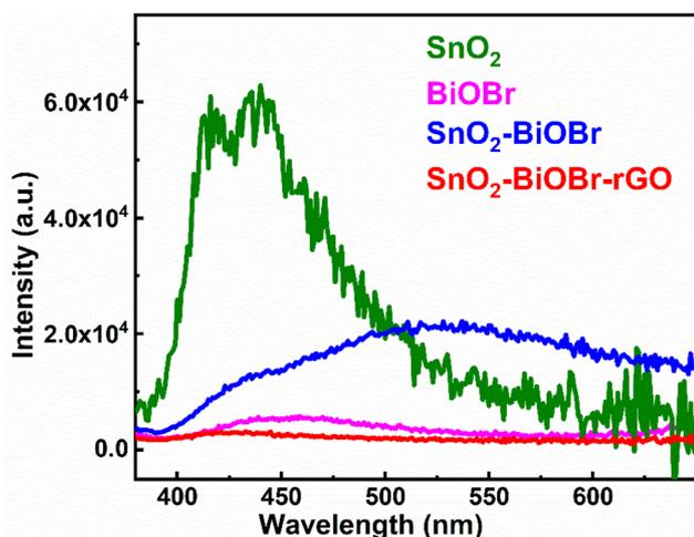
Fig. 6 Photoluminescence spectra of SnO<sub>2</sub>, BiOBr, SnO<sub>2</sub>-BiOBr, and SnO<sub>2</sub>-BiOBr-rGO.
