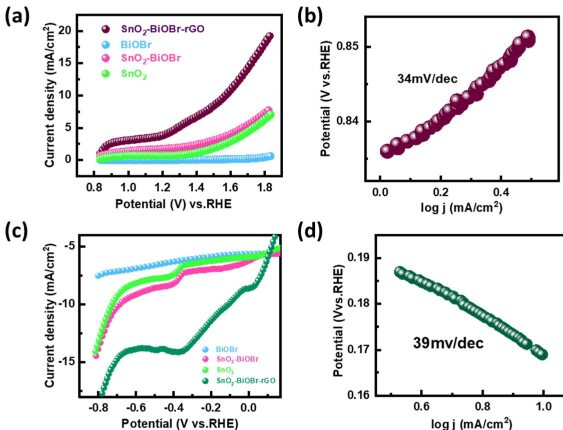
Fig. 12 (a) Linear sweep voltammetry (LSV) scan for OER performance of BiOBr, SnO<sub>2</sub>, SnO<sub>2</sub>-BiOBr, and SnO<sub>2</sub>-BiOBr-rGO under light irradiation (b) OER Tafel plot for SnO<sub>2</sub>-BiOBr-rGO (c) LSV scan for HER performance of BiOBr, SnO<sub>2</sub>, SnO<sub>2</sub>-BiOBr and SnO<sub>2</sub>-BiOBr-rGO under light irradiation (d) HER Tafel plot for the SnO<sub>2</sub>-BiOBr-rGO ternary nanocomposite.
