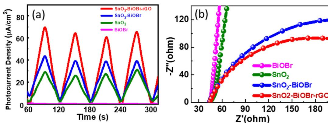
Fig. 13 (a) Photocurrent response of the SnO<sub>2</sub>, BiOBr, SnO<sub>2</sub>-BiOBr, SnO<sub>2</sub>-BiOBr-rGO and (b) EIS Nyquist plots under light irradiation for SnO<sub>2</sub>, BiOBr, SnO<sub>2</sub>-BiOBr, SnO<sub>2</sub>-BiOBr-rGO.
