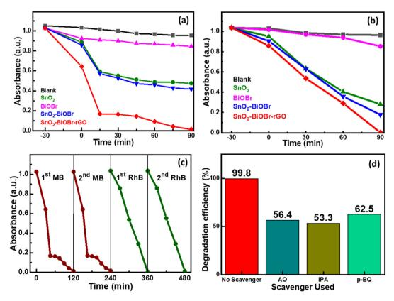
Fig. 8 Kinetics for (a) MB dye and (b) RhB dye degradation using  $SnO_2$ , BiOBr,  $SnO_2$ -BiOBr, and  $SnO_2$ -BiOBr-rGO as photocatalysts. (c) Repeatability test for two cycles for MB and RhB dyes and (d) the effect of adding p-BQ, IPA, and AO as scavengers in RhB dye.
