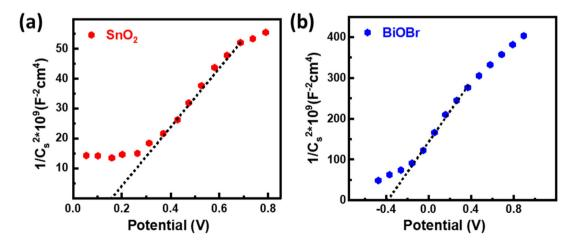
Mott-Schottky plots for (a) SnO<sub>2</sub> and (b) BiOBr.
