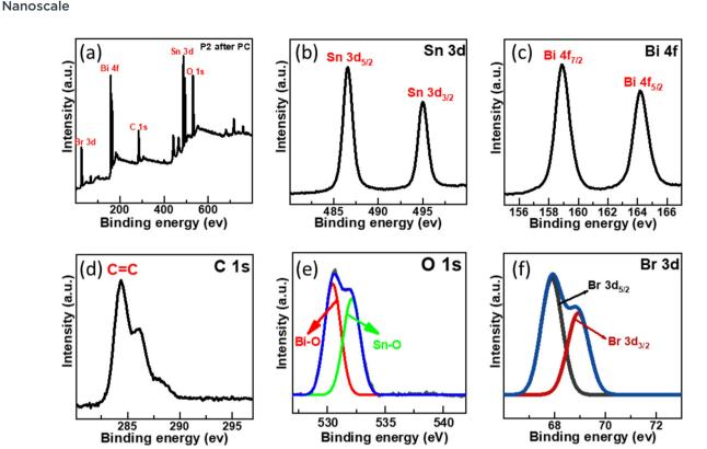
Fig. 11 (a) After photocatalytic treatment the survey scan of  $SnO_2$ -BiOBr-rGO and high-resolution XPS spectrum of (b) Sn 3d, (c) Bi 4f, (d) C 1s, (e) O 1s, (f) Br 3d.
