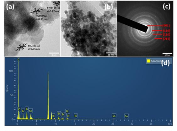
Fig. 4 (a) HRTEM image, and (b) TEM image (c) selected area electron diffraction (SAED) and (d) EDS spectrum of SnO<sub>2</sub>-BiOBr-rGO.
