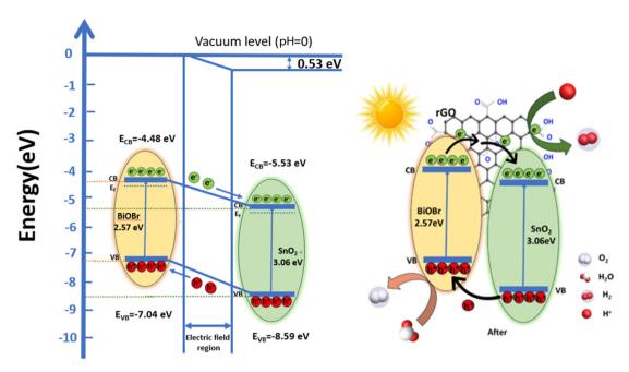
Fig. 10 Schematic illustration of energy level band bending diagram for BiOBr and SnO2 and a possible mechanism for organic dye degradation under visible light by the ternary nanocomposite (SnO<sub>2</sub>-BiOBr-rGO).
