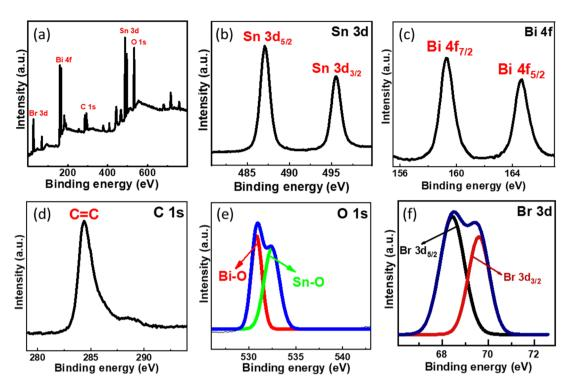
Fig. 7 (a) Survey XPS spectra of SnO<sub>2</sub>-BiOBr-rGO and high-resolution XPS spectrum of (b) Sn 3d, (c) Bi 4f, (d) C 1s, (e) O 1s, (f) Br 3d.
