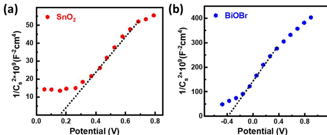
Fig. 9 Mott-Schottky plots for (a)  $\text{SnO}_2$  and (b)  $\text{BiOBr}$ .
