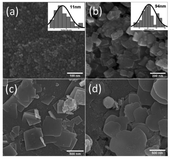
Fig. 3 FESEM images of (a) SnO<sub>2</sub>, (b) BiOBr (c) SnO<sub>2</sub>-BiOBr, (d) SnO<sub>2</sub>-BiOBr-rGO
