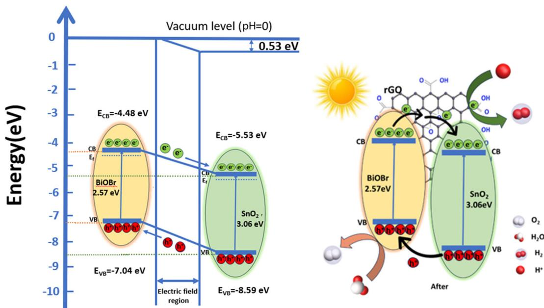
**Fig. 10** Schematic illustration of energy level band bending diagram for BiOBr and SnO<sub>2</sub> and a possible mechanism for organic dye degradation under visible light by the ternary nanocomposite (SnO<sub>2</sub>-BiOBr-rGO).
