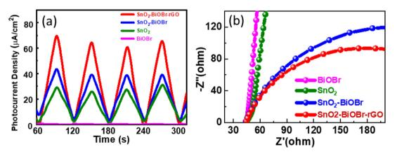
Fig. 13 (a) Photocurrent response of the  $SnO_2$ , BiOBr,  $SnO_2$ -BiOBr,  $SnO_2$ -BiOBr-rGO and (b) EIS Nyquist plots under light irradiation for  $SnO_2$ , BiOBr,  $SnO_2$ -BiOBr,  $SnO_2$ -BiOBr-rGO.
