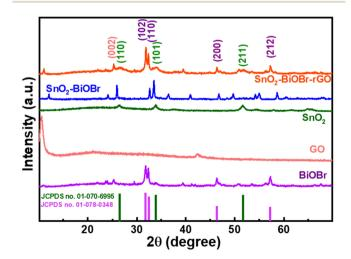
**Fig. 1** Powder X-ray diffraction pattern of BiOBr, GO, SnO<sub>2</sub>- SnO<sub>2</sub>- BiOBr, and SnO<sub>2</sub>-BiOBr-rGO.
