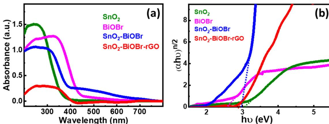
Fig. 5 (a) UV-visible-diffuse reflectance spectra for SnO<sub>2</sub>, BiOBr, SnO<sub>2</sub>-BiOBr, and SnO<sub>2</sub>-BiOBr-rGO. (b) Tauc plot of  $(\alpha h\nu)^{n/2}$  vs.  $h\nu$  (eV) for SnO<sub>2</sub>, BiOBr, SnO<sub>2</sub>-BiOBr, and SnO<sub>2</sub>-BiOBr-rGO.
